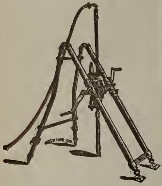
"M" Drill—Hand Power. Capacity—300 ft. depth. Removes 1 7/8 inches solid core.
