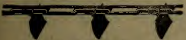
SECTION OF CONVEYOR.
