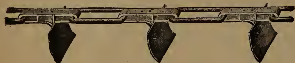
SECTION OF CONVEYOR.
