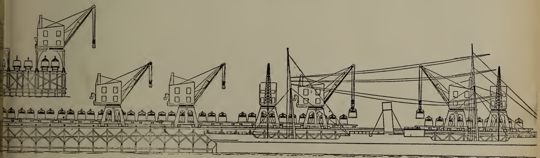
Dominion Coal Co. Ltd., International Pier. —The above illustrations show the improved coal-handling appliances now under construction by the Ludlow Manufacturing Co., Cleveland, Ohio. The pier is of following dimensions: Length, 605 feet; width, 92 feet; height, 27 feet. The derricks—12 in number—are of new design, 6 on each side of pier, and are built entirely of steel and iron, including the house, which makes them strictly fire proof. The main engine which does the hoisting and rotating are double 12x14 cylinders. For propelling a separate pair of engines, 6x8 cylinders are used. The lifting capacity of these machines is 15 tons. The buckets used are of the latest patent bottom dump, 100 inches in diameter and 64 inches high, and are tripped or discharged by the engineer at such depth in the vessel as he may desire. The buckets are placed upon flat cars and taken to the mines where they are loaded from the tippie. The cars are moved upon the dock by gravity. This is the largest and most complete bucket plant in the world.
