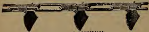
SECTION OF CONVEYOR.
