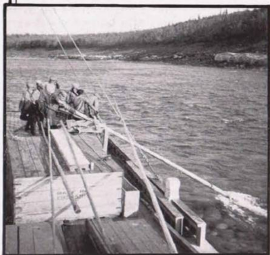
Using spar to lever the ves- sel out of shallow water into channel on Great Bear River.
