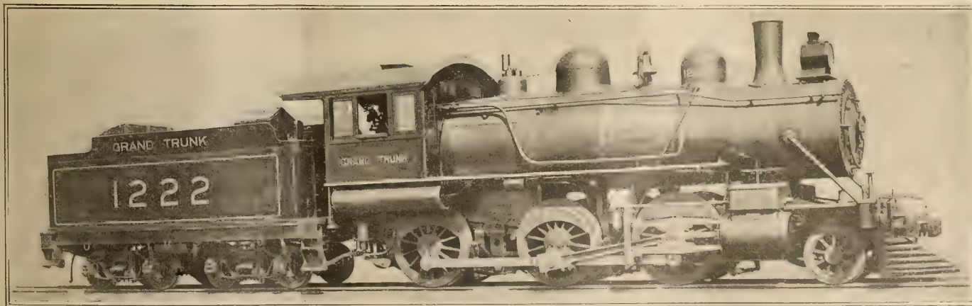
MOGUL LOCOMOTIVE BUILT FOR GRAND TRUNK RY. BY BALDWIN LOCOMOTIVE WORKS.
