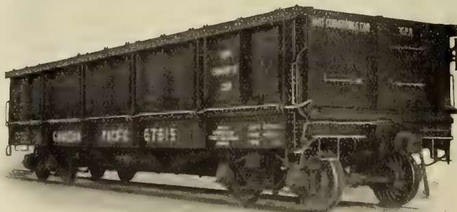
50 Ton Car with Steel Underframe, Steel Stakes, Steel Side Plates and Steel Hopper.
