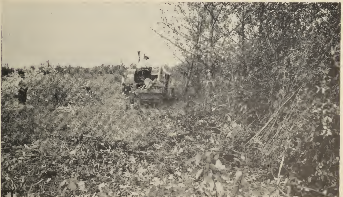
FIG. 5.—Home-made brush cutter at work in light cover. About 5 acres per day may be cleared.
