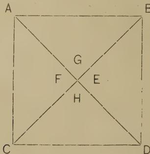
Thus: A, B, C, D, are the four openings of the kiln at the corners; AD and BC are two lines of pipes built on the ground and made hollow for the admission of air.
