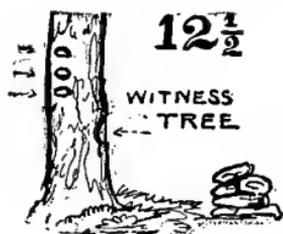
Fig. 12½. Three blazes on a tree indicate an important "line" tree, or more frequently a witness tree for a corner of plot of land; usually another blaze is made on side of tree nearest the stake or stone marking the corner.
