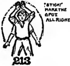
Fig. 213. You are at the right place—Mark it there—Hold your staff there. Signal used when placing a man in line usually the flag-man. (Surveyors' signal.)
