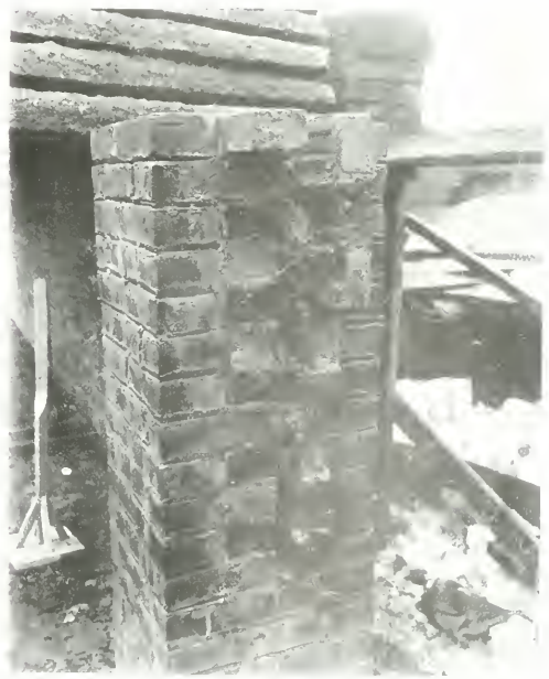
BRICKS CRUSHED BEFORE REINFORCEMENT GAVE WAY.
