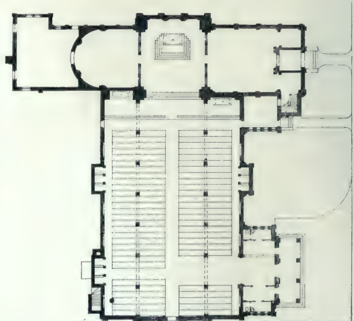
Plan of Our Lady of Lourdes Church, Toronto. Showing the New South Extension, and the Original Structure, which now Forms the Transverse Section. J. P. Hynes, Architect.
