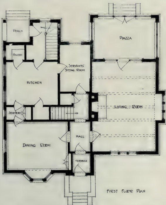
First floor plan, Residence of Mr. F. Christie, Winnipeg. J. D. Atchison, Architect.
