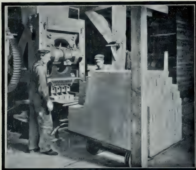
Process View—Showing a Sand-Lime Brick Press with a Minimum Capacity of 20,000 Bricks per Day.
