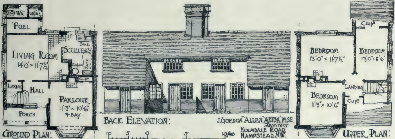
Rear Elevation and Floor Plans of Same House. J. Gordon Allen, Architect.
