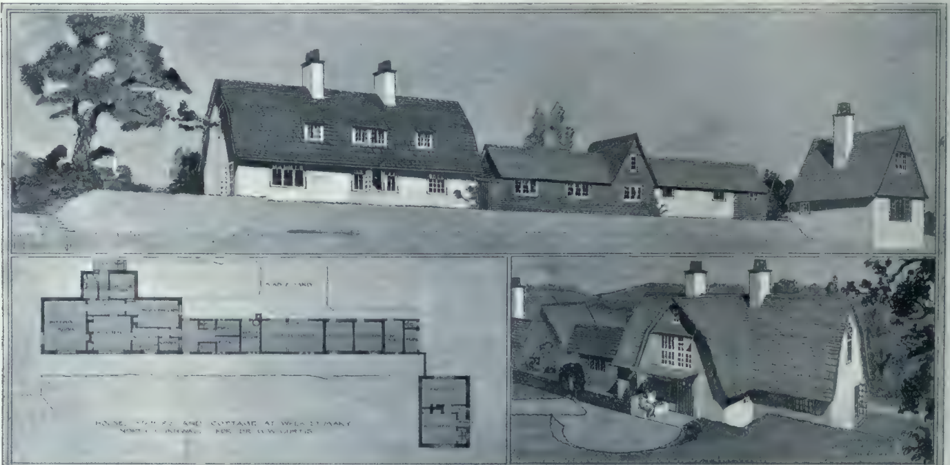
Group of Buildings for Small Holding at West St. Mary. These Structures are of an Extremely Simple and Inexpensive Character. Costing only $4,860 Complete; the House, $2,650; Cottage, $900, and the Stables, $1,300. The Walls for the Most Part are of Brick Roughcast, but Part of the Stables is Weather Boarded and Tarred. The Roofs Throughout are of Delabole Rag Slates. A Noteworthy Feature is the Simply Constructed porch with its Fixed Seat. W. Curtis Green, F.R.I.B.A., Architect.
