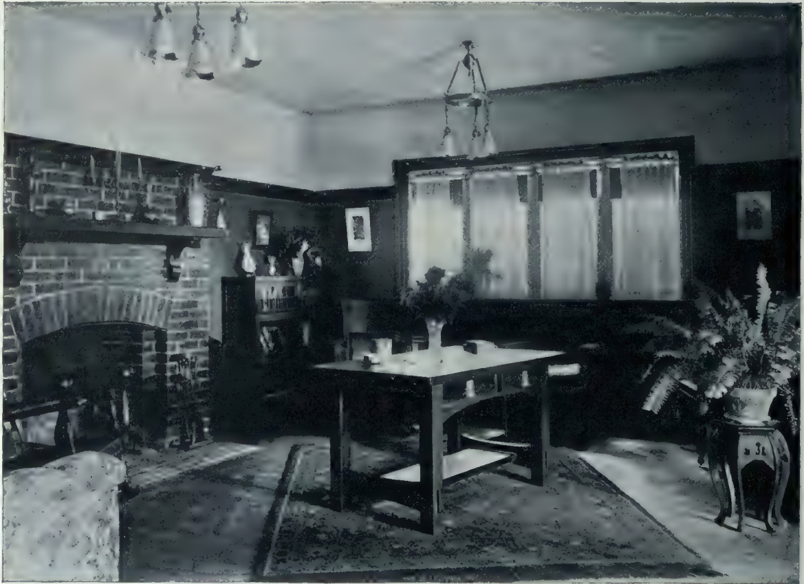
Living Room, Residence of F. A. Coryell, Jameson Avenue, Toronto. An Inviting Interior with a Simple Architectural Scheme, having Walls done in Dark Orange Paper below Plate Rail and Frieze and Ceiling in Gray Stucco. The Fireplace is Built of Red Brick and the Woodwork is Stained a Golden Brown. Chadwick and Beckett, Architects.
