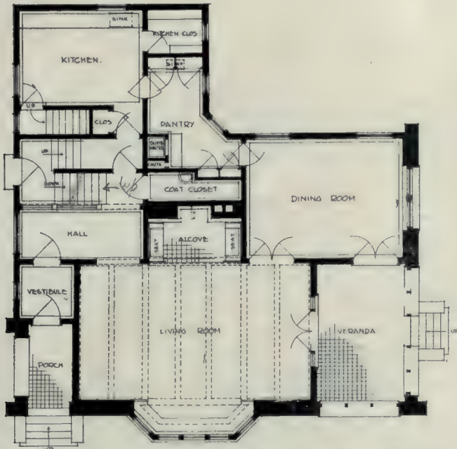
First floor plan, Home of Dr. K. C. Campbell, Ruskin Row, Winnipeg. Note the large living room and the connection between dining-room and kitchen. J. D. Atchison, Architect.
