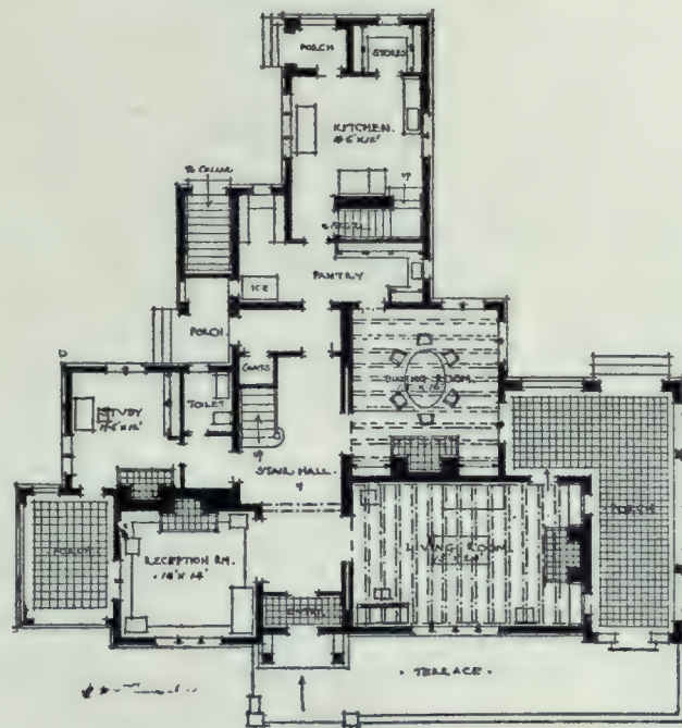
Ground floor plan, Residence of A. B. Steen, Oil City, Pa. Squires and Wynkoop, Architects.
