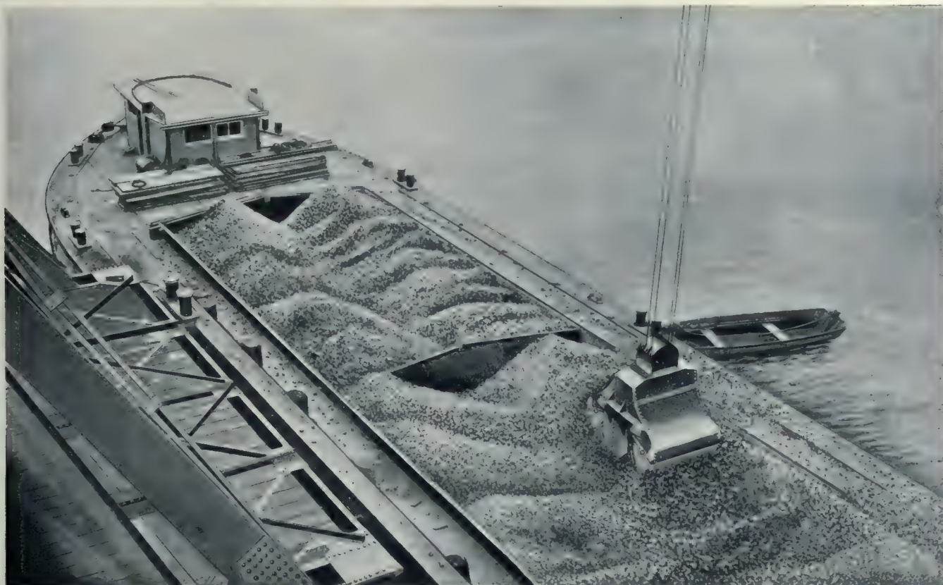
Looking Down at a Loaded Barge from the Operators' Booth, Showing the Ease with which the Operators Direct the Movement of the Grab Bucket.
