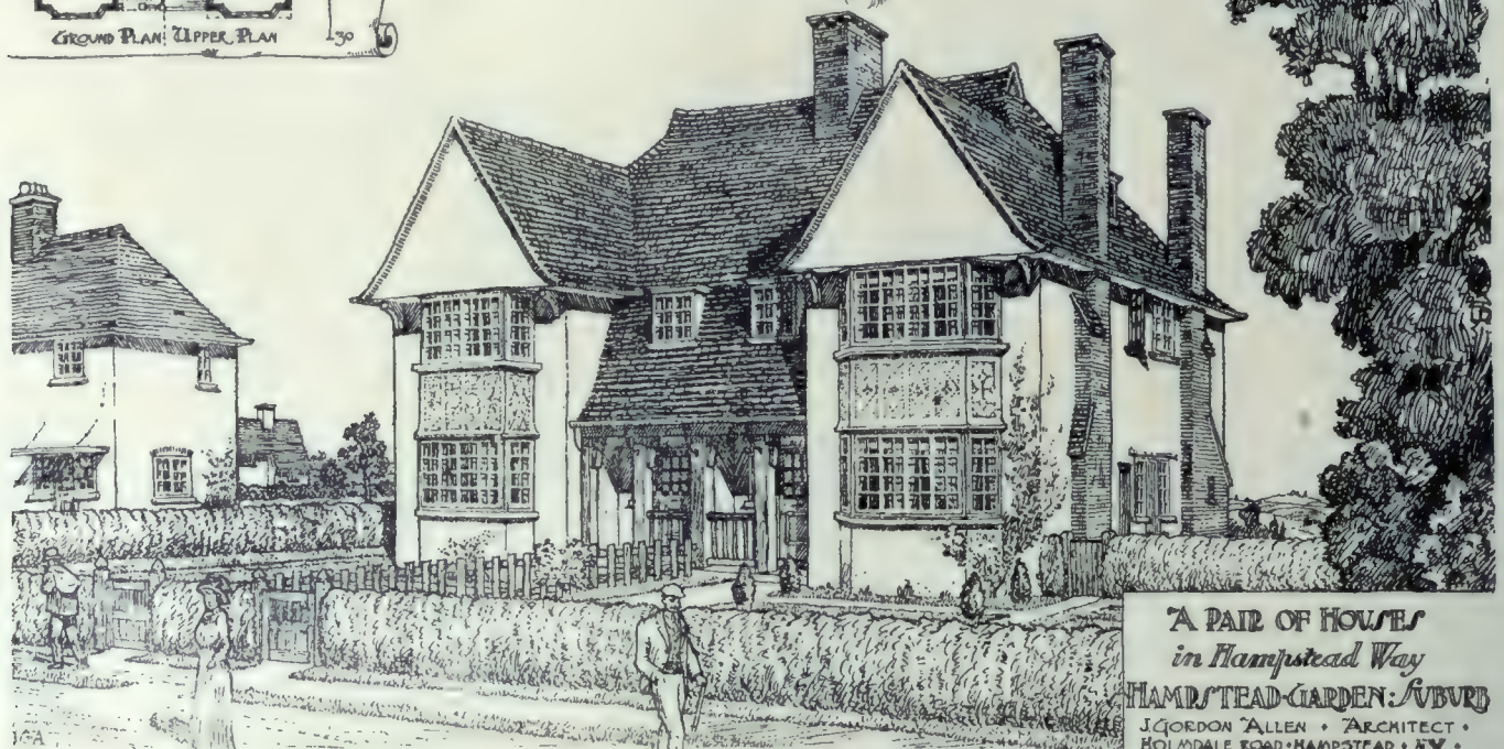
Pair of Houses in Hampstead Garden Suburb. In this Structure the Extension of the Roof Line Down Over the Porches Materially Lessened the Cost of Construction by the Reducing of Brickwork between the Bays to a Minimum. The External Composition is: White Stuccoed Brick Walls with Red Brick Chimney Stacks and Tile Roof. The Post and Beams in the Porches are of Hardwood Left in the Natural State and Unpainted or Unstained. J. Gordon Allen, Architect.
