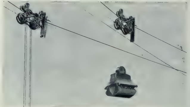
Another View of the Carriage and Buckets, Showing also the Fall-rope Carriers.
