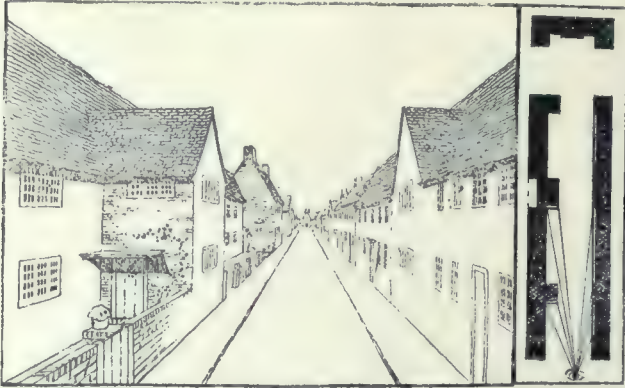
Plan and Sketch of Street, Showing on One Side the Uninteresting Vanishing Perspective of the Unbroken Building Line, and on the Other the More Picturesque Result of Breaks.
