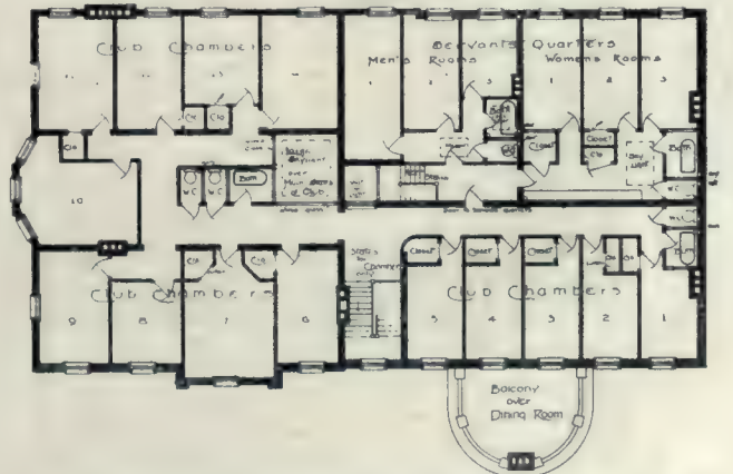
Plan of third floor, Edmonton Club, which is to form a part of future extensions to the building. A. M. Calderon, Architect.
