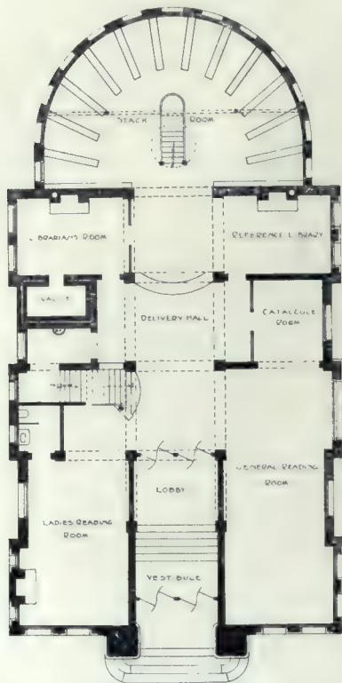
Ground Floor Plan, Public Library Building, Victoria, B.C., Showing General Lay-Out of the Interior and Arrangement of Stack Room. Thos. Hooper, Architect.
