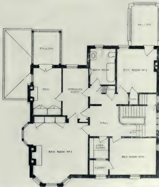
First Floor Plan, Residence of F. L. Ratcliff, 145 Crescent Road, Toronto. Burke, Horwood and White, Architects.
