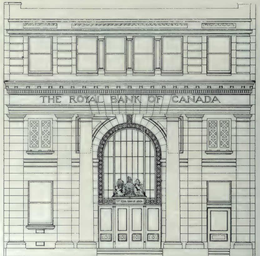
Front Elevation, Recently Erected Premises of the Royal Bank of Canada on Government Street, Victoria, B.C. This Front is Executed Entirely in a Rich Native Granite, Even Unto the Latticed Windows, Which are Cut Through Three-Inch Stone Slabs. Thos. Hooper, Architect.
