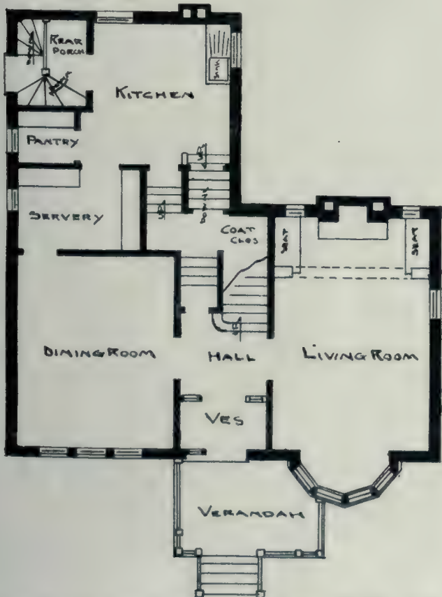
Ground Floor Plan, Residence of W. Carter, Dunvegan Road, Toronto. Bond and Smith, Architects
