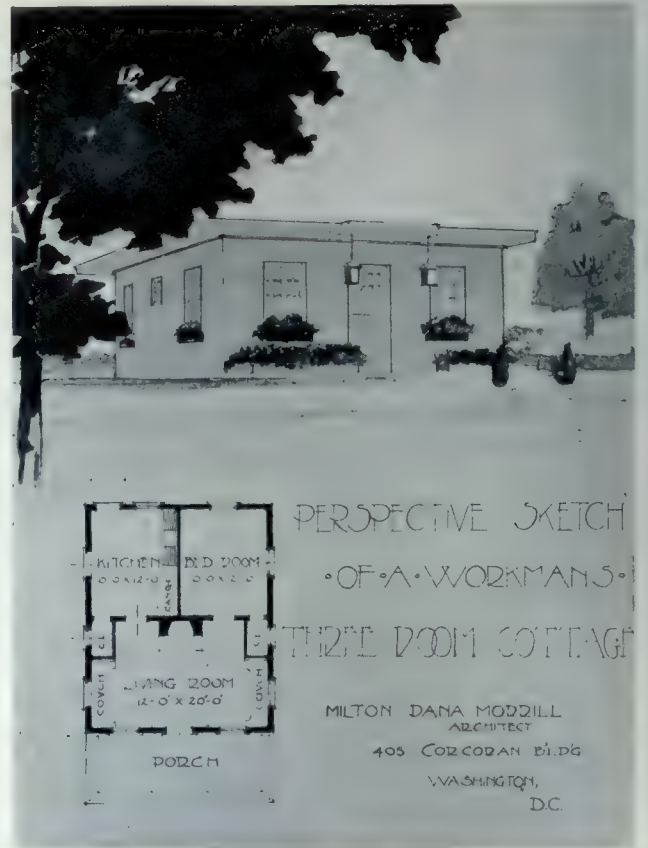
Perspective Sketch and Floor Plan for a Three-Room Workman's Cottage. Note the large living room with alcoves at each end fitted with couches. These can be transformed into bedrooms by sliding curtains. The chimney of the fireplace also serves the kitchen, and a shower bath can be installed in one of the closet spaces if so desired. Milton Dana Morrill, Designer.
