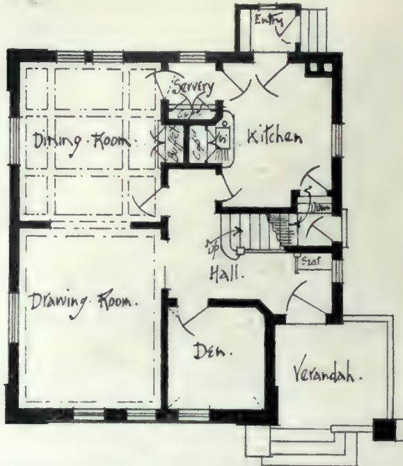
Ground floor plan, Residence of W. B. Van Egmond, Regina. Storey & Van Egmond, Architects.
