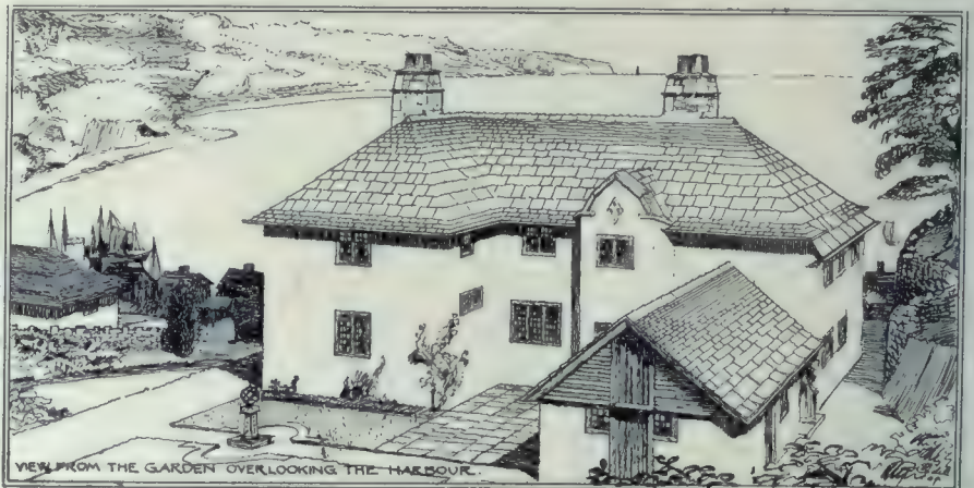
Rear View, House at Brixham. This House is Built of Stone Quarried on the Site. The External Treatment is Roughcast and the Roof is of Delabole Rag Slates. W. Curtis Green, F.R.I.B.A., Architect.
