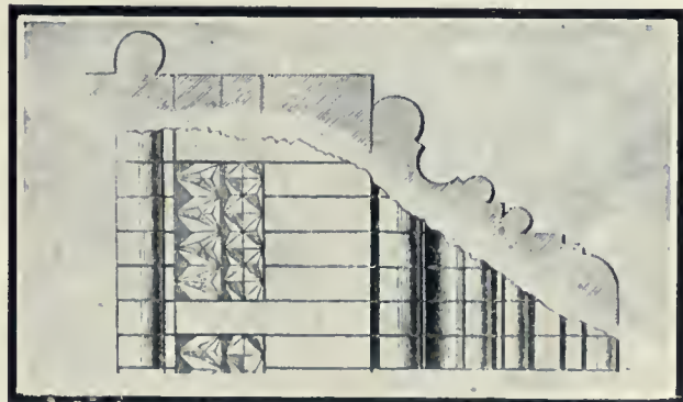
Detail of window-jamb, Cremona, Italy.
