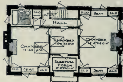
First floor plan, Design No. 2, a feature of which is the sleeping porch, projecting slightly beyond the outside wall.
