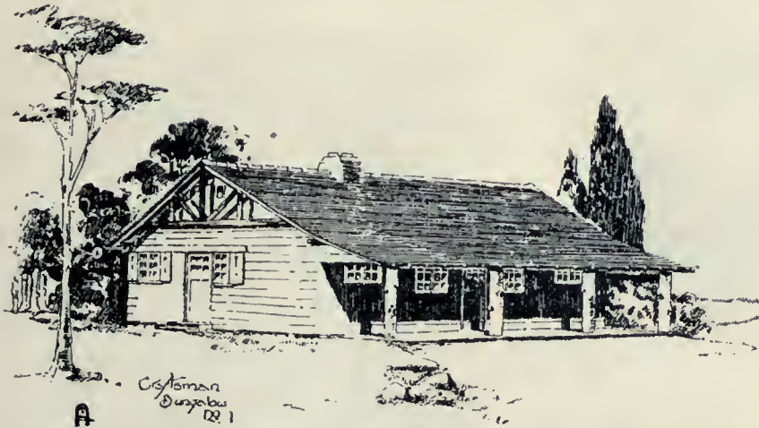
Design No. 7.—A craftsman bungalow, sheathed with boards 8 x 10 inches wide, 7/8 of an inch thick, laid like clapboards. Note the truss of hewn timber in the gable, which not only forms a decorative feature, but gives added support to the roof.
