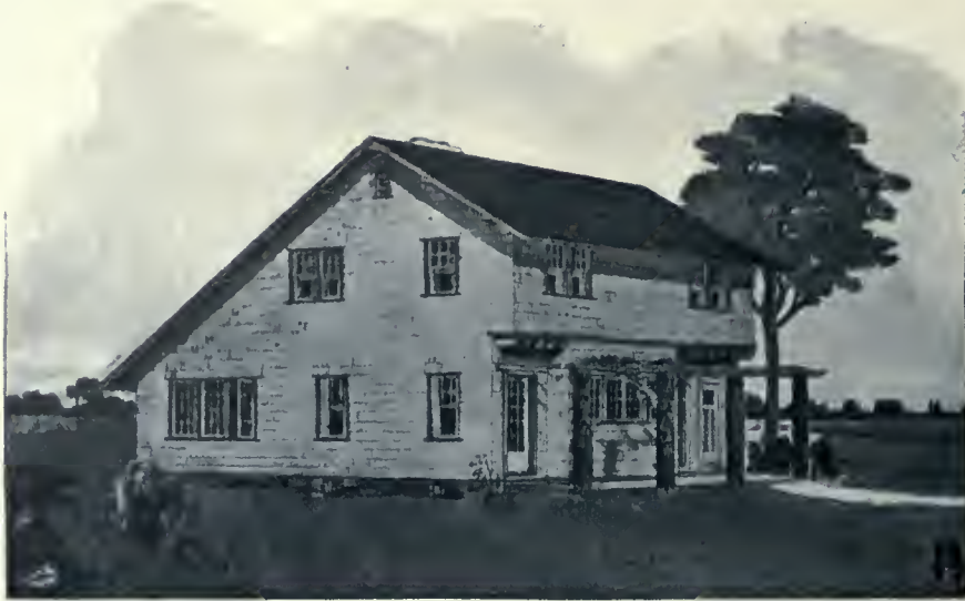
Design No. 4.—Front view of an unusually graceful design for a suburban house. The walls are covered with shingles or clapboards; the roof shingled; the terrace of cement or vitrified brick. The pergola, which is shown in this view, is of a rustic character.
