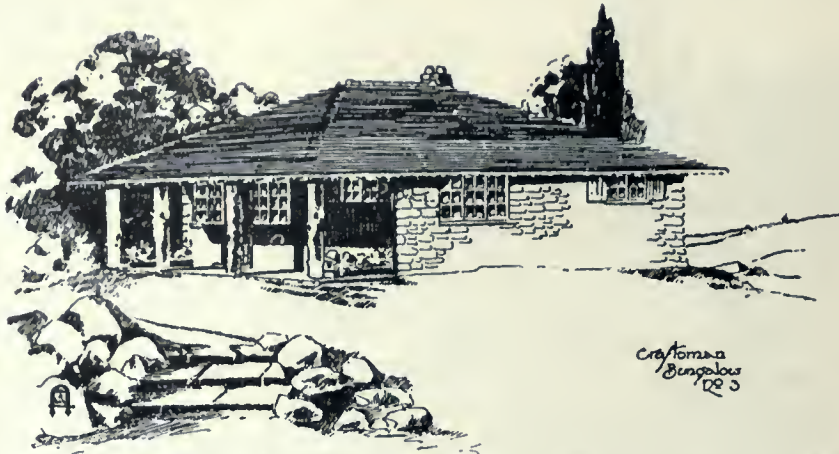
Design No. 9.—A craftsman bungalow with walls of field-stone. Note the usual bungalow roof, low pitched, square in line and widely overhanging. It extends in front, without a break, over the porch, and is supported by rustic pillars.
