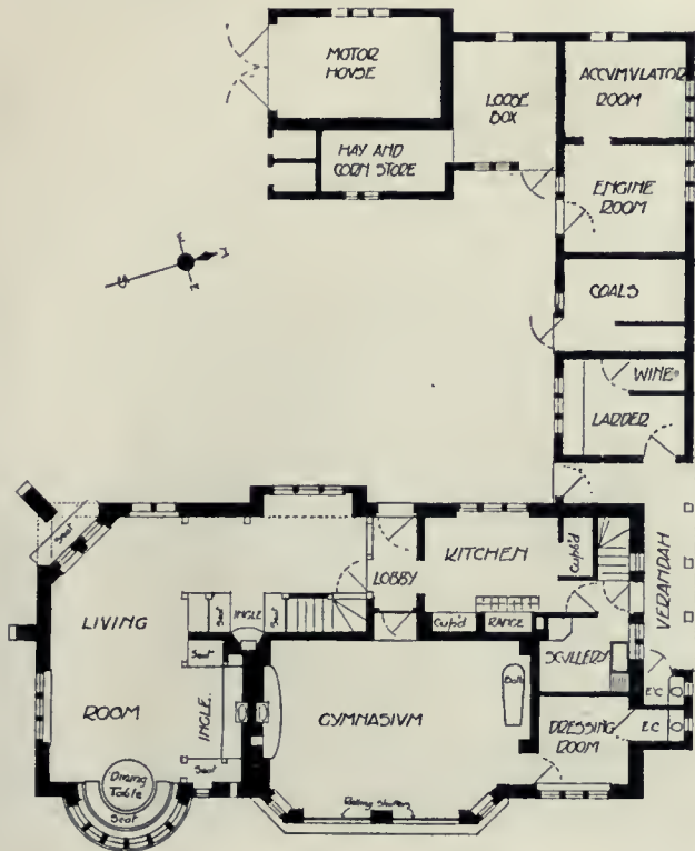
Ground floor plan, Home of W. E. Steers, at Caterham, Surrey, showing the large private gymnasium, and the arrangement of the various rooms. The main entrance opens onto a spacious court at the south-east corner of the living room. Messrs. Unwin and Parker, Architects.
