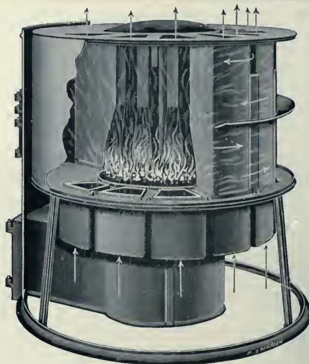
Sectional Diagram, showing Interior of Combustion Chamber, Position of Hot Air Columns and Direction of Fire Travel. Record Calorific Warm Air Heat Producer.
