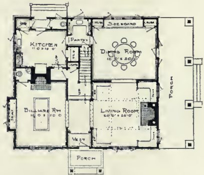
Ground floor plan of Design No. 1, showing the location of the fireplaces and the positions of the built-in features.
