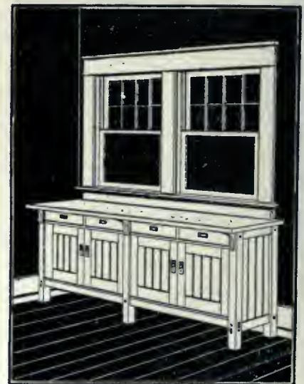
Figure 15.—Built-in counter shelf.
