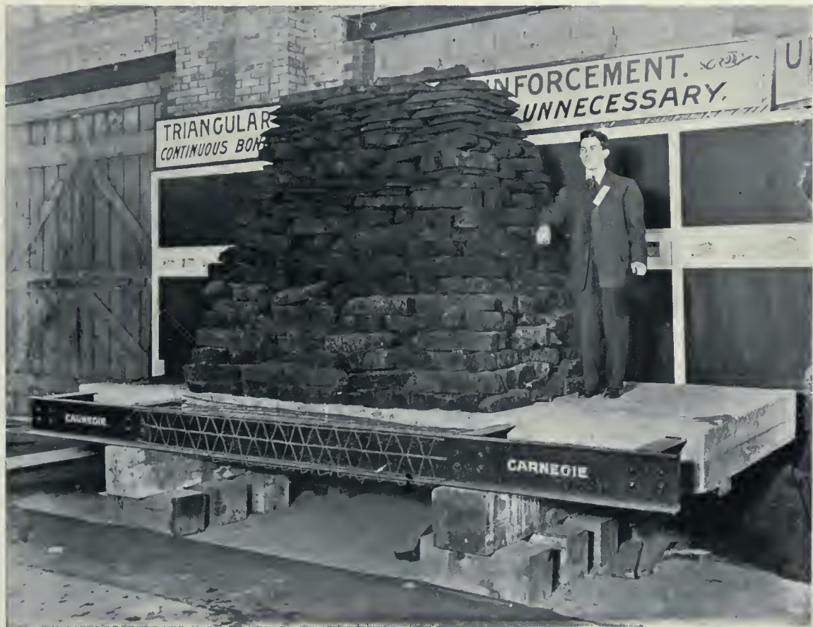
CONCRETE SLAB TEST MADE AT RECENT CEMENT SHOW, TORONTO, SHOWING THE PANEL AS IT APPEARED WHEN SUBJECTED TO 52,900 LBS.
