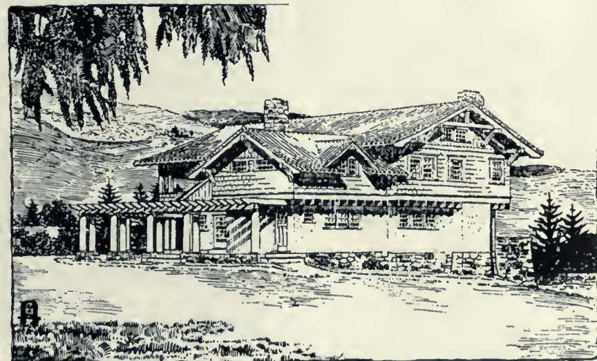
Front view of Design No. 5. This design is suitable for cement or brick, or wood construction, and the roof is equally well adapted to tiles, slates or shingles.
