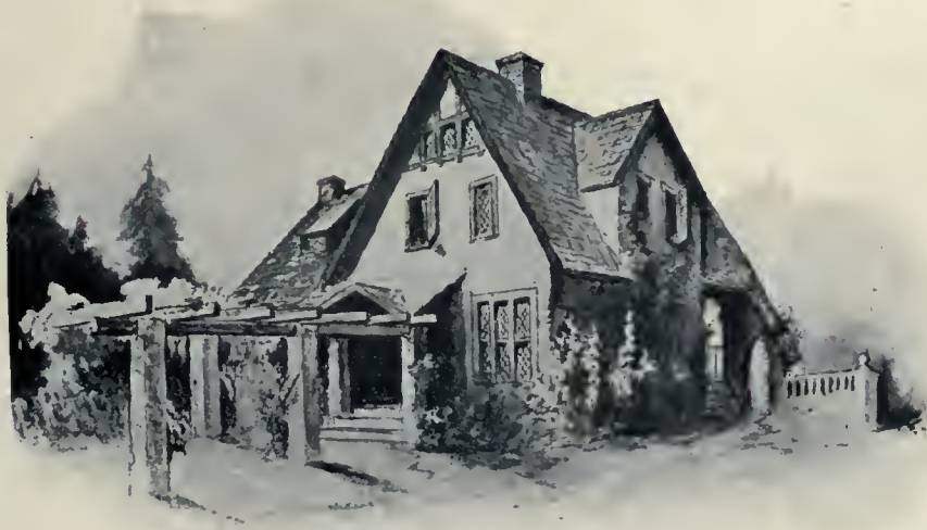
Rear view, Design No. 3, showing the roof lines and treatment of windows. The pergola having concrete posts, opens off the entrance of the porch, where the family dinner can be served during the summer months.
