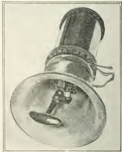
An Auxiliary to the Wireless The Electric Bell, Fixed on a Vessel Below Water, Which Gives the Position of the Ship
