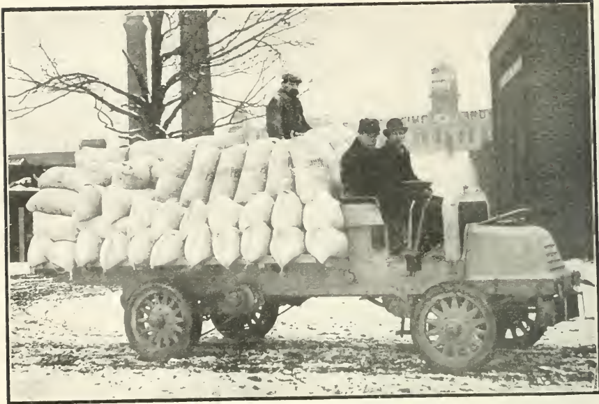
A Motor Dray With Capacity of Five Tons
