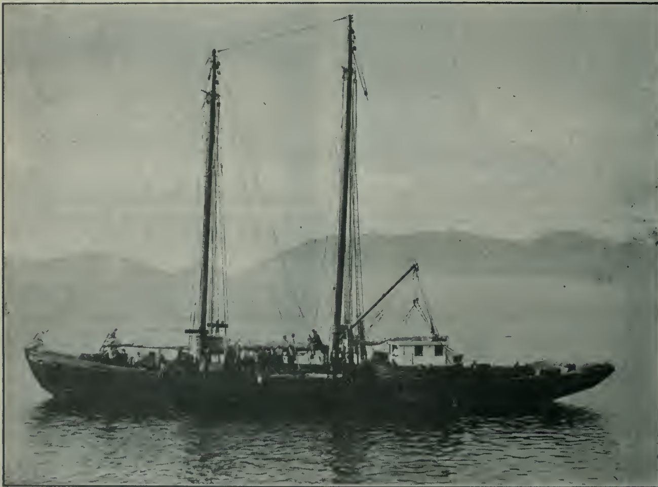
Sails Cut Down—Power Installed. An Auxiliary Fishing Schooner.
