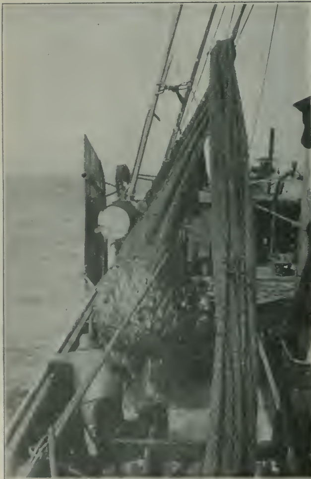
The Bag on Deck. Ready to pull the draw rope of the cod end.
