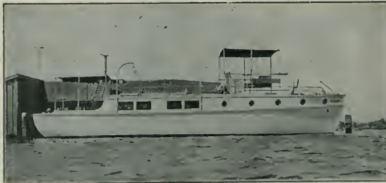
47 ft. x 10 ft. 6 in. Cruiser "Remington," equipped with a 46 H.P., 4 Cylinder, Remington Oil Engine.
