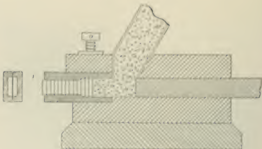
FIG. 155—Section of Briquette Press.
