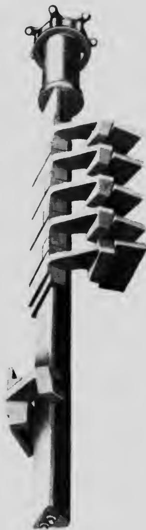
Wedge mechanical roaster. 1. Rabble arm 2. Arm dressed with rabble blade holders and blades 3. Arm partly dressed with holders and breech block
