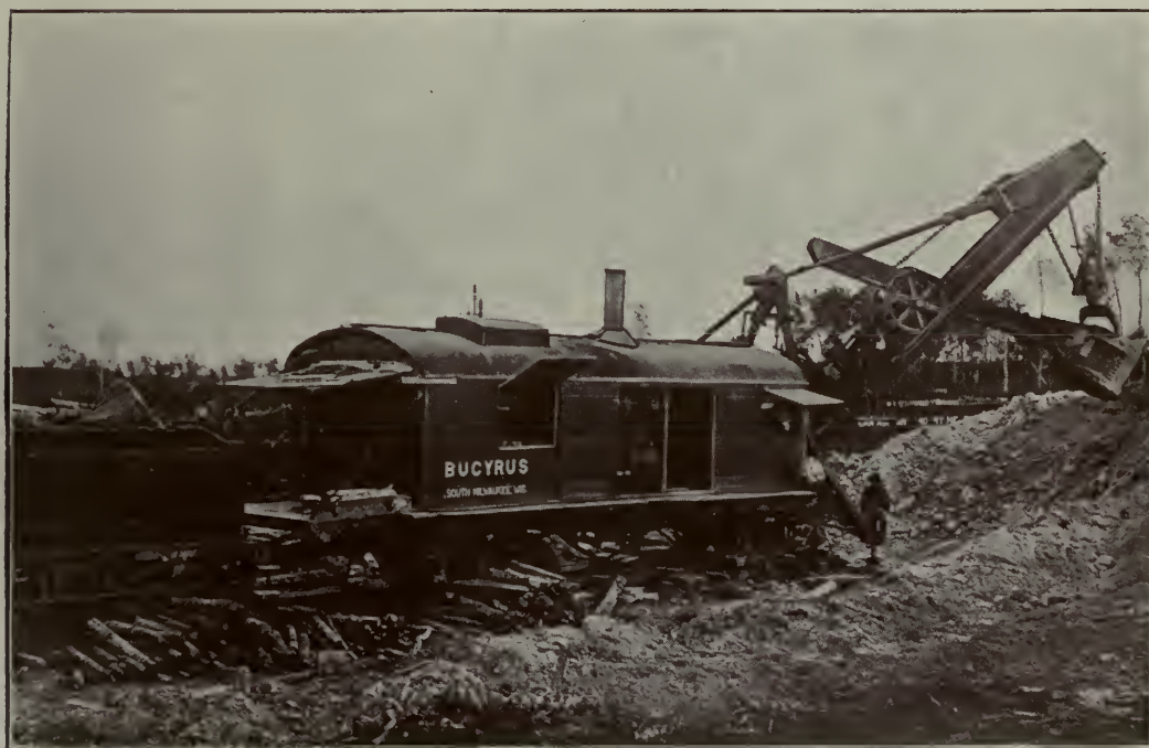
B. Steam shovel loading gypsum into cars, Manitoba Gypsum Company's quarry, Gypsumville, Man.
