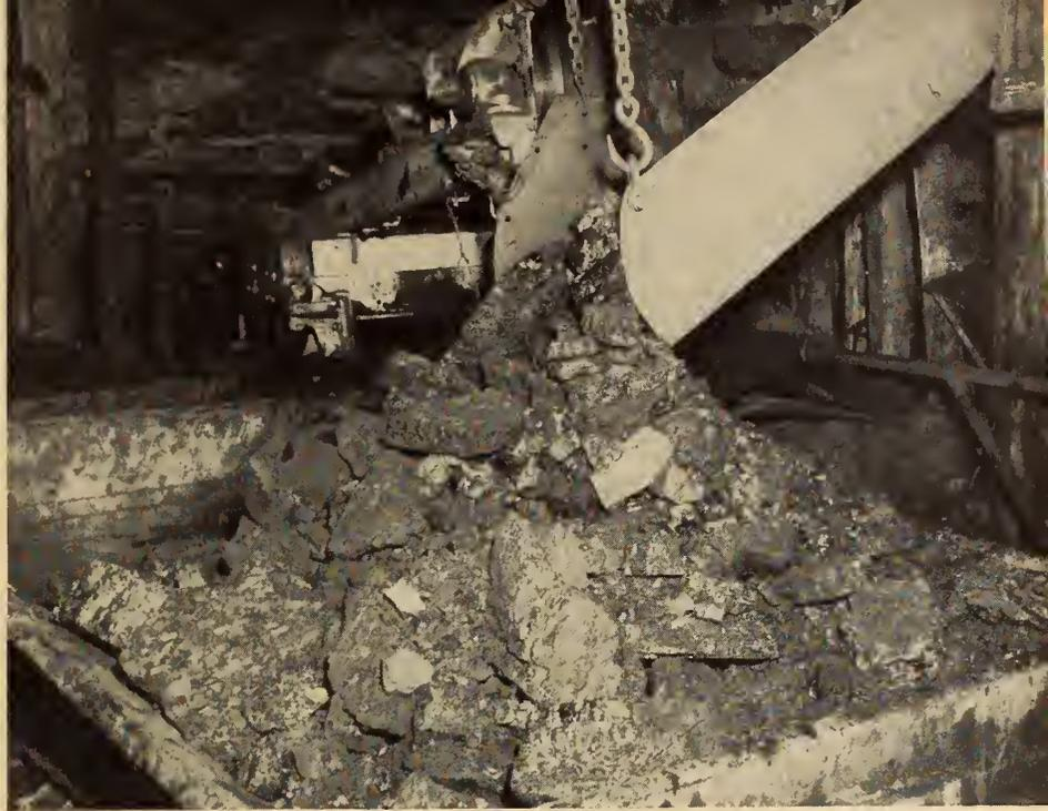
Fig. 7. Loading mine car at end of conveyor belt.
