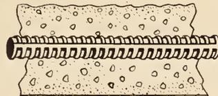
Irrespective of the position in which they are cast HI-BOND bars provide a greater mechanical grip in the concrete and, therefore, offer higher resistance to slippage.
