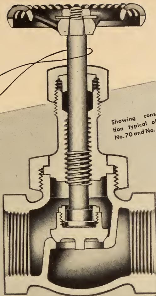
WHEREVER severe service conditions on steam, water, oil or gas, dictate the need for tight valves with metal-to-metal seating (although not requiring the more specialized plug-type disc used on exceptionally severe throttling, blow-down and similar service)—the Crane Nos. 70 and 370E “regrinding” valves are in popular demand, particularly in the marine field.
