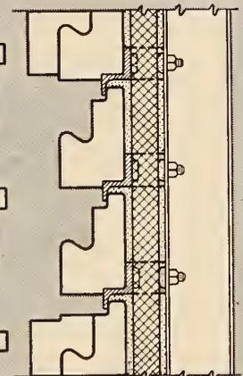
New tile ready to be set in place. Unit-suspension avoids cumulative loading.
