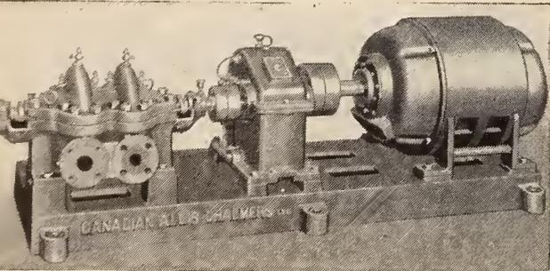
C A-C type "CM", two-stage, high-pressure pump driven by 1450 rpm motor through a step-up herringbone gear set at 3500 rpm. Pump illustrated has 2" suction, 1½" discharge.
