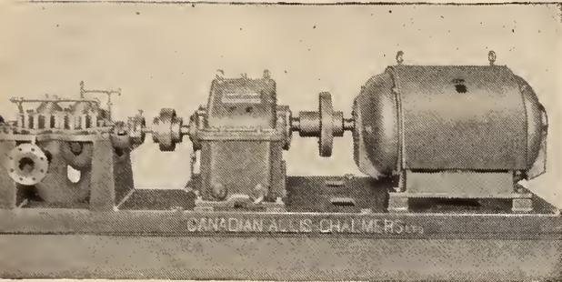
CA-C, 6" suction, 4" discharge type "MM", two stage, double-suction, stainless steel pump. Rated 600 Imp. G.P.M. against 1125' head, 3550 rpm driven through step-up gear by 300 hp, 1470 rpm motor.
