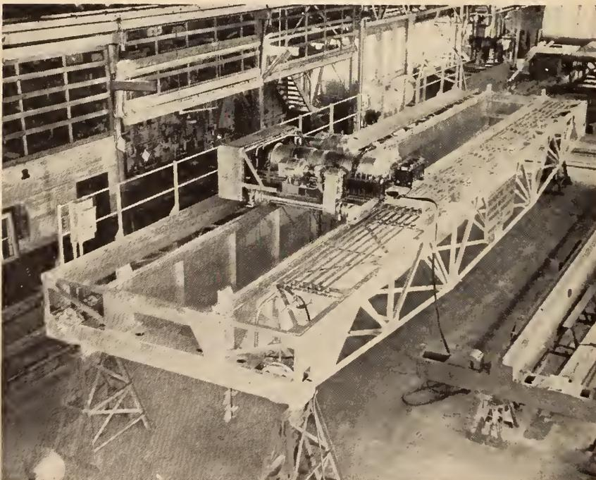
An Aluminum Welded Overhead Electric Travelling Crane of 15 tons capacity, 55 feet span, has been designed and fabricated by Provincial Engineering Ltd., Niagara Falls, Ontario. It is believed to be the first welded aluminum crane in the world. It is now in operation at the plant of the Aluminum Company of Canada, Kingston, Ontario.
