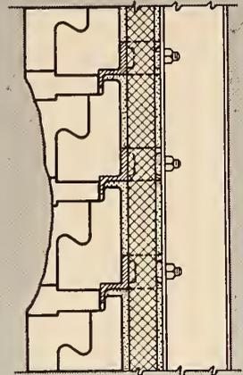
Worn section of wall. Damaged tile ore chipped out, adjacent areas untouched.
