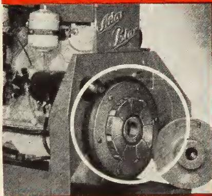
Type SRC-50 BLM Clutch with drive body applied directly to flywheel of Chrysler engine. Drive controlled from throttle. Driven body removed to show mechanism.
