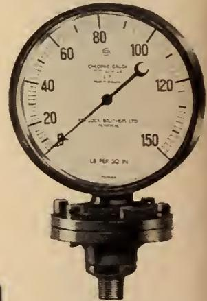
Above — Budenberg Diaphragm Gauge. These Schaffer pattern gauges for low and medium pressures are not damaged by rough usage and are ideal for viscous or corrosive fluids. Also available are Bourdon gauges and Steel-tube gauges for high pressures.
