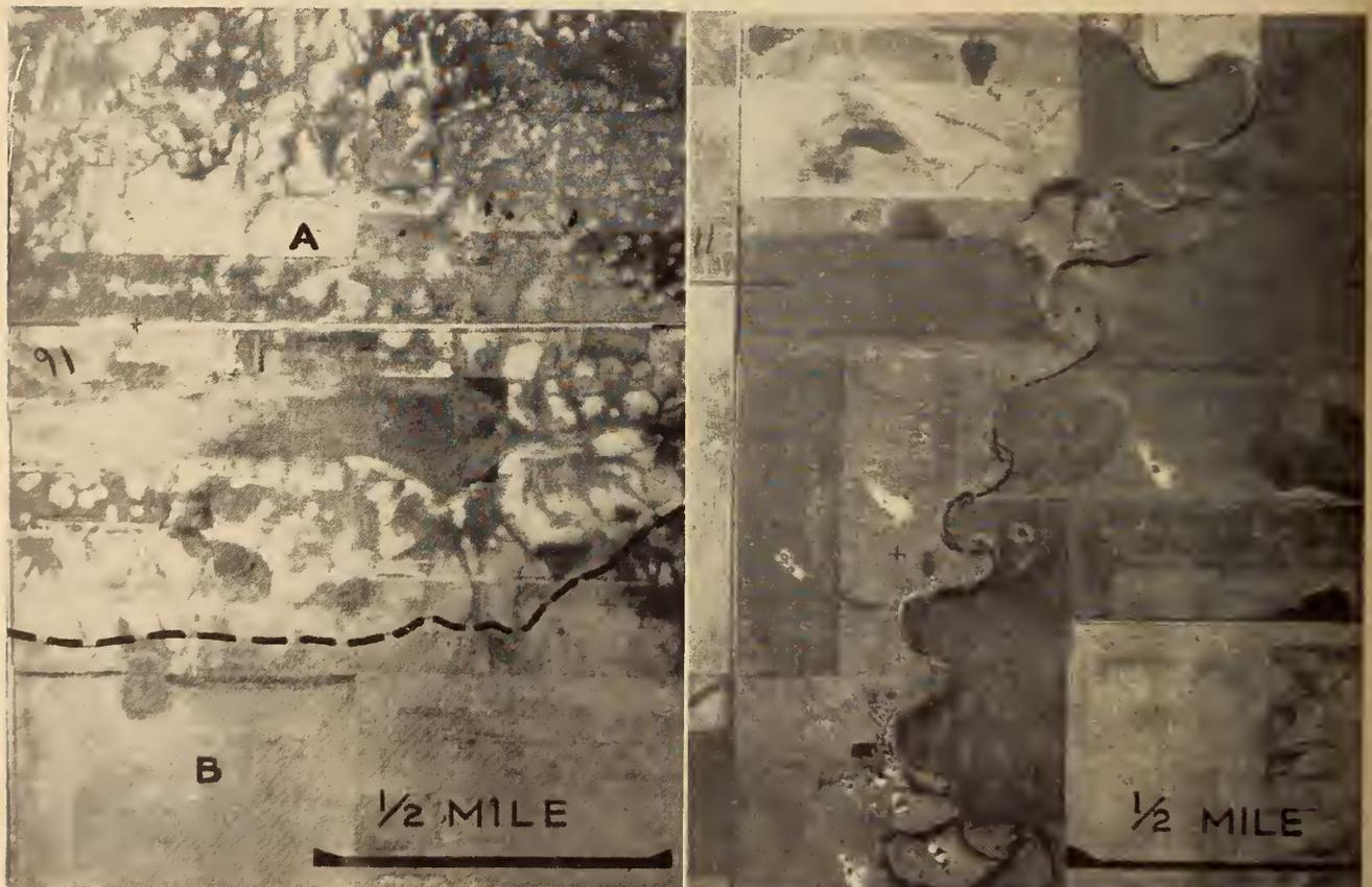
no runoff would be expected to reach the river. Ground-water supplies are favourable, since water will be found entrapped in sand and gravel lenses. Although borrow materials are available, the hilly terrain is not suitable to highway or airport construction. Farm lands will be correspondingly poor in these vicinities because of the rough topography, high losses of moisture by rapid runoff, and high proportion of wasteland caused by wet depressions ⑩.
