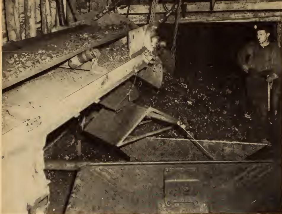
Fig. 4. Discharge end of level conveyor belt.
