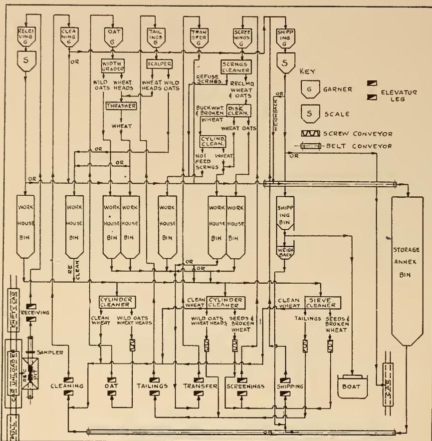
Fig. 3. Typical flow diagram of a terminal grain elevator.
