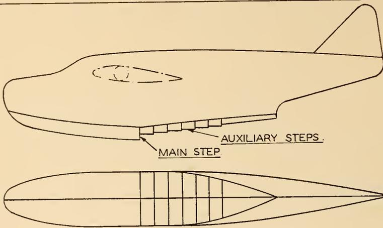
MULTI-STEP HULL ON BV 238 FLYING BOAT.
