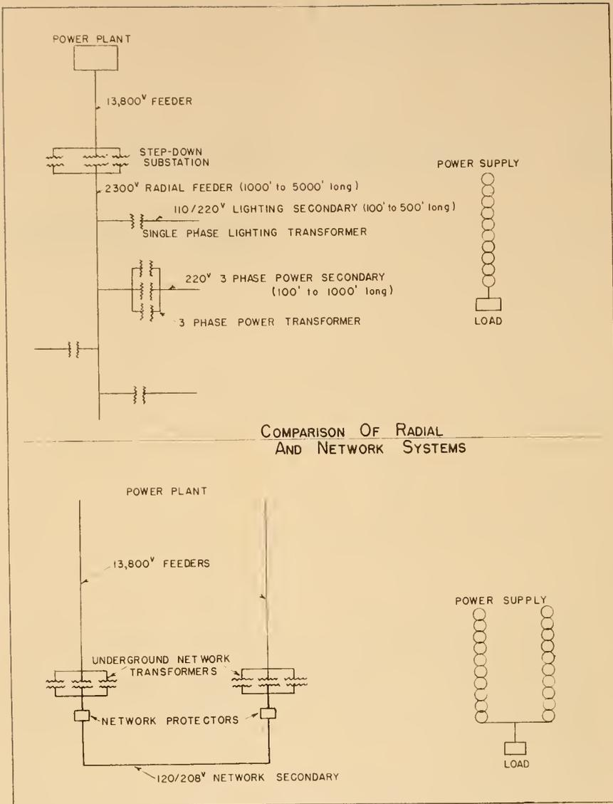
Fig. 1. Comparison of radial and network systems.
