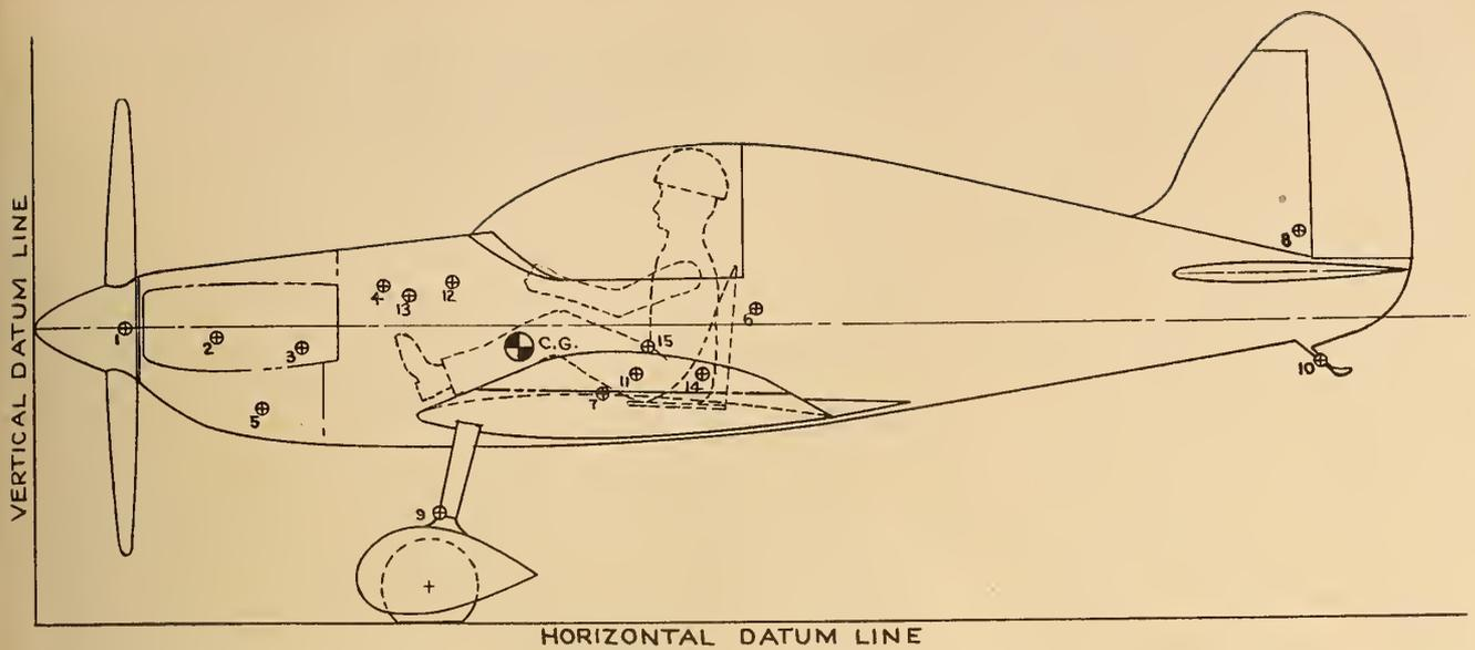
Fig. 3. Balance diagram. See Table I in conjunction with this diagram. Centre of gravity is 17 per cent aft of leading edge of the mean aerodynamic chord.
