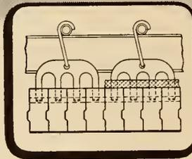
A cross section showing offset tile and prong-type supporting casting.
