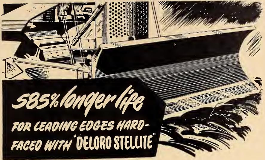
★ Behind this scraper lies 24,000 lbs. weight and driving power. Tough Grade 6 Deloro Stellite hardfacing kept this blade work-worthy nearly six times longer than the original hard steel.
