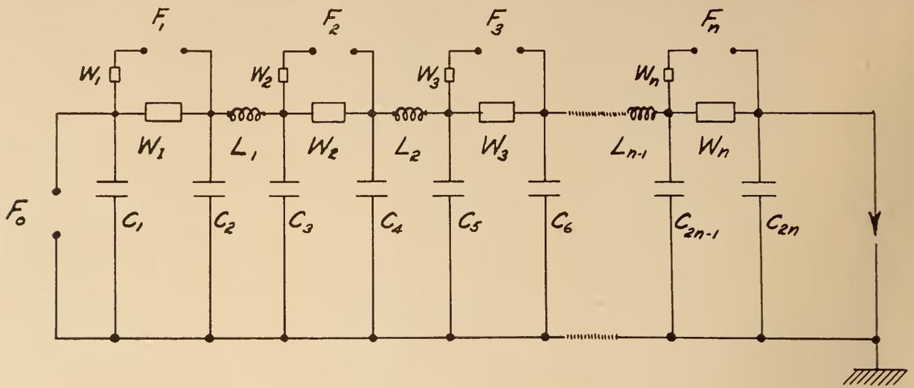
Fig. 3. Electrical arrangement for multiple spark photography.
