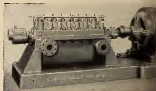
C A-C type "M" 6-stage double-suction, high-pressure pump driven by 400 horsepower, 1800 rpm motor.
