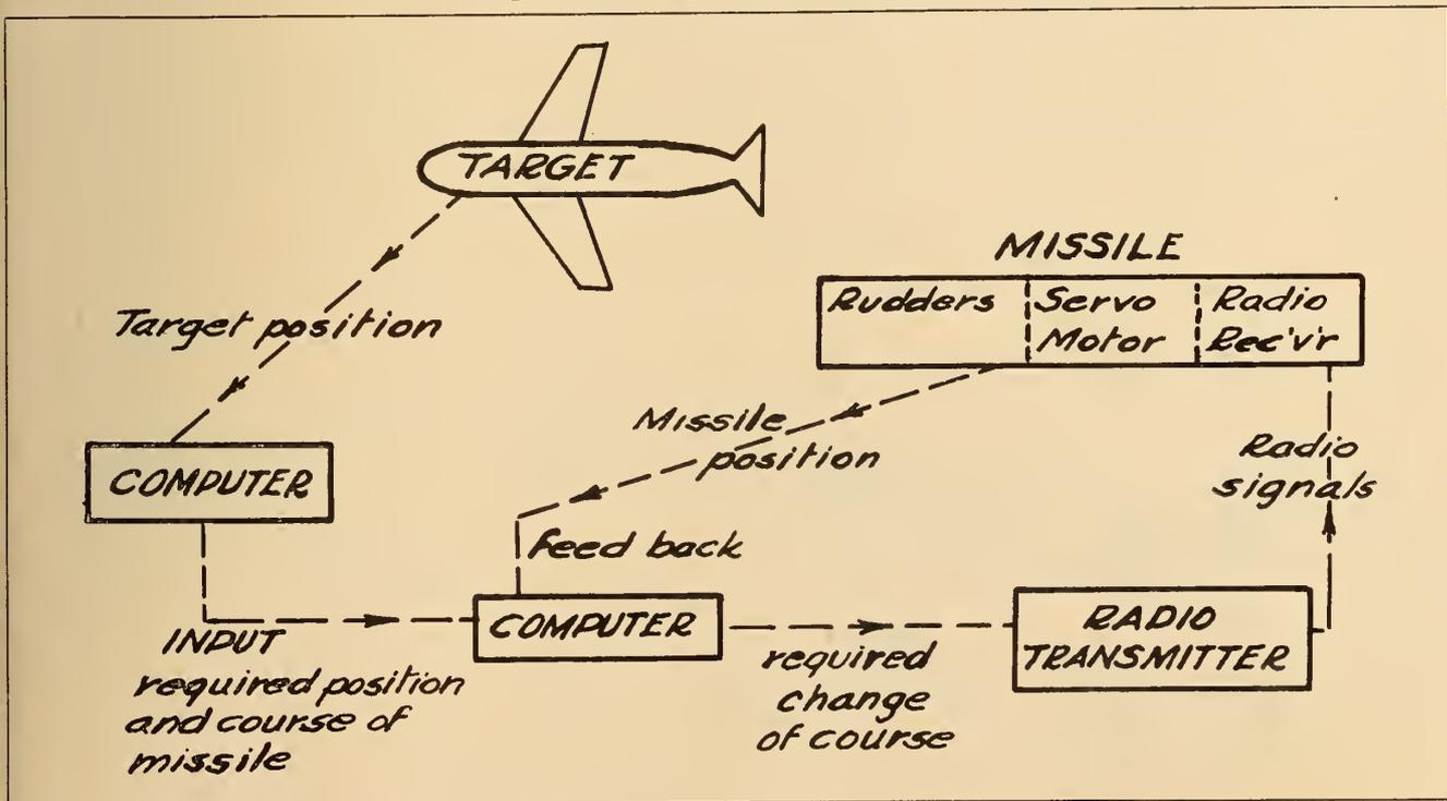
the missile en route relative to this flight path; and (4) telling the missile what changes in course or speed it should make to get on the desired path. These phases of guidance are followed by the so-called control phase, in which a force is made to act on the missile to change its motion in response to the guidance information.
