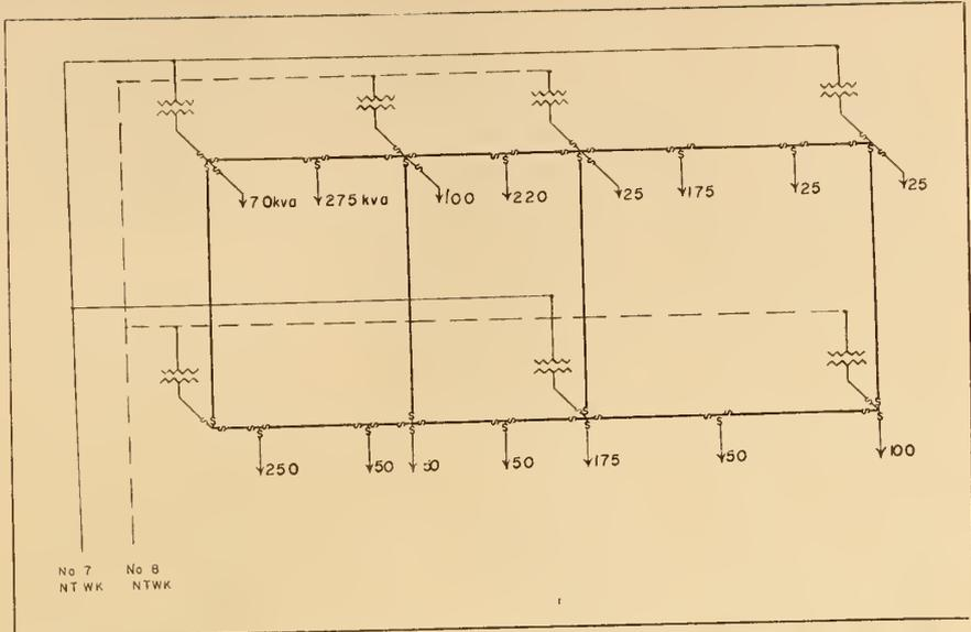
Fig. 2. Schematic drawing of underground network, showing locations of limiters and size of loads.
