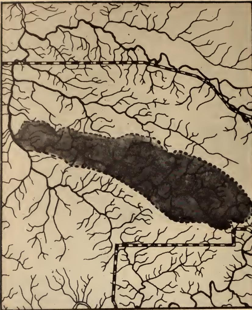
Fig. 2. Drainage map. Use of the drainage map for computing watershed areas in rough terrain. This map has been prepared from aerial photographs.
