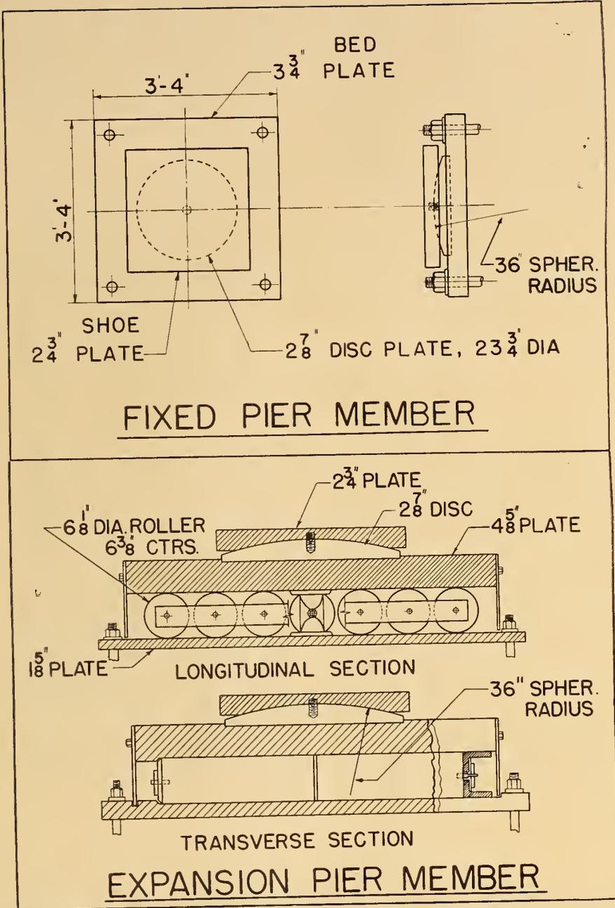
Fig. 7 and Fig. 8 (above) illustrate fixed pier member and expansion pier member.
