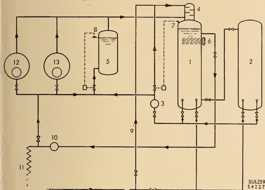
Fig. 6. Diagram of an electric hot-water accumulating plant in a textile factory.
