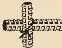
HI-BOND bars stay anchored when they are crossed and wired because the ribs key into each other and hold firmly.
