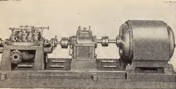
High-head mine pumping unit. Type "MM", two-stage, double suction, extra heavy centrifugal pump, driven through herring bone gear, speed increaser. Motor speed is 1450 rpm which is increased to 3500 rpm of the pump.
