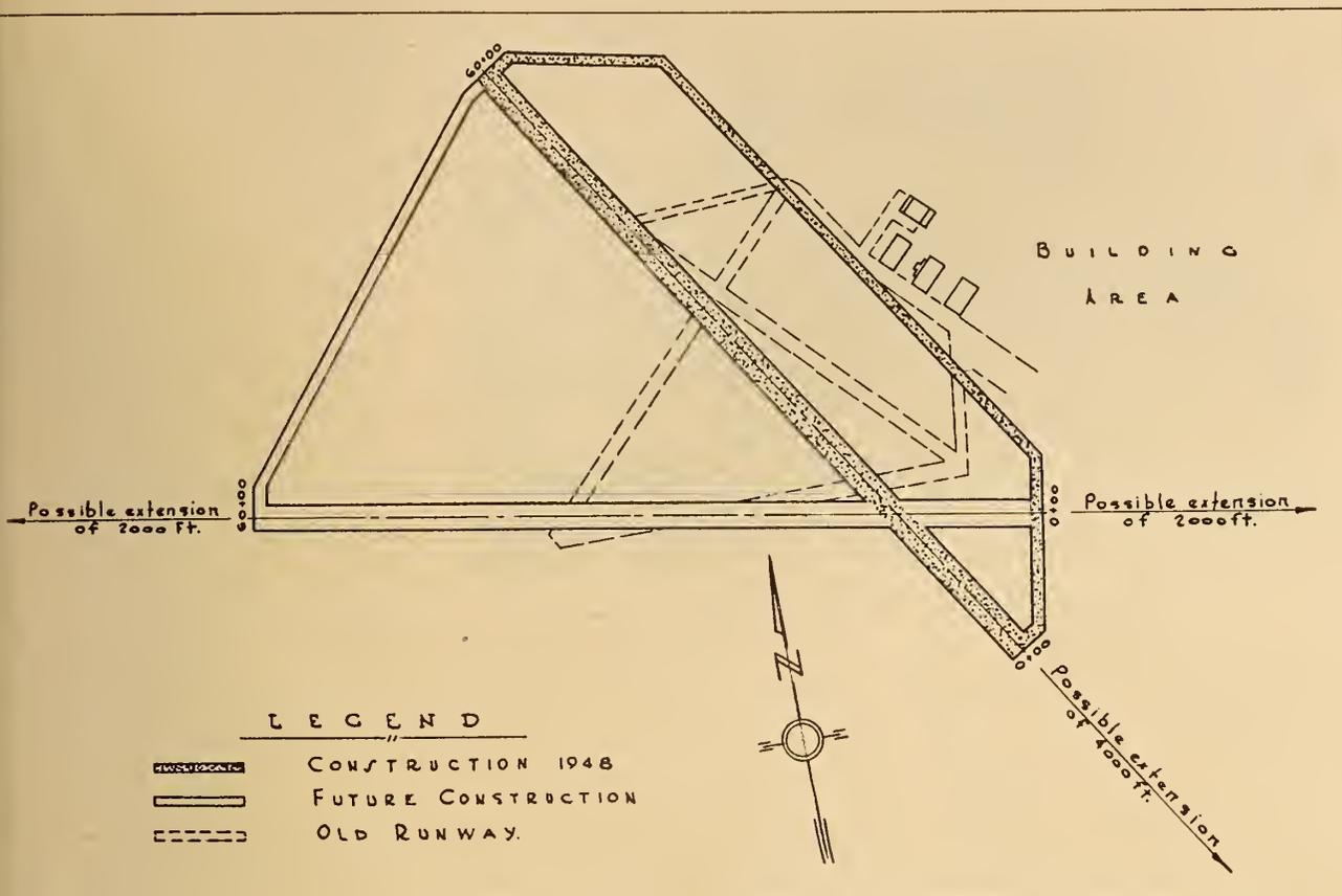
Fig. 1. Plan for improved runways at Rivers, Manitoba.
