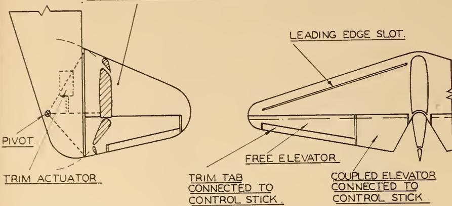
MANUAL ELEVATOR CONTROL ON BV238 FLYING BOAT.
