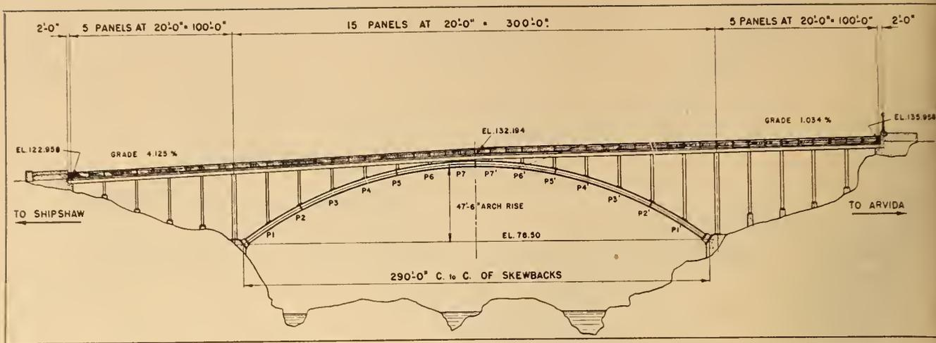
Fig. 2. Elevation of Aluminum Highway Bridge at Arvida.
