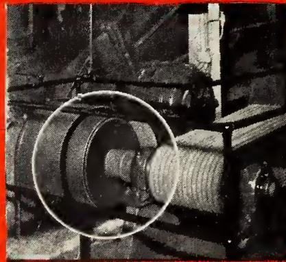
Type SC-45 Clutch with eleven groove "V" Sheave in drive to pulverizer in pulp mill (Hinde & Dauche Company Limited).
