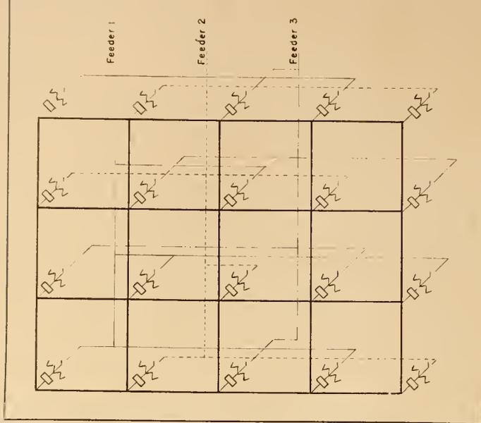
Fig. 4. Schematic diagram showing the basic arrangement of primary feeders, network transformers, and secondary mains in a low voltage secondary network.
