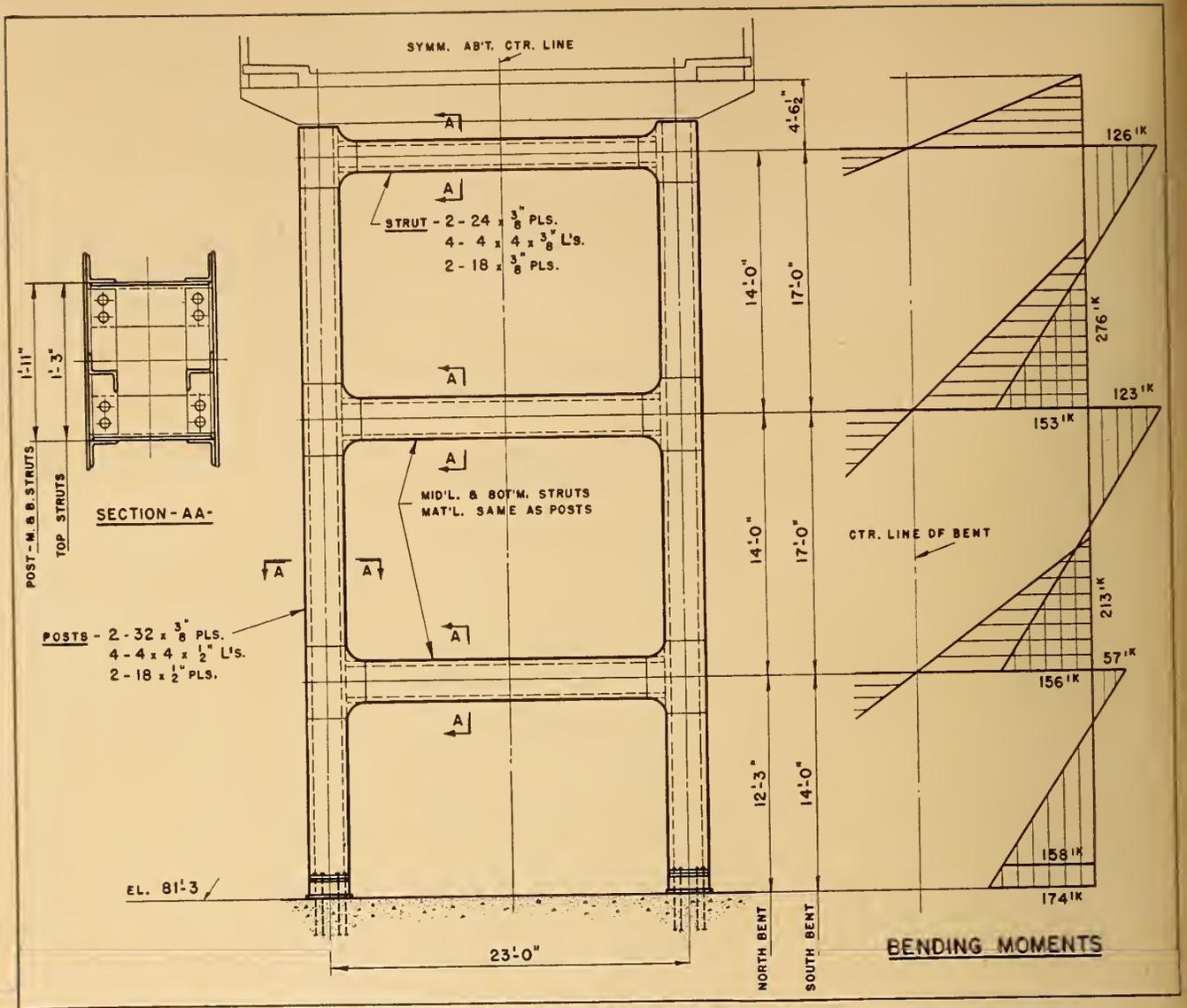
Fig. 4. Bents at Skewbacks.
