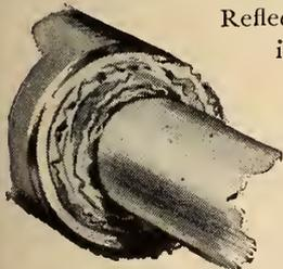
Reflects 95% radiant heat. An ideal insulation for boilers and steam piping. Helicallly-wound aluminum foil-air heat insulation is fireproof and permanent. It will not absorb water in the event of leakage.
