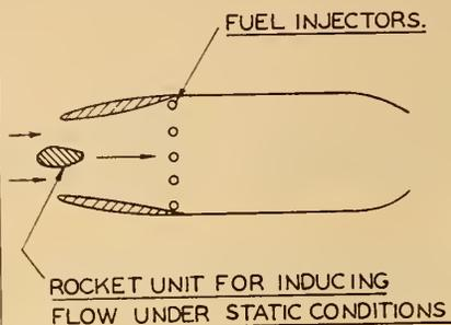
ROCKET BOOSTED PROPULSIVE DUCT
