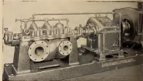
C A-C type "CMSK", size 5" by 3", 3-stage, double-suction bearing stainless steel mine pump. Capacity 360 U.S. G.P. against 1075 feet head at 3500 rpm.
