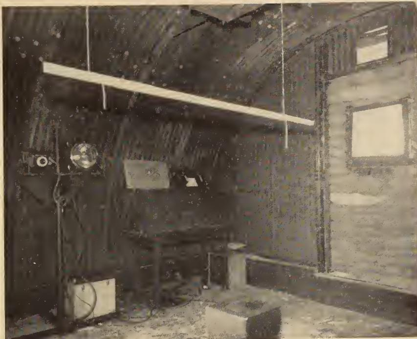
Fig. 5. Range set-up for single flash photography of projectiles.
