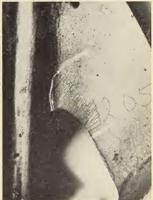
Fig. 6—Angle bracket after loading. Note cracks in lacquer. Direction of stress is at right angles to cracks.
