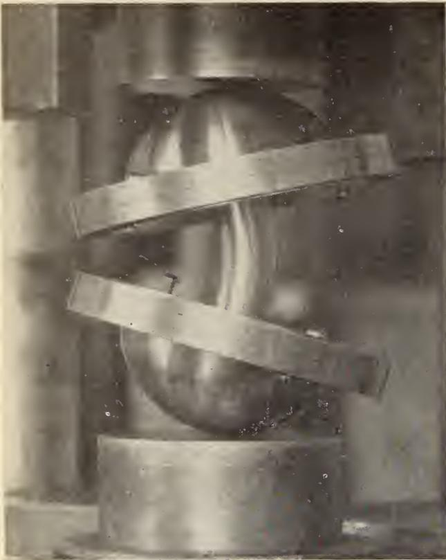
Fig. 14—Showing pin-ended column under test.
