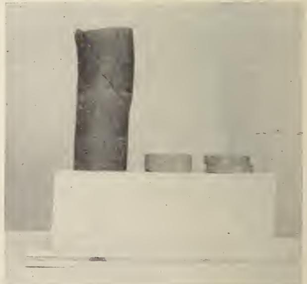
Fig. 10—Soil specimens showing shear planes.
