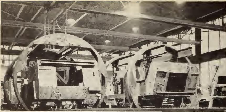
Fig. 7—Roll-over positioner used on production line.
