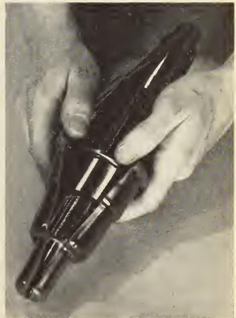
Stripcoat has been slit and is about to be removed from shaft. Note cleanliness of machined surfaces and the exactness with which the coating has followed the contour of the part.
