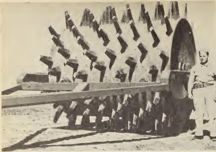
Fig. 15—Sheepsfoot roller used by Army engineers. (Acme Photo)
