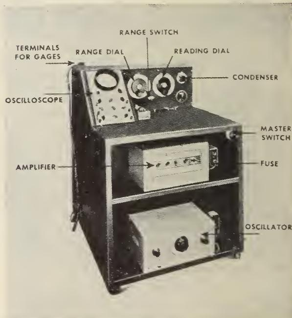
Fig. 4—Dynamic strain recorder used at the Bureau of Mines' physical metallurgy research laboratories.
