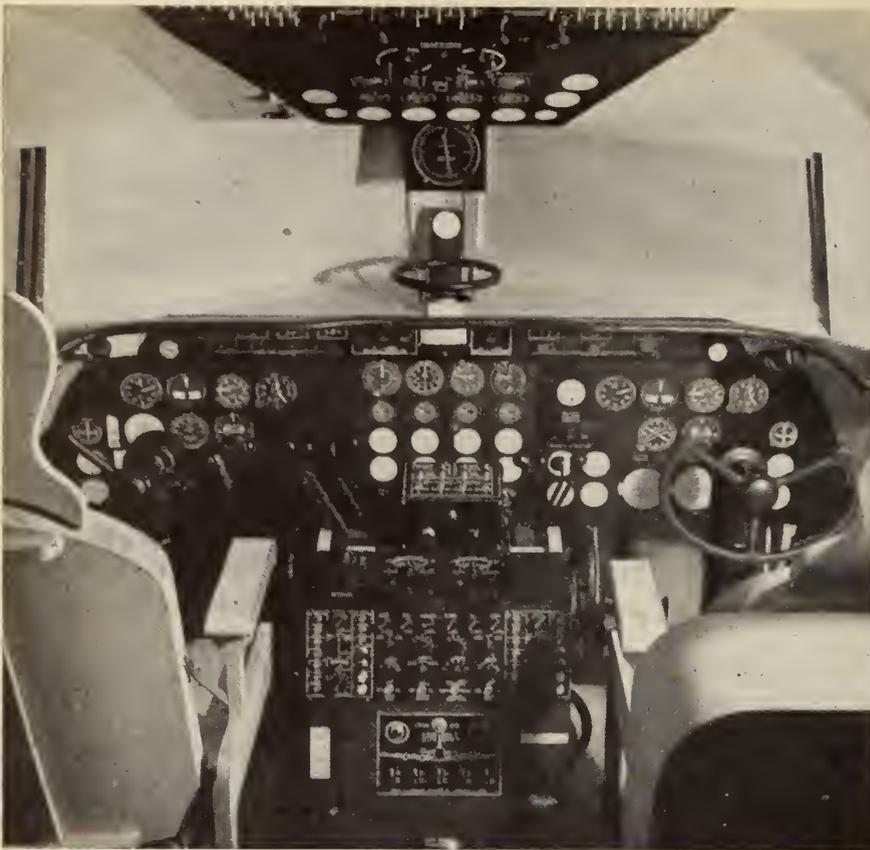
Fig. 7—"Mock-up" of pilots' station in flight compartment.
