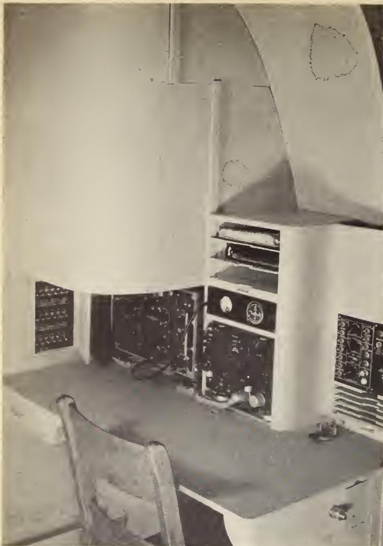
Fig. 9—"Mock-up" of radio operator's station in flight compartment.
