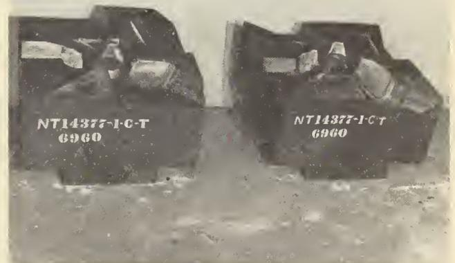
Fig. 2—Finishing dies.
