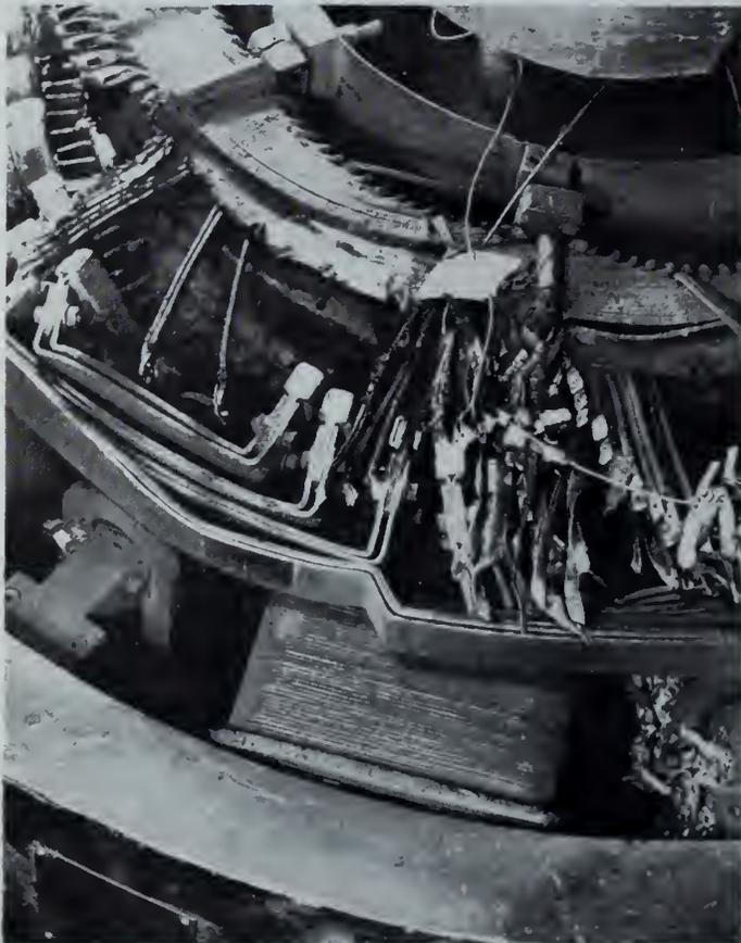
Fig. 7—Showing damage to armature and field coil winding of a paper machine drive generator. The accident was due to the banding wire supporting the armature conductors breaking or burning and allowing the armature conductors to come out of the slots.
