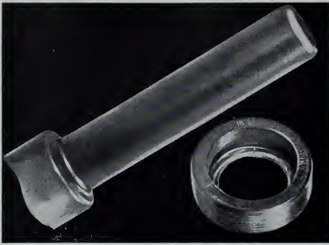
Fig. 1—Silver-brazed detonator exploder and threaded collar.
