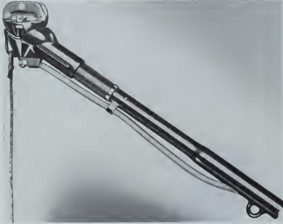
Fig. 3—Shoe collector with carbon insert.
