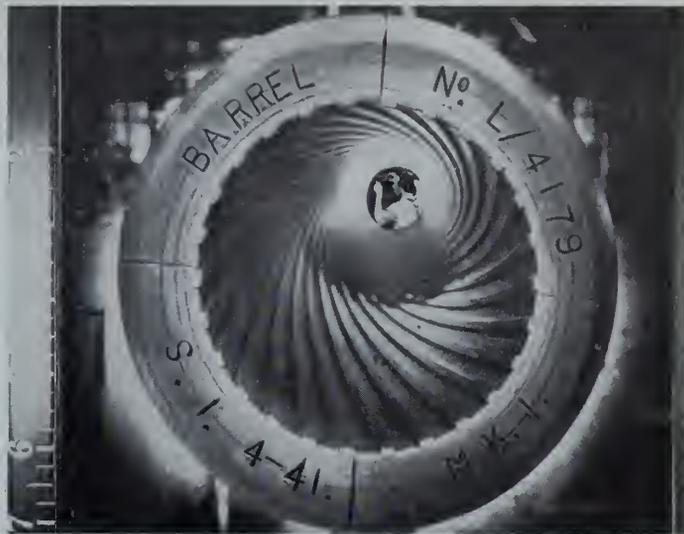
Fig. 6—Muzzle of 25-pounder barrel showing rifling.
