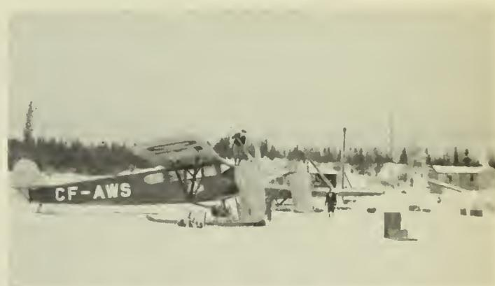
Fig. 3—Winter operating base at Oskelaneo, P.Q. Fairchild 71C and Junkers W34, also loading crane, winter engine covers, radio masts, etc.
