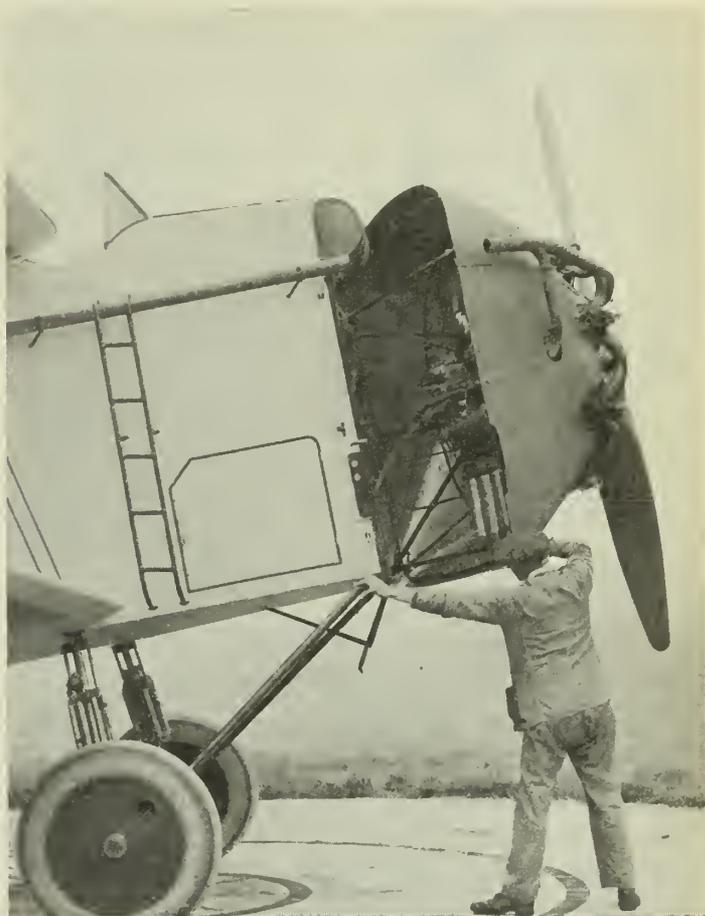
Fig. 4—Swinging Engine Mounting of the Bristol Brandon Biplane.
