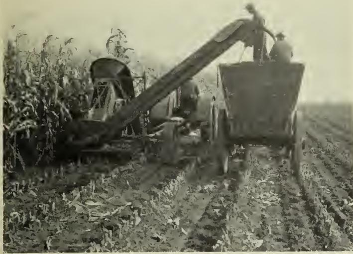
Fig. 2—The combined corn harvester and silage cutter has been used successfully for many years on the Central Experimental Farm, Ottawa.
