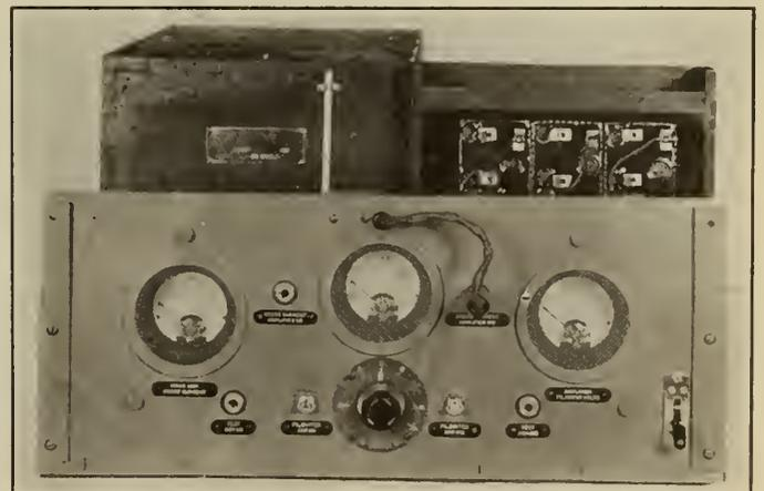
Figure No. 21.—Canadian Radio Beacon Transmitter—Front View of One Tuning Fork Panel, showing the Controls.
