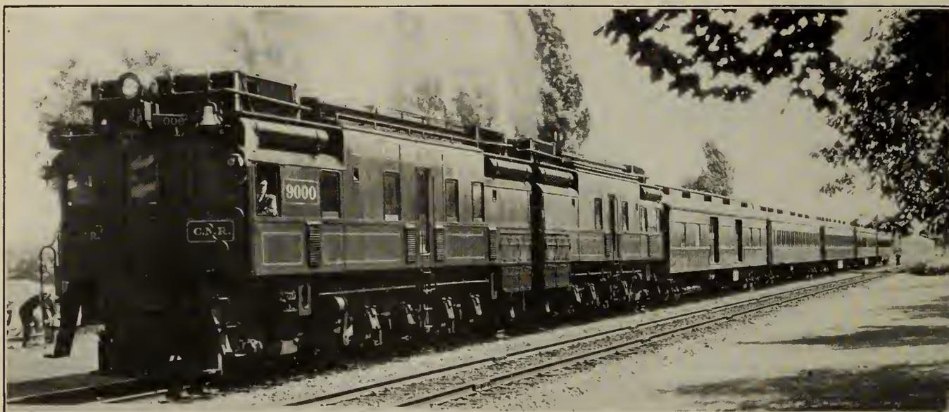
Figure No. 3.—“9000” Type Oil-Electric Car.
