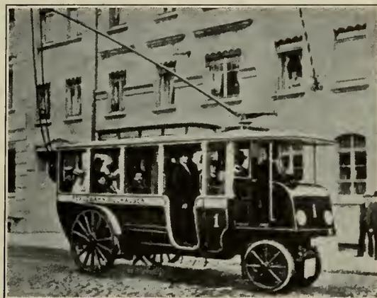
Figure No. 3.—Trolley Bus with Single Trolley Pole at Mülhausen.
