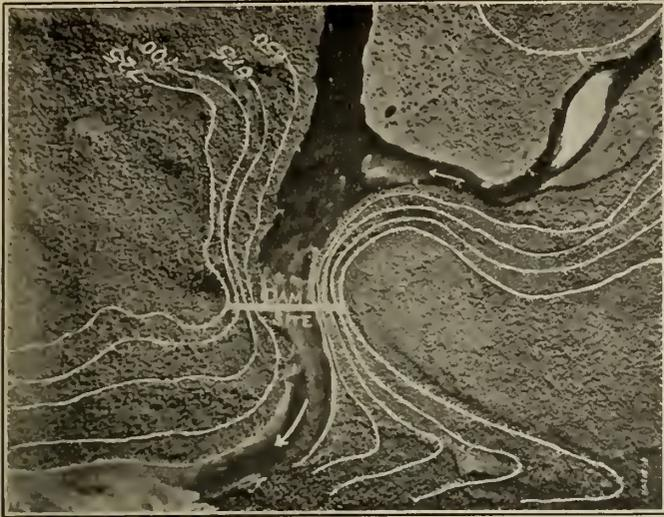
Figure No. 3.—Specimen of Individual Photograph with Stereoscopic Form Lines.
