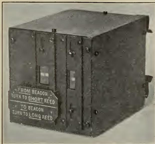
Figure No. 24.—Visual Indicator with Third Reed for Marker Beacon Transmitter.
