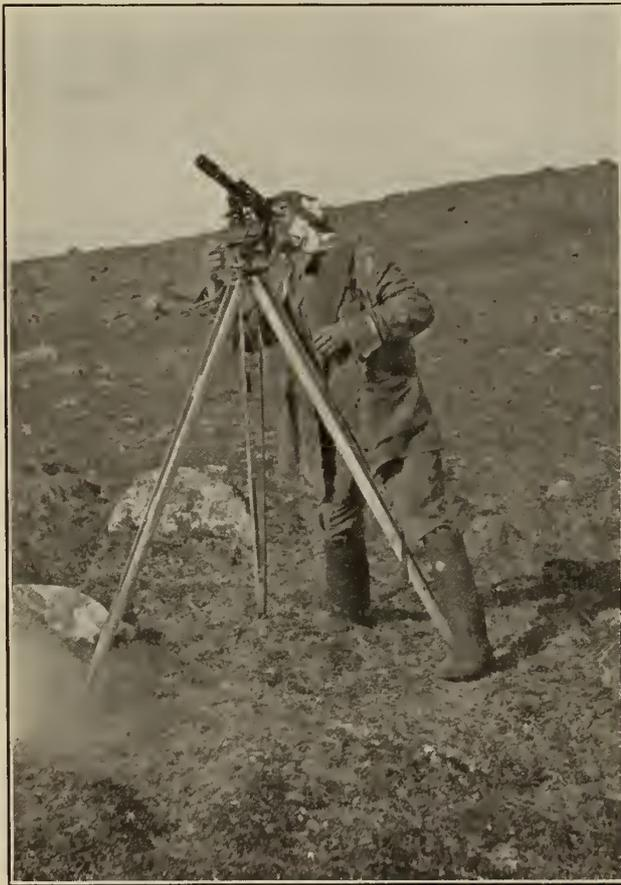
Figure No. 9.—Solar Observation for Watch Correction.
