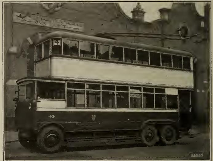
Figure No. 6.—Six-wheeled Double-deck Trolley Bus at Wolverhampton, England, 1926.
