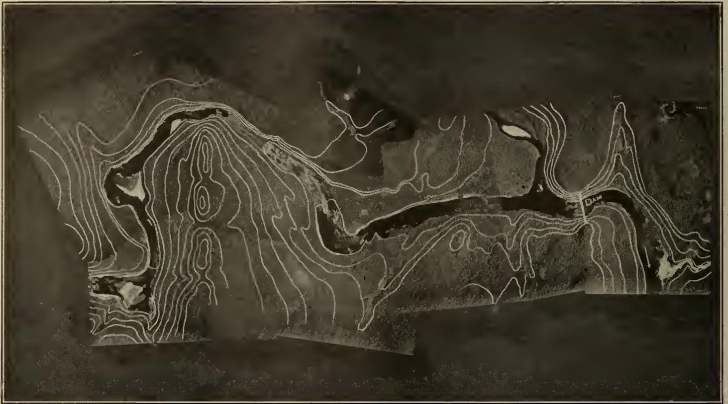
Figure No. 2.—Specimen of Mosaic of River showing Stereoscopic Form Lines.
