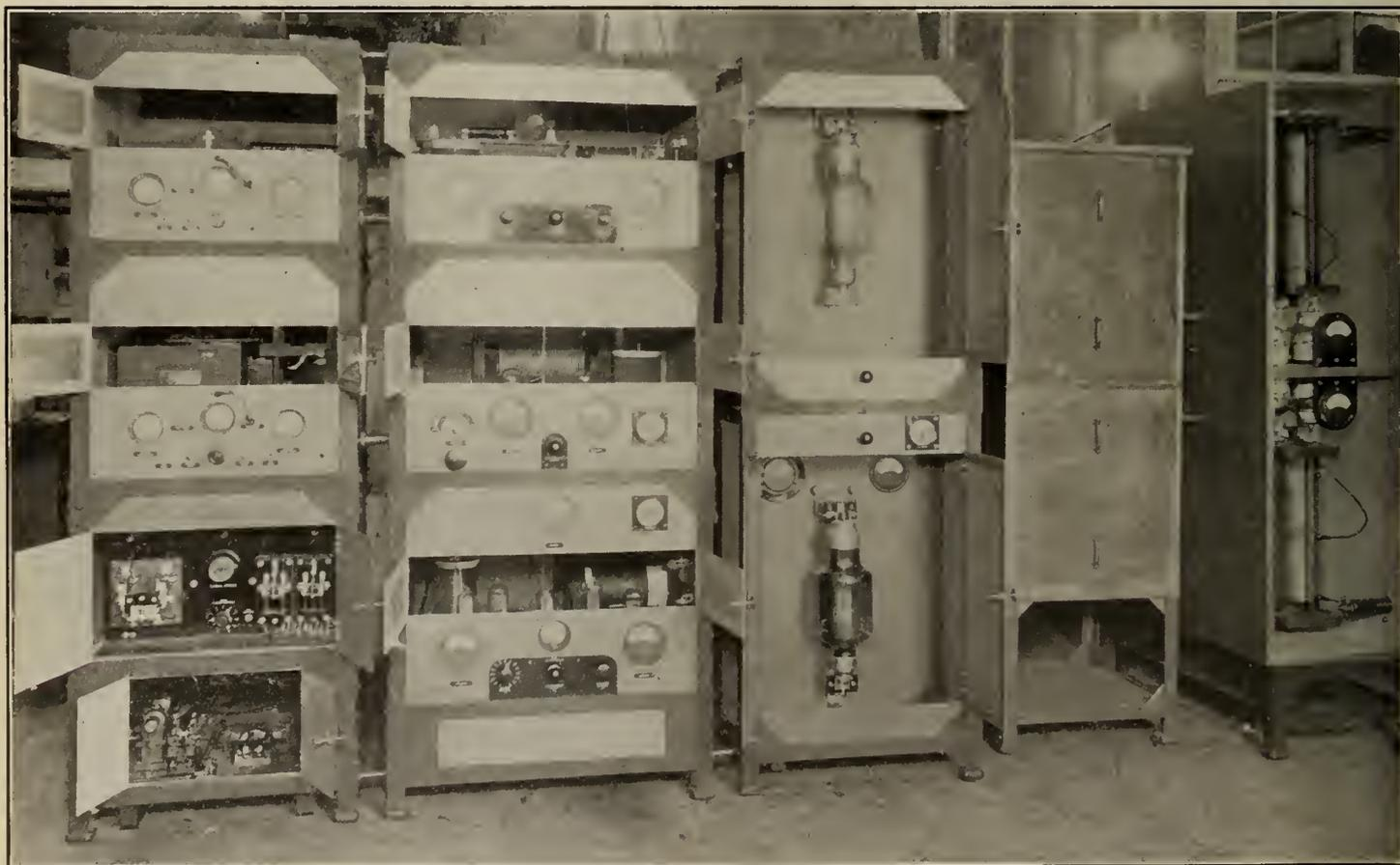
Figure No. 22.—Canadian Radio Beacon Transmitter—Front View, on Left is Tuning Fork and A and N Drive—on Right is the Loop Tuning Apparatus.
