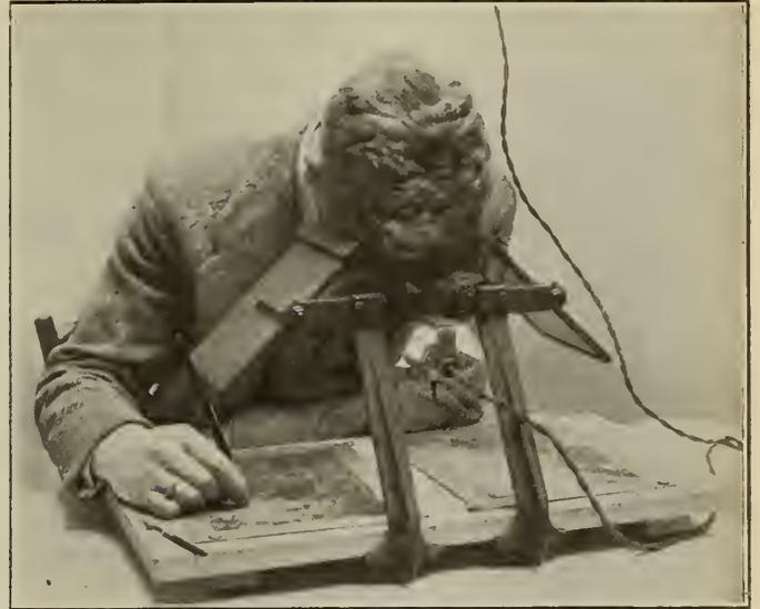
Figure No. 4.—Aerial Stereoscope in Use.
