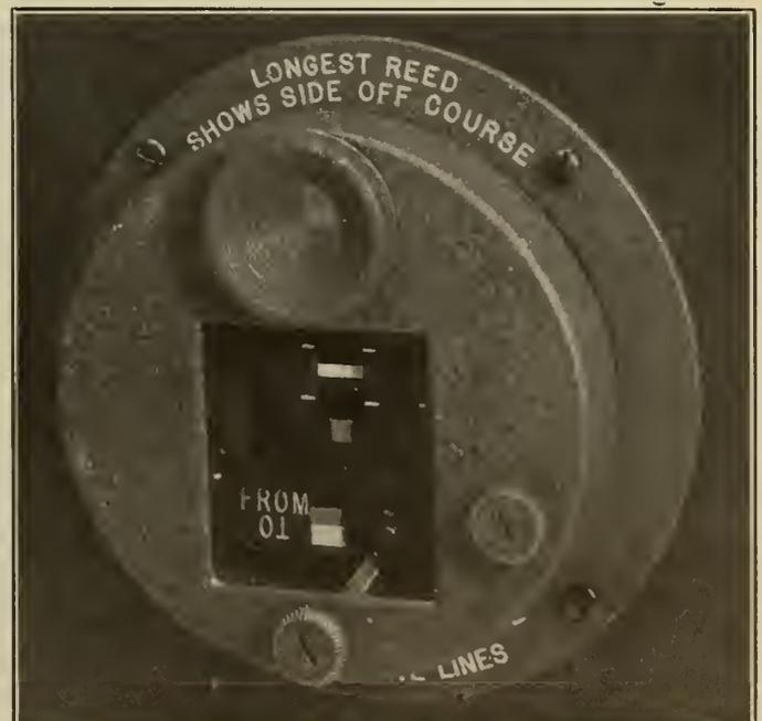
Figure No. 25.—Visual Indicator of the Vibrating Reed Type, developed by Bureau of Standards, Washington, D.C. for Use in Aircraft.
