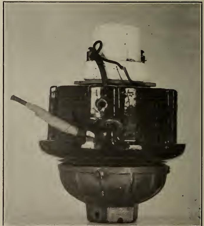
Figure No. 2—Street Light Fixture Causing Interference.
