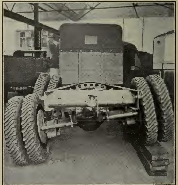
Figure No. 4.—View showing Extent of Flexibility of Rear Suspension without affecting Level of the Chassis Frame.
