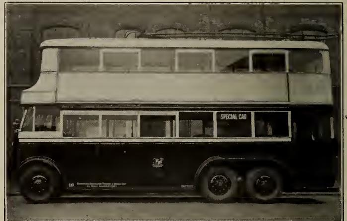
Figure No. 15.—Latest type Double-deck Trolley Bus supplied to Birmingham by Guy Motors, Ltd.
