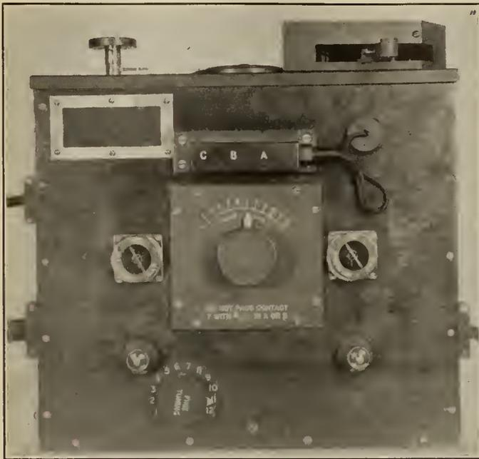
Figure No. 8.—Wavelength Control Panel of CT21 Aircraft Transmitter.
