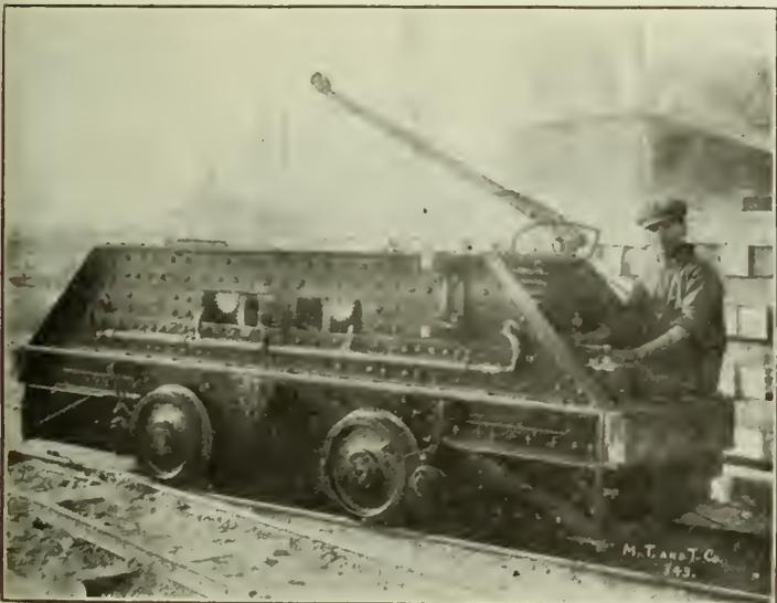
Fig. 23. Eight ton Construction Locomotive.
