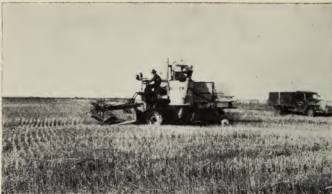
FIG. 27.—Self-propelled combine cutting wheat on the parklands near Berwyn.
