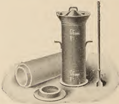
Moulds for Making Concrete Drain Tile
