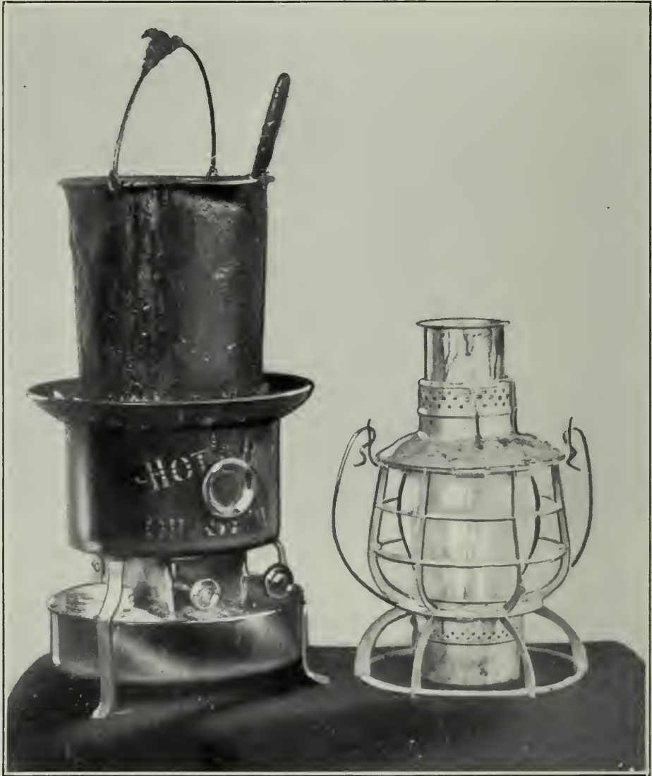
Fig. 25—Wax Heaters. Left—cheap, efficient equipment to be carried in a box. Right—Merribrooke Melter.
