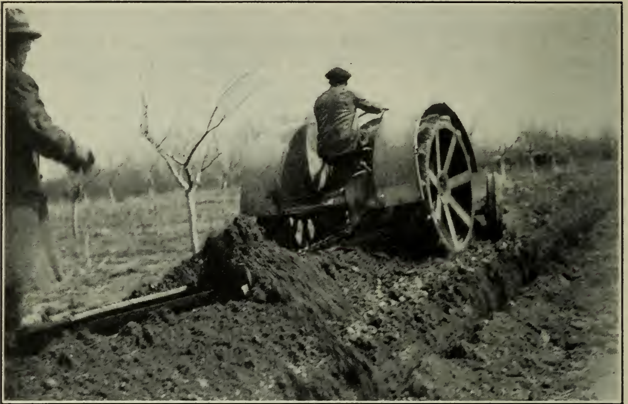
Fig. 9.—Martin ditcher used for backfilling. This is particularly well adapted to fruit orchards where the tree rows are narrow.
