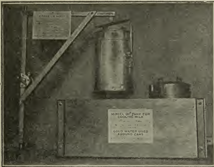
TANK FOR COOLING MILK AND HOISTING APPARATUS.
