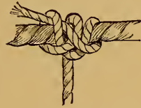
FIG. 25.—TO TIE A SHORT LINE, TO WHICH A HOOK IS ATTACHED, TO A LONGER OR GROUND LINE.
