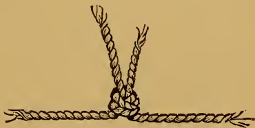
FIG. 2. — THE WRONG WAY.
