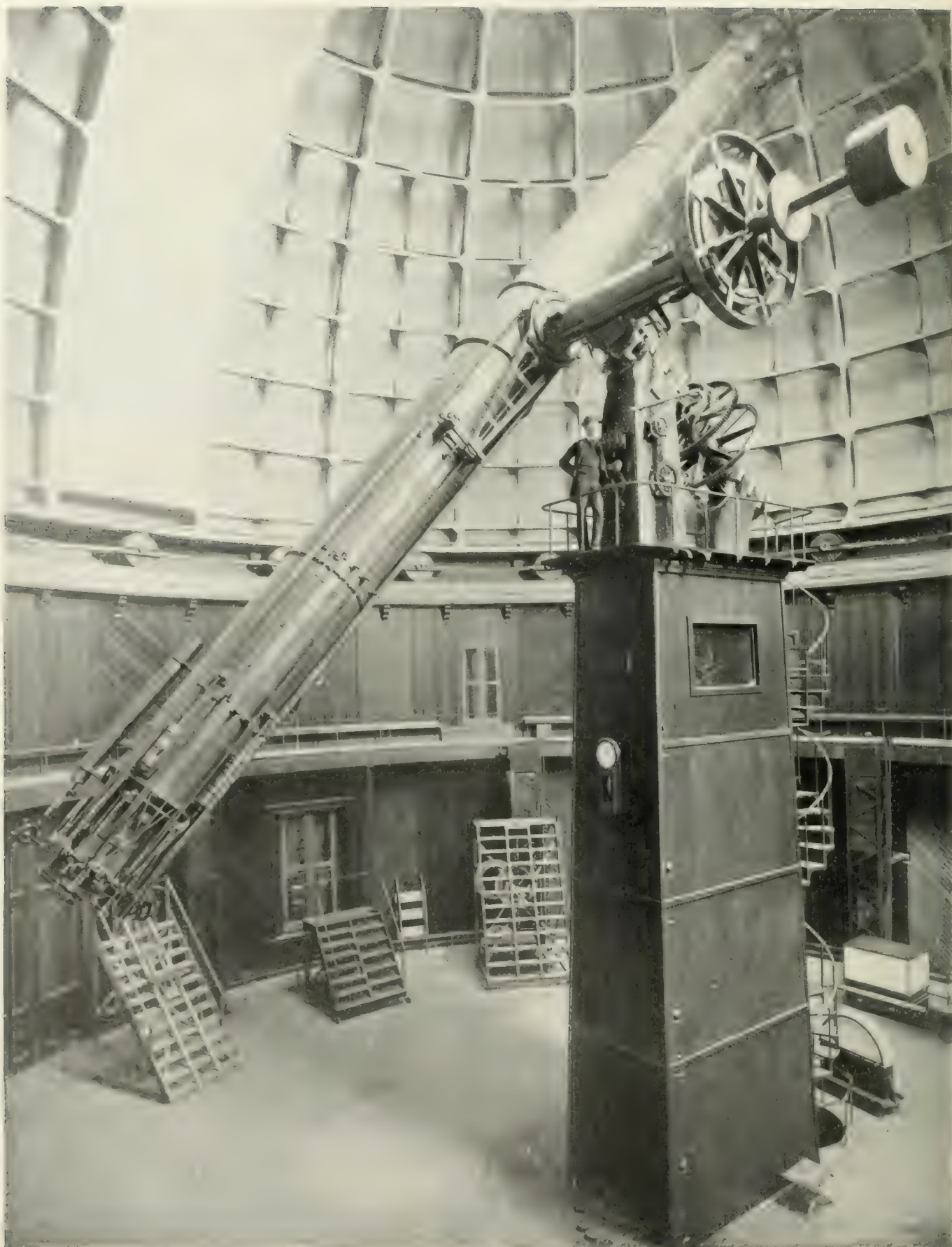
THE FAMOUS 36-INCH REFRACTOR OF THE LICK OBSERVATORY
