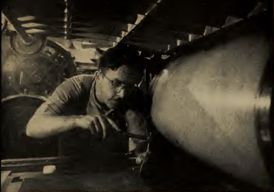
*Last careful adjustments are made to the form before new Miller automatic press is started*
