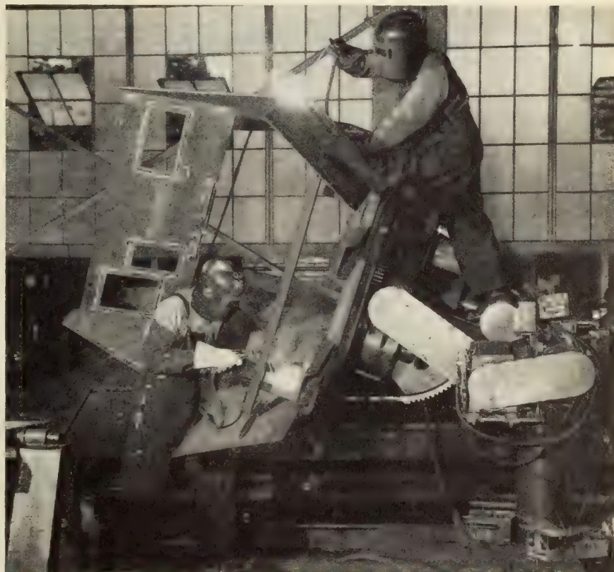
Fig. 6—Large motor-operated positioner for handling major hull assemblies.
