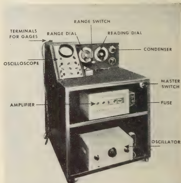
Fig. 4—Dynamic strain recorder used at the Bureau of Mines' physical metallurgy research laboratories.
