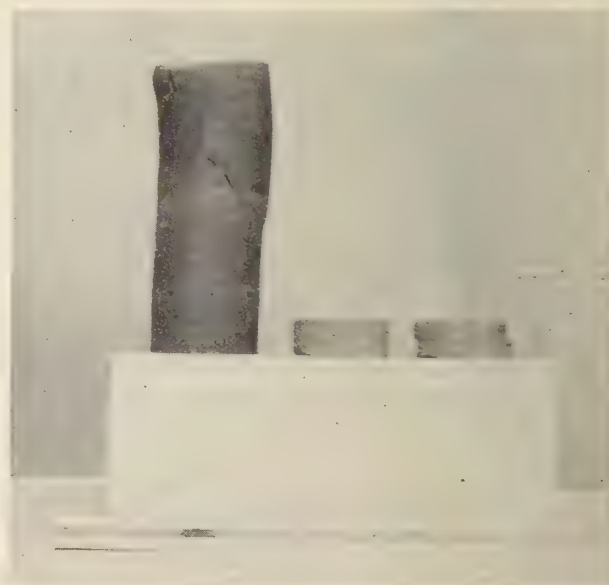
Fig. 10—Soil specimens showing shear planes.
