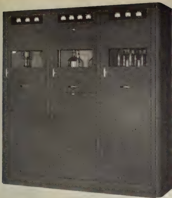
Fig. 2—Collins high powered, 10 channel, crystal controlled ground station transmitter used at several Trans-Canada Air Line Maritime stations.
