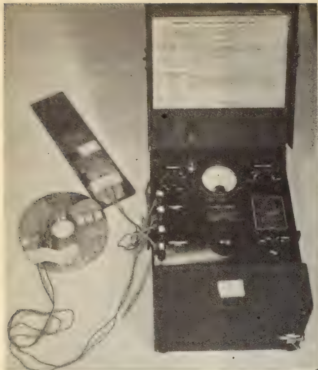
Fig. 3—Testing a Belleville spring at the Bureau of Mines' physical metallurgy research laboratories, using SR-4 strain gauges and strain indicator.
