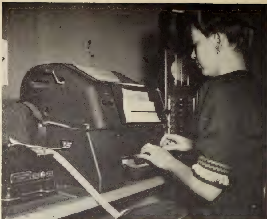
Fig. 9—Model 19 semi-automatic teletype equipment used by Trans-Canada Air Lines.
