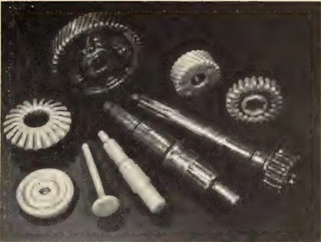
(The Dow Chemical Company) For protection against corrosion the parts shown above have been packaged in stripecoat and are ready for shipment.
