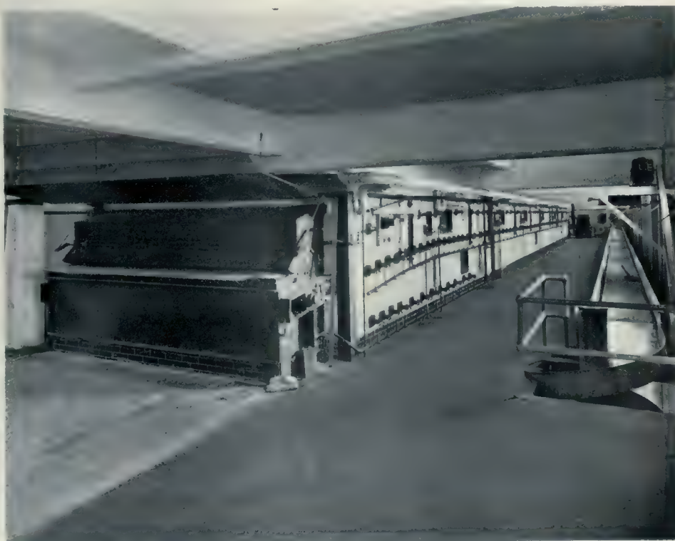
TRAVELLING OVEN, SECOND FLOOR, SHOWING BREAD CONVEYOR.
