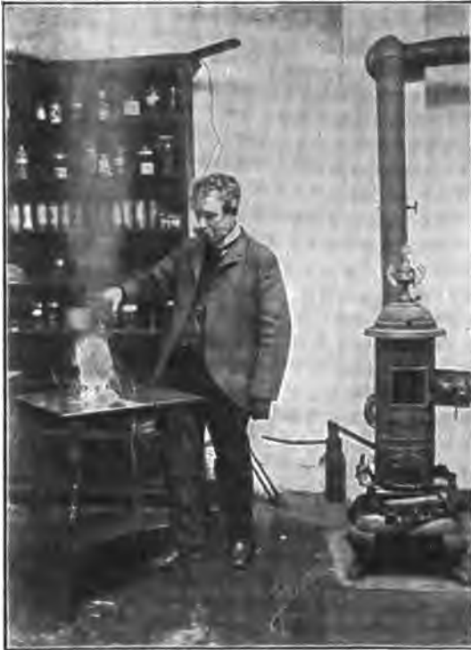
Mr. Maxim pouring molten cast iron on a quantity of Maximite without producing an explosion.
