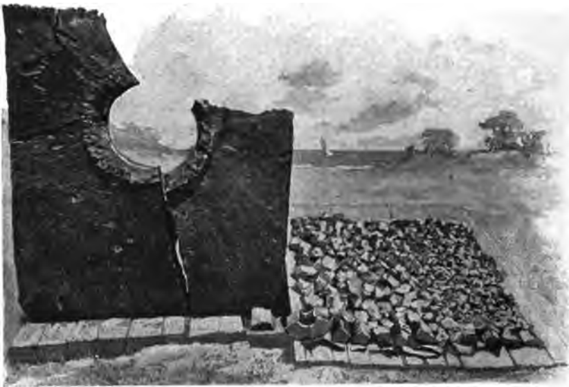
Fragments of a 5\frac{1}{4} -inch plate, readjusted in position, after explosion in the plate of a Maximite shell, together with the recovered fragments of the shell at the right.
