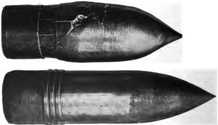
Two six-pounder A. P. shells, one showing the shell in its normal shape, the other a shell which was filled with Maximite and fired at a 3-inch plate, entering about half its length, upsetting, as shown, until it broke open at the side, some of the Maximite being forced through the aperture. This shell rebounded from the plate about 200 feet and struck in front of the gun from which it was fired, all without exploding. This was a test for insensitiveness, the shell carrying no fuse.
