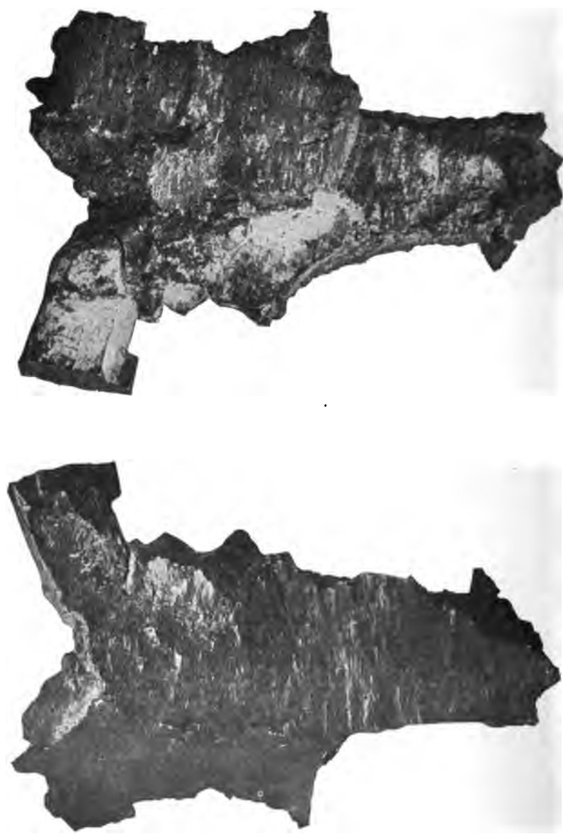
Two views of a fragment of a shell exploded with Maximite. On the left of the first fragment, which was the inner surface of the shell, is seen the flattening and stretching effect of the blow which was received from the explosion, as though it had been heated and then struck with a sledge hammer, the force of the blow being so sudden and severe that the whole outer surface of the shell, except a small piece seen hanging to the fragment on the right, was knocked off by the force of the impact. On the right is an opposite view of the same fragment, showing where the piece was jammed upon a neighboring fragment with such force that its surface was made to flow like wax.
