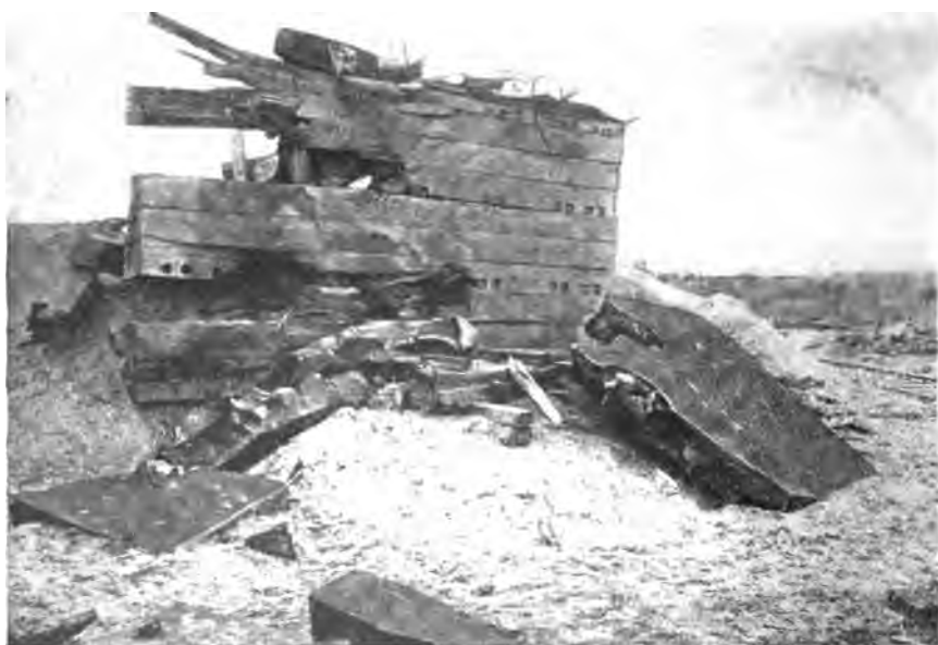
Wreck of 30-ton plate and sand crib by 12-inch armor-piercing shot, charged with 23 pounds of Maximite.
