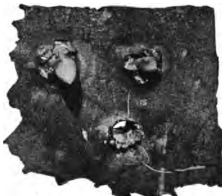
Points of unexploded 6-pounder Maximite shells, left sticking through a 3-inch plate, in a test for insensitiveness.
