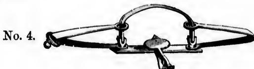
No. 4 is called the BEAVER TRAP. The jaws spread six inches and a half. It is adapted to the wolf or the lynx.—Extra sets of jaws with teeth constructed expressly for taking deer, are made to fit this trap, and can be had separately, or may be inserted in the place of the ordinary jaws.
