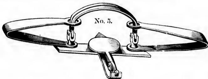
No. 5 is called the SMALL BEAR TRAP. The jaws spread eleven inches and three-fourths. The weight of each spring is two pounds and ten ounces, and the weight of the whole trap is seventeen pounds. It is adapted to the common black bear, the panther, and most of the large animals found this side of the Rocky Mountains.
