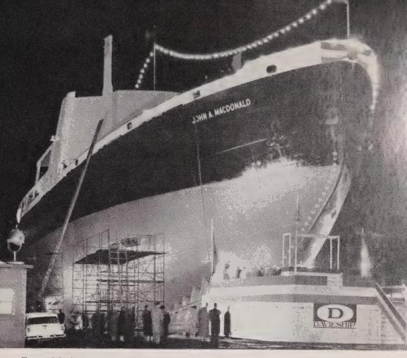
The world's third strongest 15,000-hp. ice-breaker, the John A. Macdonald, completed its maiden northern supply tour in 1960. It is scheduled to make a crossing of the Northwest Passage in 1961. This ship has a radius of action of 20,000 miles without refuelling and is fitted with triple propellers, three helicopters for reconnaissance, an electric fire detection system, an electrically heated crowsnest, and a hull capable of withstanding heavy ice pressure.
