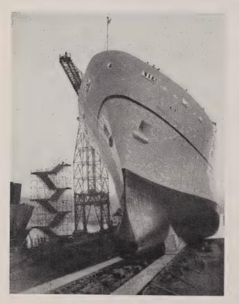
Canadian Pacific Steamships' new flagship, the Empress of Canada, minutes before she was launched in May, 1960. Put into operation on the Atlantic run in April, 1961, this 27,500-ton ship is featured by a bulbous bow designed to reduce pitching and stabilizers to cut roll from  $25^{\circ}$  to  $3^{\circ}$ .
