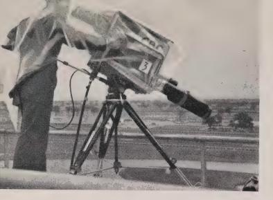
A CBC technician and a camera share the latest in transparent rainwear—a plastic hood designed to protect man and machine from bad weather during telecasting of outdoor events. Nearly 1,000 skilled technicians maintain and operate cameras and other electronic equipment in CBC's 18 production centres across Canada and hundreds are employed in private television stations.
