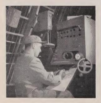
Meteorological research is important in transport, communications, agriculture and other fields. In the dome of the weather station building at Maniwaki, Quebec, a technician tracks down a balloon and radiosonde transmitter by radio direction finder, thus recording direction and velocity of the wind at upper air levels.
