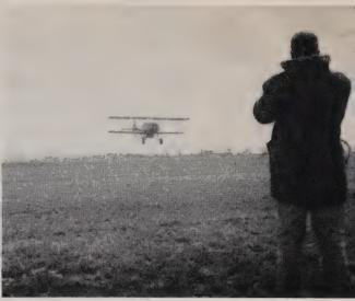
A new use for aircraft: spreading of dry fertilizer. A plane can cover about 600 acres per day. Planes are used extensively by farmers for supervision of farms and spraying of crops.
