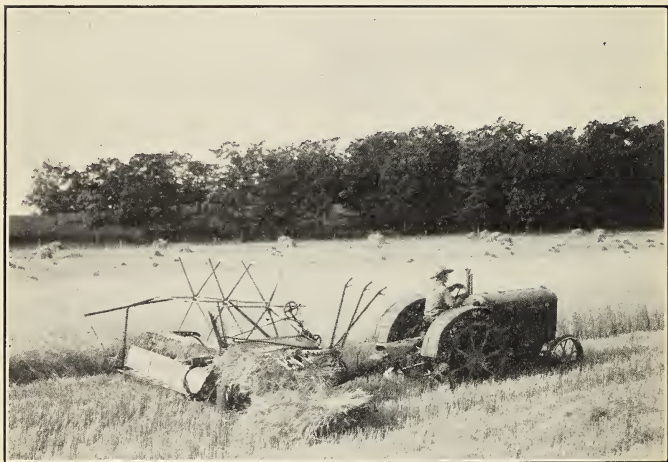
Fig. 140. Tractor-Binder. The power take-off is right behind, and underneath, the driver.
