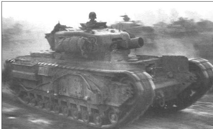
The Churchill AVRE was used to destroy enemy strongholds, and to protect and transport demolition teams.
