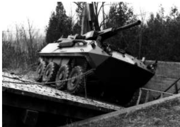
Equipment testing at LETE. A Bison AVGP with experimental gun mount on the tilt-table. DND.
