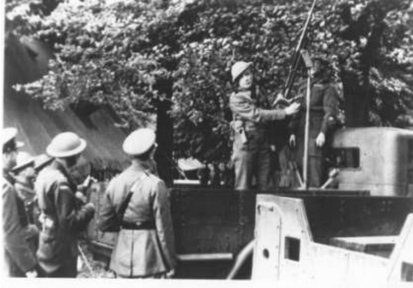
First Line of Defence - summer 1940. After Dunkirk to meet the needs of light low-level air defence in Southern England, 2 Army Field Workshop designed and built several hundred high-angle machine gun mounts for installing on light vehicles. Major G.W. Beecroft demonstrates one for the Duke of Gloucester in Ladas Park, Kent. The late Col G.W. Beecroft.
