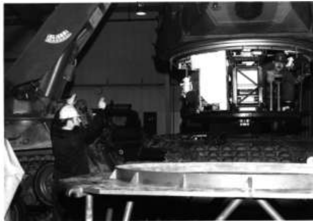
Tank overhaul at 202 Workshop Depot. Replacing a Leopard tank turret. DND.
