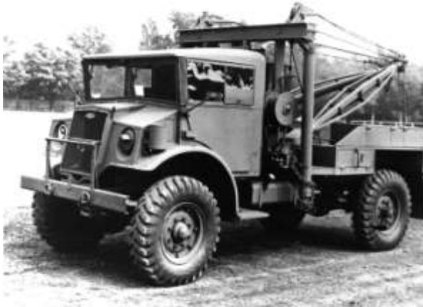
Left: 60-cwt CMP Wrecker - 1940s-1950s. General Motors/Ford 3-ton 4x4, Garwood (later Holmes) twin boom wrecker gear, powered winch. Dr. W.A. Gregg
