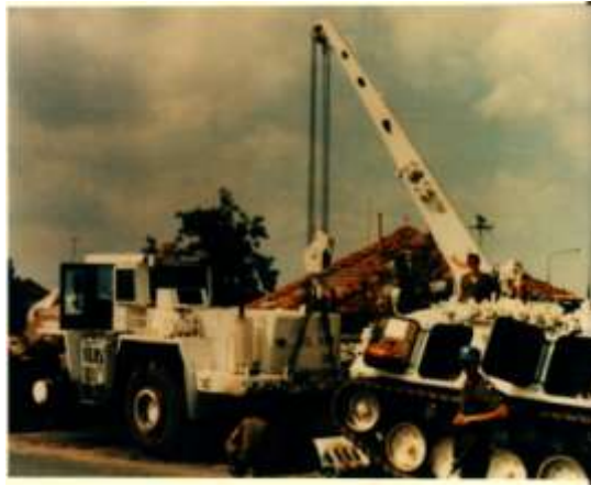
Heavy equipment recovery - UNPROFOR. Zettelmeyer being lifted by a Leopard ARV (Krauss-Maffei improved) with 20-ton rotating boom, 35-ton winch and rear-deck which can carry complete tank power pack. M/Cpl B. Graham.
