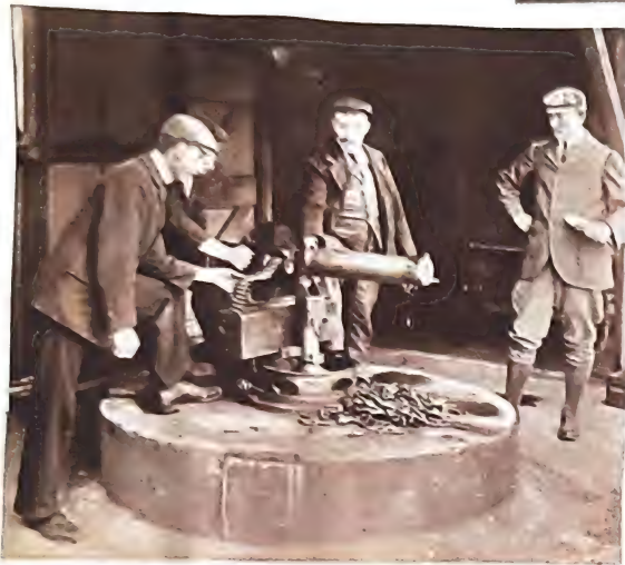
FIRING ROUNDS AT CLOSE RANGE, INTO A BANK OF SAND TESTING THE MECHANISM OF A MAXIM ON A PERMANENT MOUNT
