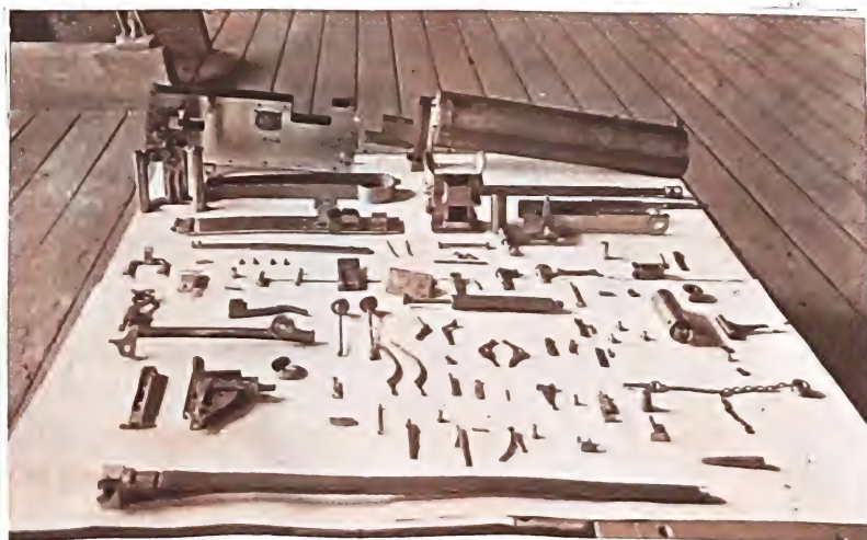
USED FOR REFERENCE: PARTS OF A MAXIM—ALL OF THEM SPECIALLY FINISHED—EMPLOYED AS STANDARDS.
