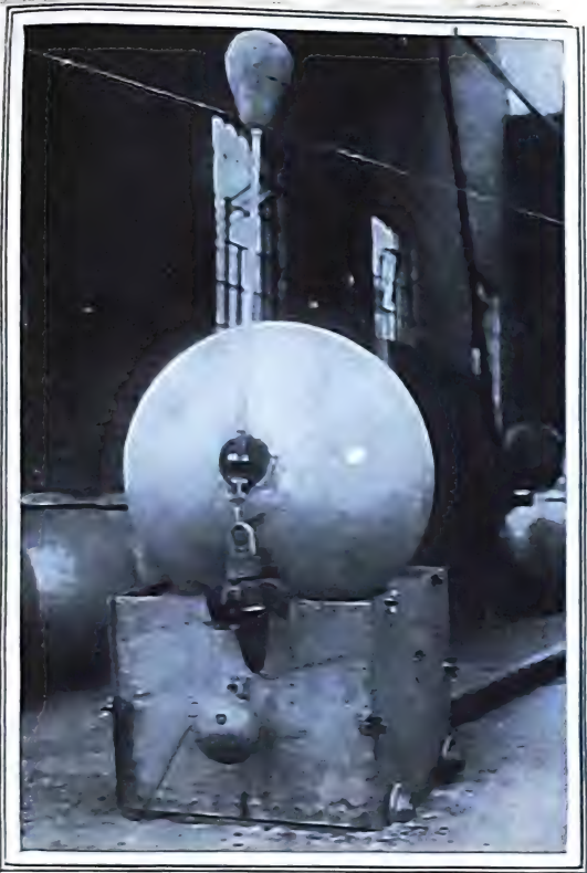
THE SPHERICAL FORM OF SUBMARINE MINE: ONE OF THE LATEST TYPES OF FLOATING MINES USED FOR BLOWING-UP SHIPS AT SEA.
