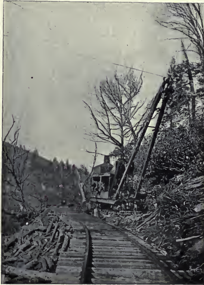
Clyde Overhead Skidder, showing logs being piled below the railway track,—Townsend, Tennessee.
