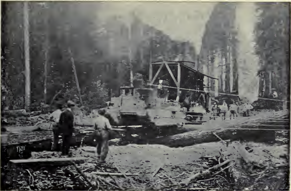
(1). Skidder mounted on timber skids hauling itself sideways off a railway car at a new setting ; New Westminster, B. C.
