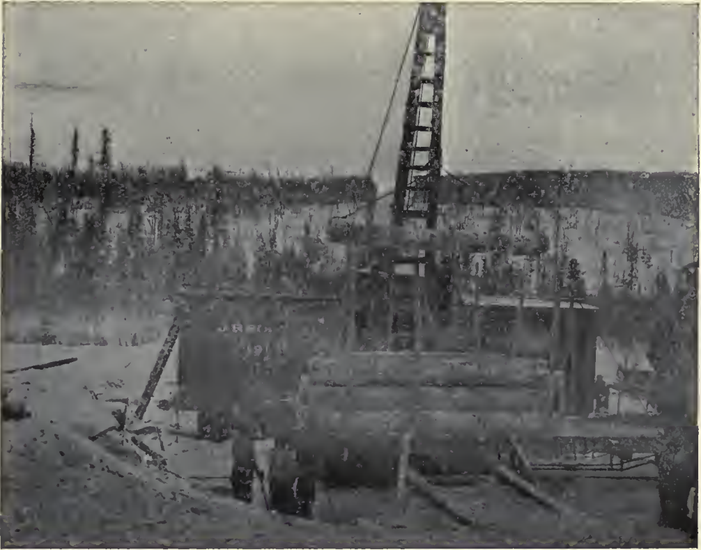
(1). Fixed Boom machine mounted on car, loading pulp wood ; double track;— Madawaska, Ontario.
