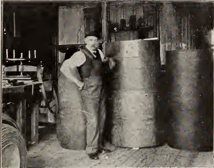
Cut of 50-inch "Extra" Double Belt Made by The J. C. McLaren Belting Co., Limited.
