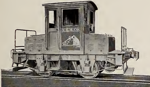
15-Ton Baldwin-Westinghouse Storage-Battery Locomotive with Pedestal and Channel Frame.
