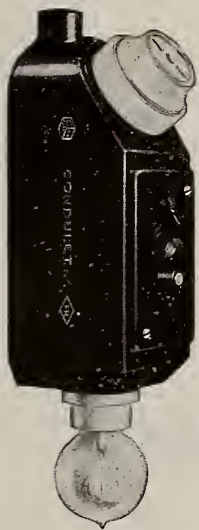
Type FH Condulet Showing Surface Plug Receptacle, Double Push Button Switch, Cover DS8, Receptacle C337 and Incandescent Lamp Mounted.
