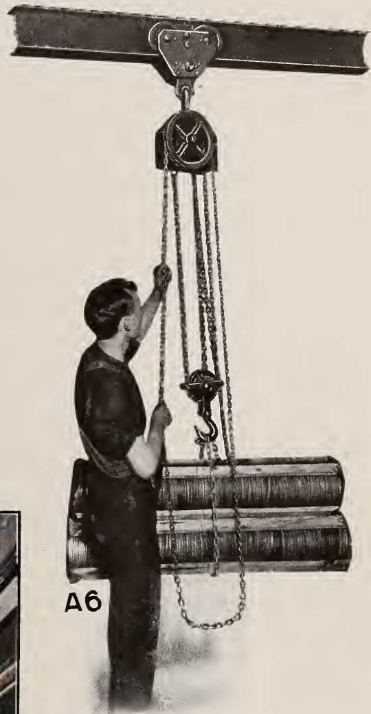
Standard Beath Trolley, Type A. with Chain Block on an Overhead Runway System with Switches and Curves, is a wonderful money saver in lifting and moving goods.
