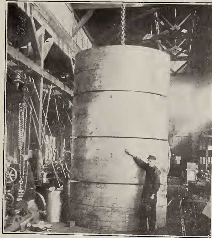
Stock of Rubber-Covered Head Pulleys for C. P. R. Million Bushel Elevator at Victoria Harbor, and Manufactured by the Dodge Manufacturing Co., Toronto.
