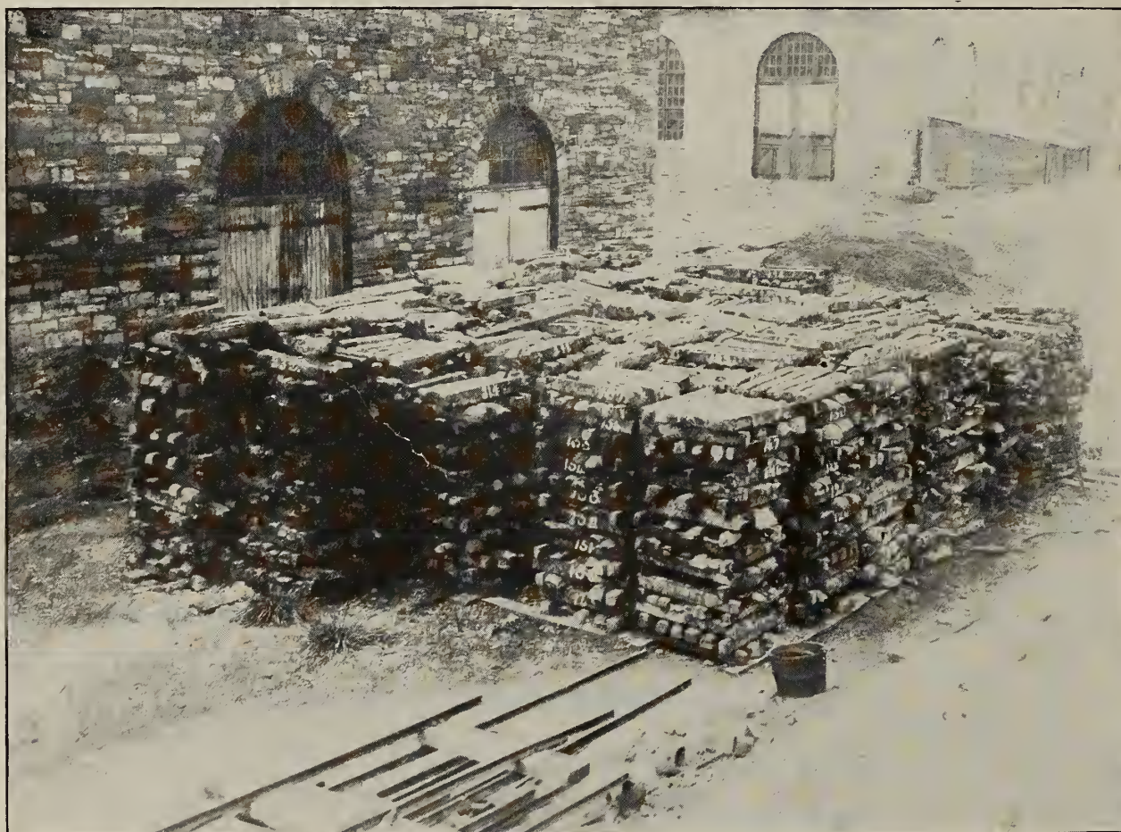
165 Tons of Nickel Pig, Produced from the Electric Furnace at Sault Ste. Marie, Ont.
