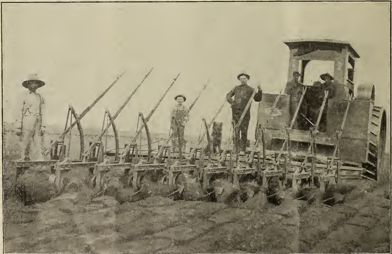
A ten furrow steam plow, built by the Cockshutt Plow Co. doing the work of several men.
