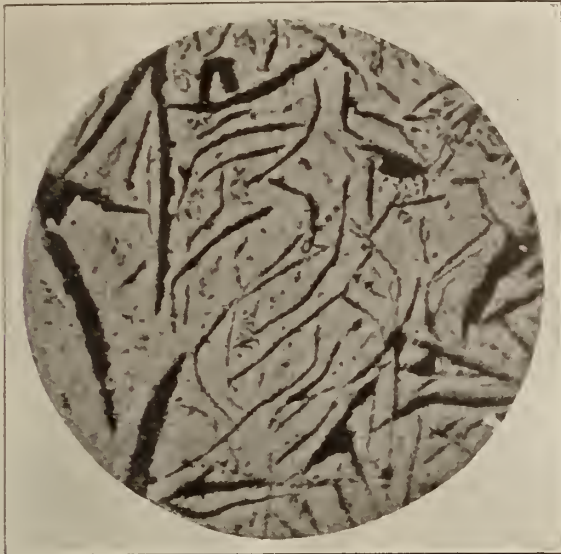
Fig. 2—Photo-micrograph taken under a magnification of 750 diameters. The dark portions represent the plates of graphite interspersed through the metallic iron
