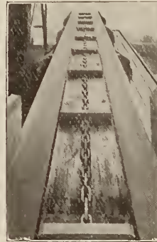
Ceiling Chain Refuse Conveyer
