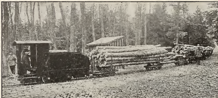
Fig. 1.—An Alcohol Locomotive in German Forestry Service near Darmstadt.
