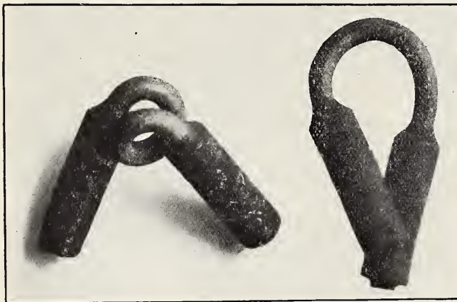
Plate 1. Bending of \frac{1}{2} -inch Round Test Bars.
