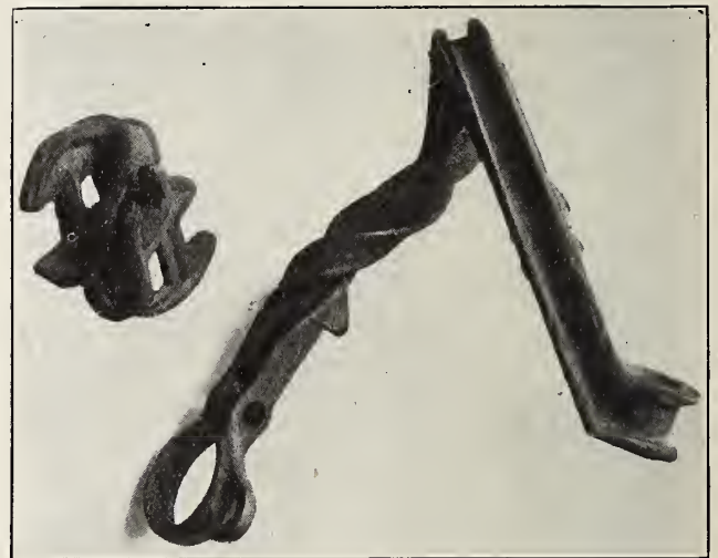
Plate 2. Illustrating Malleability of Finished Castings.
