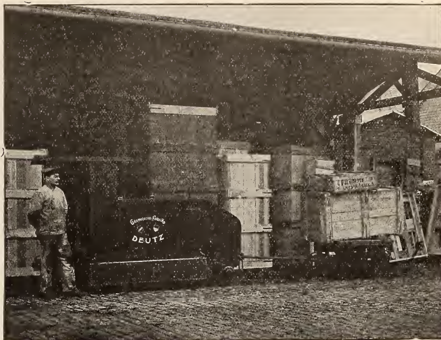
Fig. 3.—A 6 H.P. Alcohol Locomotive, built by the Gasmotoren Fabrik, Deutz, near Cologne, Germany, Hauling Miscellaneous Merchandise on a Factory Railway.
