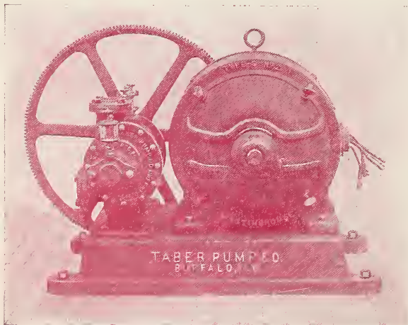
Westinghouse Type S Motor Driving Taber Pump
