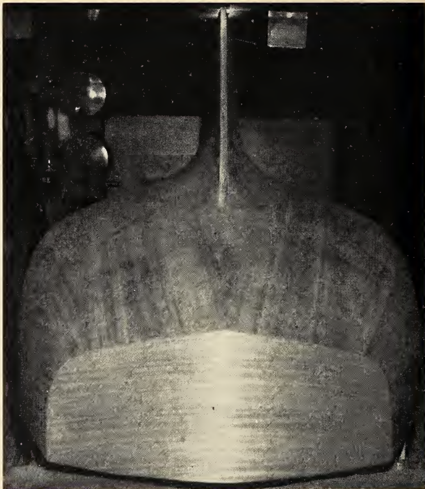
Figure 7. Stern View of Hull Plug. The flowing curves of this 35 ft. sailboat are readily molded in plastic.
