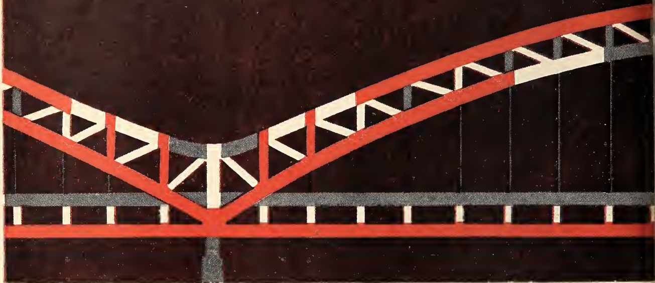
Sketch of one span of the two-span bridge showing where it was most efficient to take advantage of the high yield strength provided by steels such as "T-1" Steel (in red), USS TRI-TEN High-Strength Low-Alloy Steel (in white), A7 and A373 Structural Carbon Steel (in gray). Louisville-New Albany Bridge
