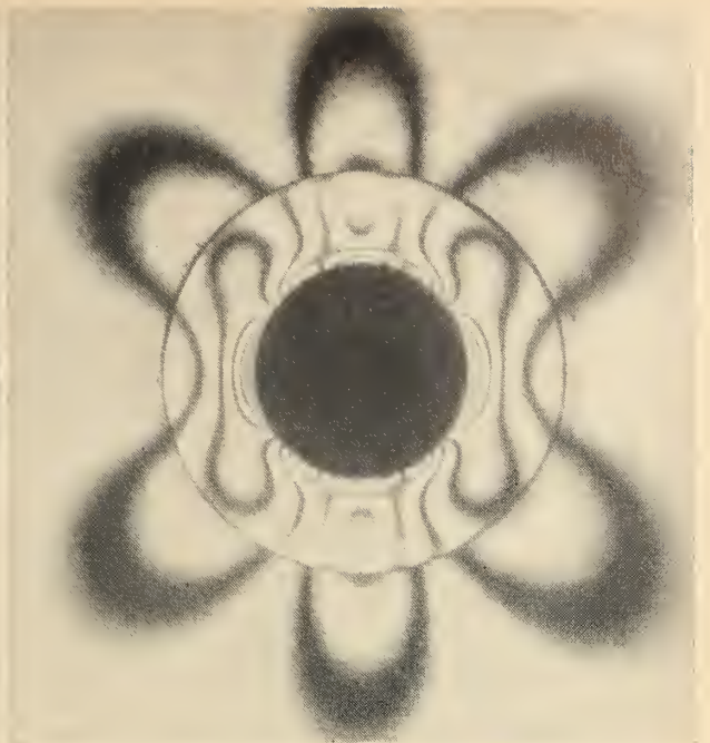
Fig. 6. Frozen Stress Pattern of Reinforced Circular Hole in a Plate under Tension.
