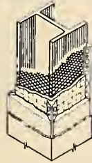
Vertical columns are fireproofed and finished with gypsum plaster over self furring metal lath. Recesses between column webs provide excellent ducts for service pipes.
