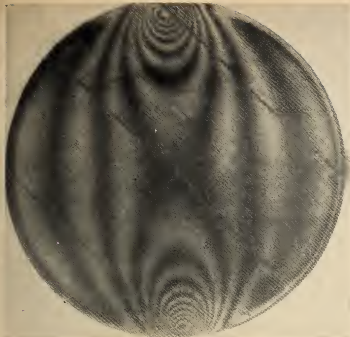
Fig. 5. Frozen Stress Pattern of Diametrically Loaded Laminated Disc.
