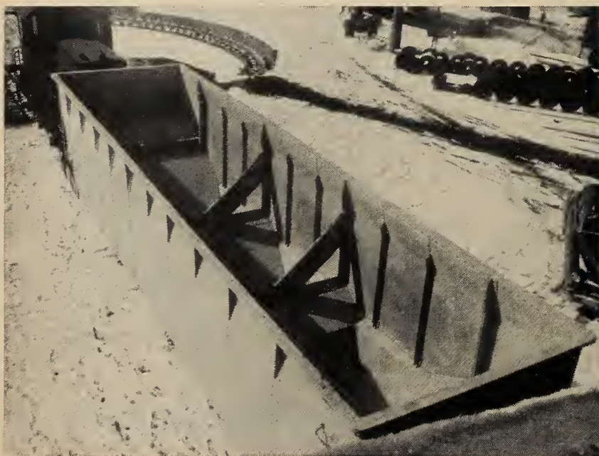
Fig. 1. Inside View of 70-ton Open Hopper Car with Aluminum Body. 30 cars of this type were built in 1948, 50 in 1949 and 10 in 1951 for the R.&S.
