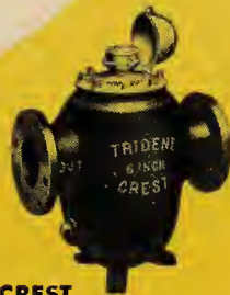
CREST Velocity or inferential type, with turbine or propeller, for high rates of flow. Sizes 1\frac{1}{2} " and 2" screw end. 1\frac{1}{2} " to 16" flange end.
