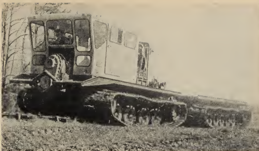
Fig. 10. Musk-Ox 20 Ton Articulated Transporter.
