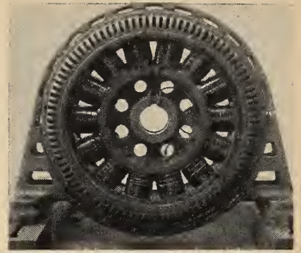
Fig. 6 Synchronous motor built in 1922 to drive a reciprocating compressor
