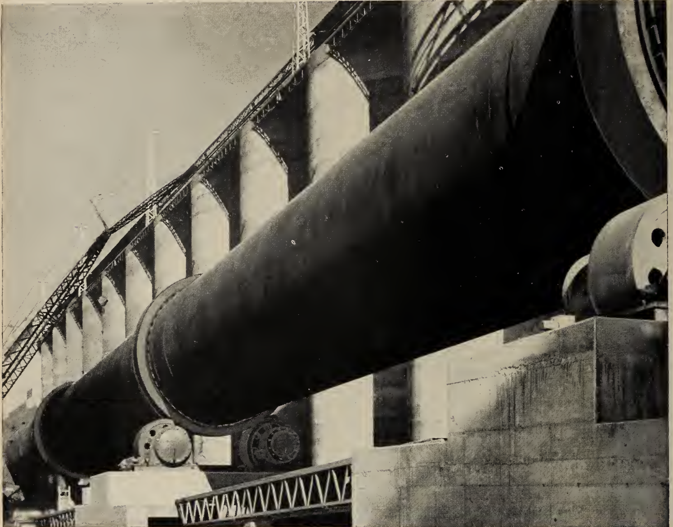
Section of heat transfer system for new cement plant, Miron et Frères, Montreal.
