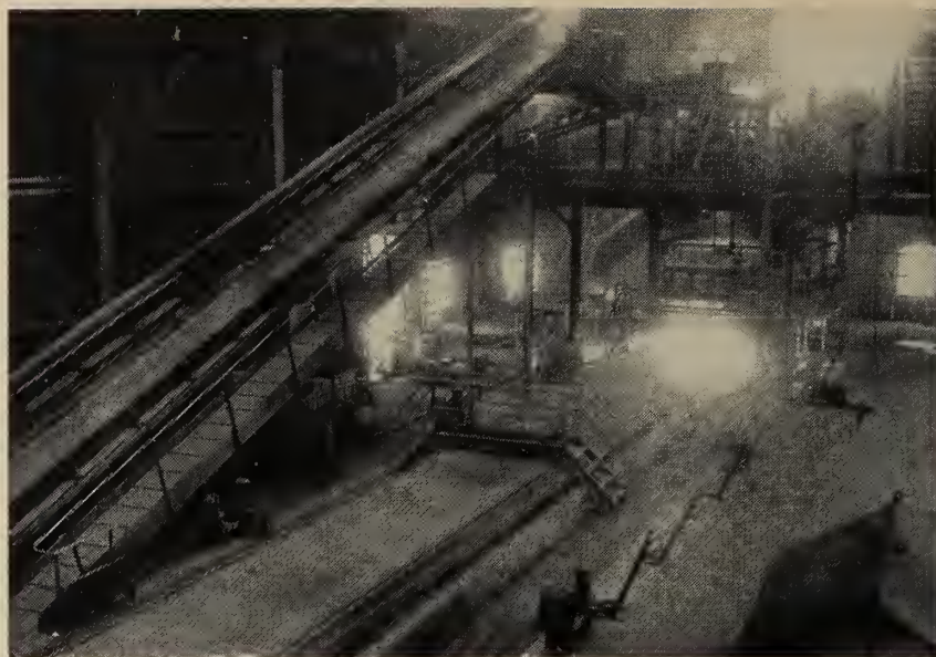
Fig. 4. View looking towards loading end of sinter strand. Conveyor elevating mixed material to head of strand at left.
