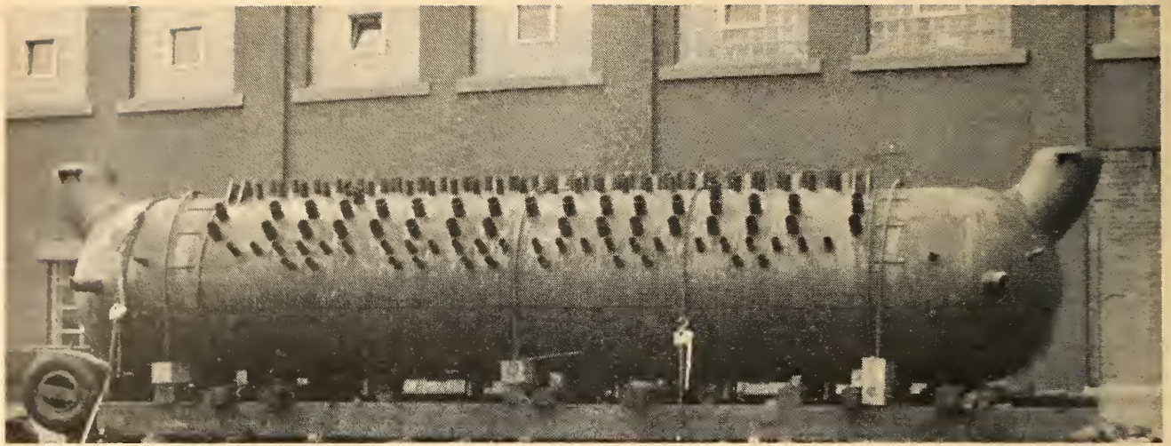
Fig. 7. A view of Steam Drum showing stub tubes projecting.
