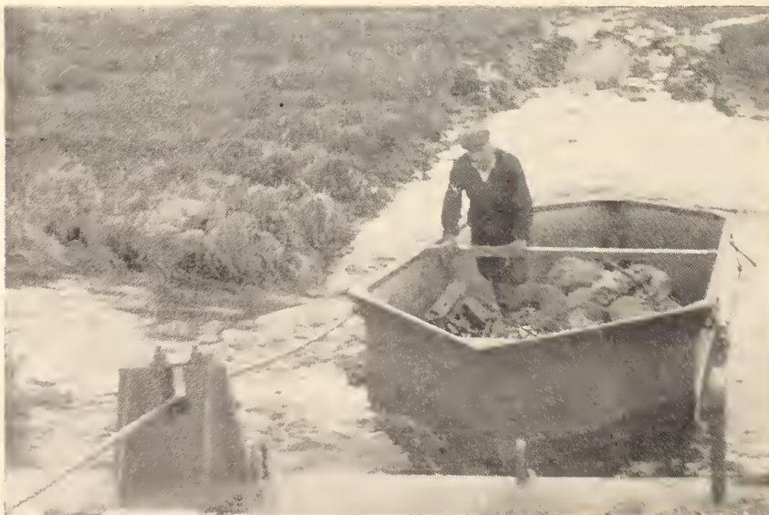
Fig. 5. Here, a non-powered slipe is being drawn behind a powered unit: loads of up to ten tons can be hauled in these slipe.
