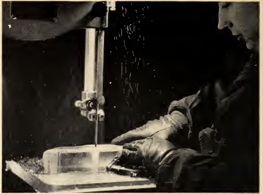
Preparing samples for testing of the physical properties of ice, in the snow and ice laboratory of the Division of Building Research.
