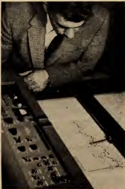
Fig. 11. The Electro Dataplotter for plotting of profiles and cross sections from punched tape or punched cards.
