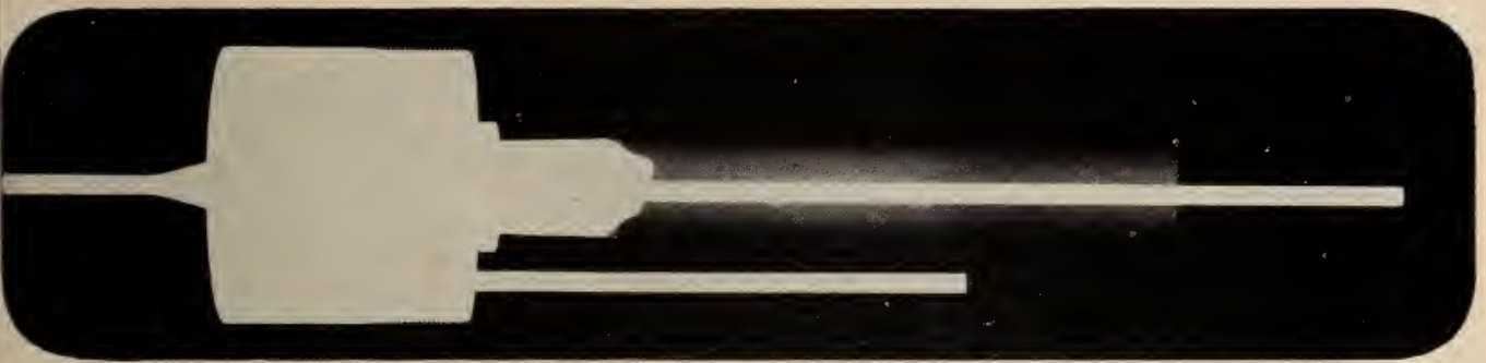
Radiography reveals no foreign particles or voids in molded areas, shows the ultimate contact of the molded insulation with seal to the central conductor.
