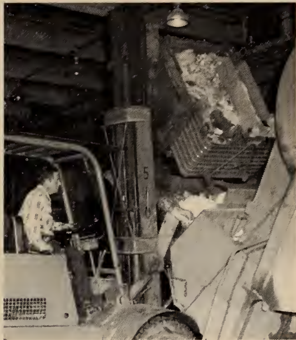
Fig. 10 Fork lift truck with swivelling head attachment about to dump contents of special waste-bin into garbage truck.
