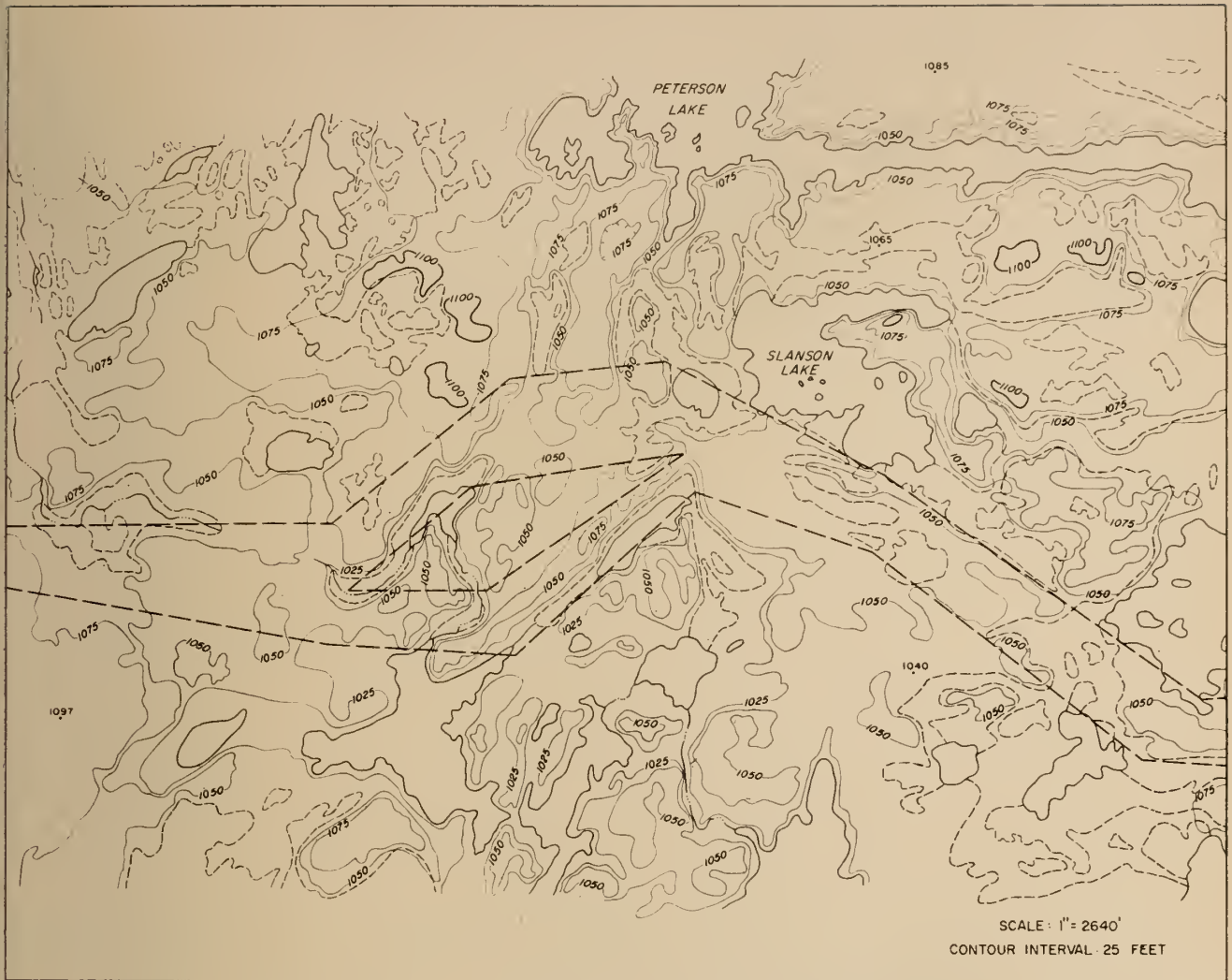
Fig. 2. The outlined strip on this reconnaissance map has been chosen to be re-photographed as the selected route. The new photograph will be used for detailed photo analysis and the preparation of accurate topographic plans (32.5% reduction from original drawing).
