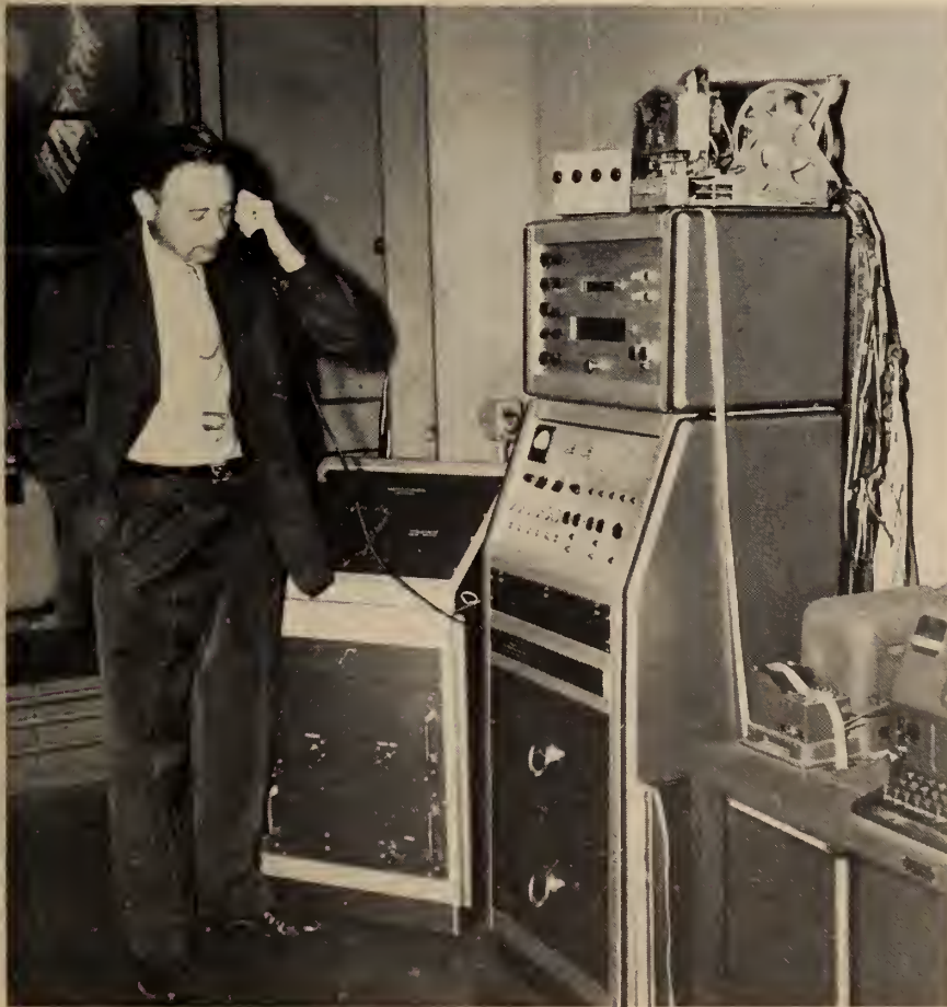
Fig. 14. Equipment for digital printout, programming, and teletype transmission to electronic computer.
