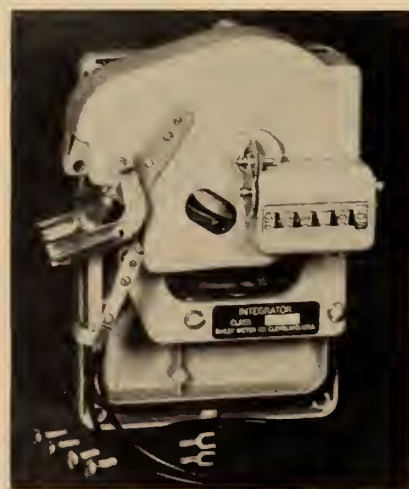
Fig. 9. Pneumatic and electronic receiving elements and integrator.
