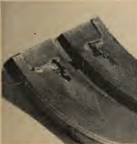
Fig. 16. A cavitated connecting rod bearing.
