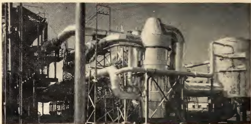
Converters containing a vanadium catalyst are part of C-I-L's sulphuric acid plant at the explosives works, Beloeil, Que.
