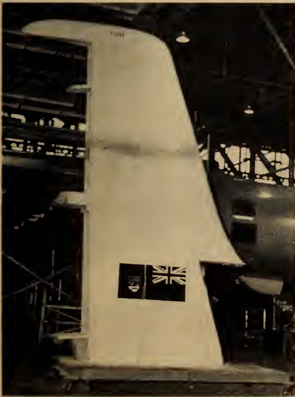
Fig. 6 Vertical stabilizer mounted on its special handling fixture.
