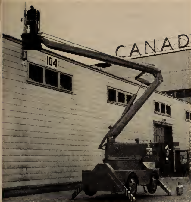
Fig. 9 Hydraulically-operated 'giraffe' hoist is now used to move men working on upper surfaces of aircraft. Two of these units are in use at Canadair plant.
