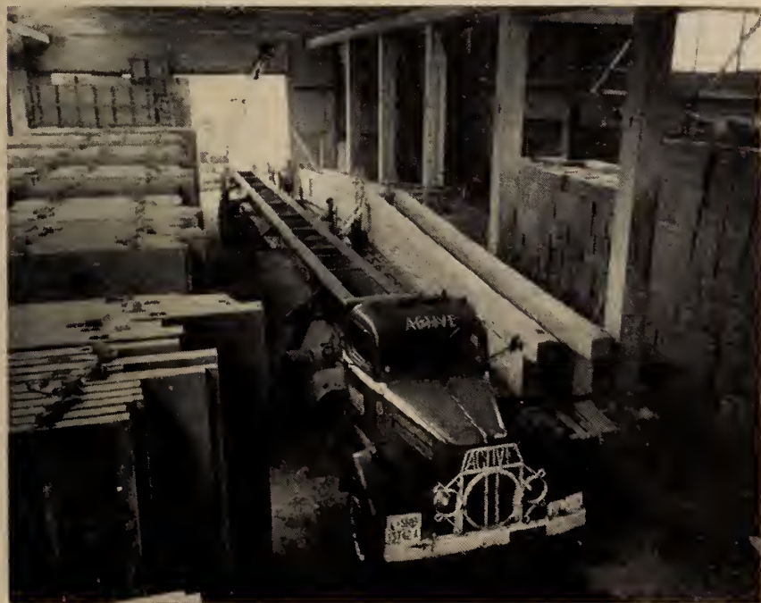
Fig. 5. Factory storage under cover avoids on-site storage problems in winter and allows complete curing in controlled conditions.
