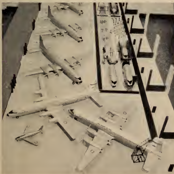
Fig. 1 Model table showing layout for CL-44 fuselage assembly shop (upper right), final line (upper left), and pre-flight area (foreground). The floor is marked in the equivalent of two-foot squares. Note the relative sizes of the CL-44 and the small Sabre (at left).
