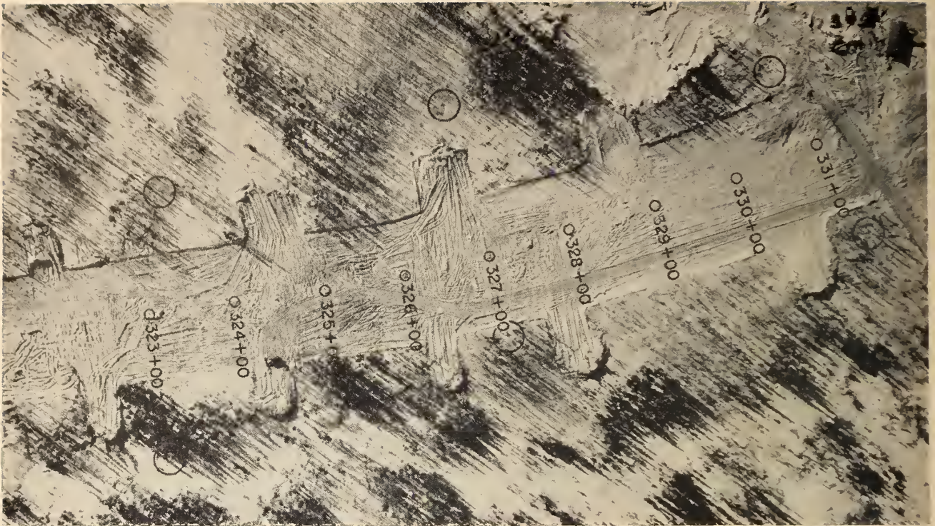
Fig. 12. Portion of an aerial photograph showing a cleared right-of-way. This was taken for the purpose of obtaining cross-sections and quantities of photogrammetric methods. The large circles indicate the location of permanent control points. The small circles show the location of flags placed on the centre line stakes.
