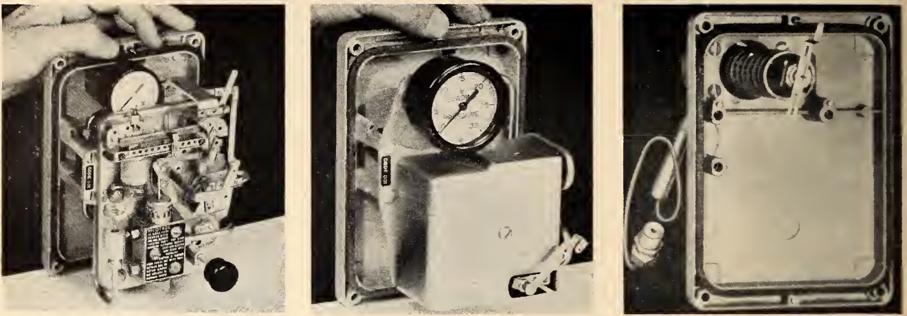
Fig. 10. Pneumatic transmitter, pneumatic controller, and pressure element.
