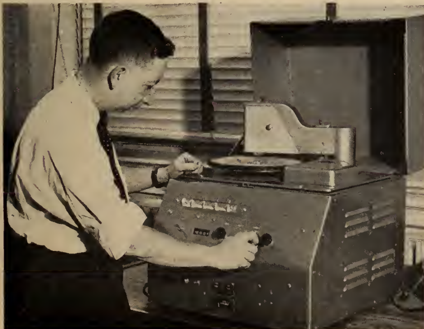
Fig. 4. The Electronic Dirt Counter. Paper sample rotates on turntable, is scanned photoelectrically, and dirt specks are counted electronically.
