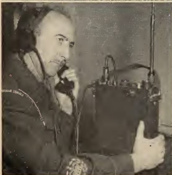
Another new Army means of communication is the field radio set AN/PRC-510, a portable, continuously tunable FM unit with a working range of about five miles in the 58.0-54.9 Mc. frequency range. The set is immersion-proof and is designed to withstand dropping by parachute.
