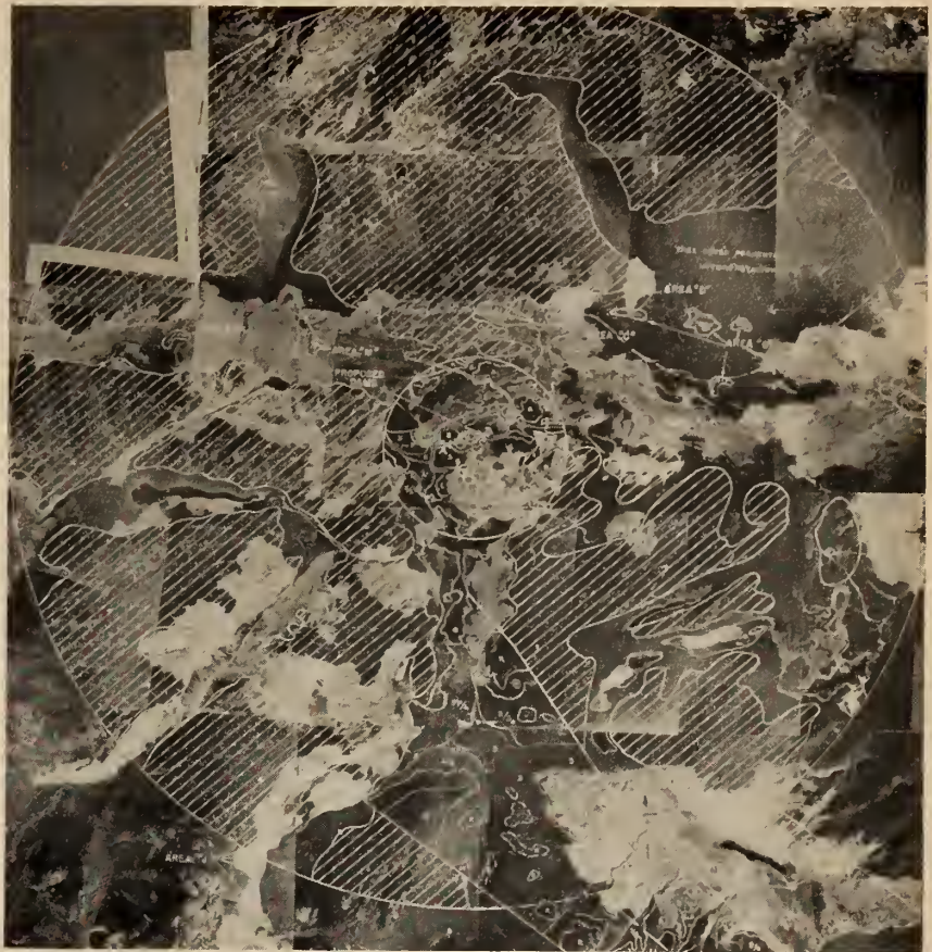
Fig. 3. Photographic interpretation of conditions around a proposed dam site. The large circle defines the area in which the sources of construction materials are desired. Bedrock, gravel, impermeable fill, and other materials have been indicated. The small circle and corridor are areas where overburden depths have been mapped.
