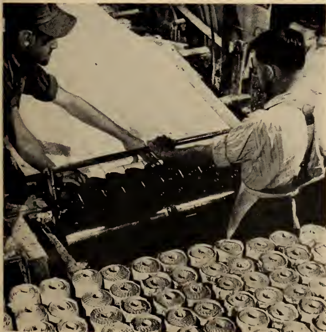
Winding pipe-covering sections made of corrugated and flat asbestos papers. (Photo: Canadian Johns-Manville Limited.)
