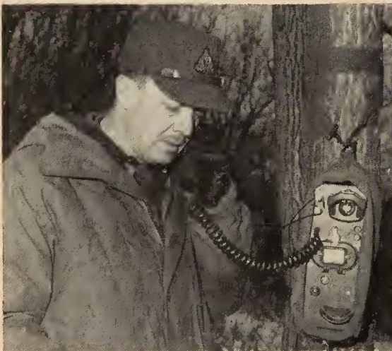
The Army's new field telephone set TA-43/PT was designed for efficient operation under rigorous conditions. It weighs 9½ lb. and range of operation is 14 miles under wet conditions, 22 miles in dry conditions.
