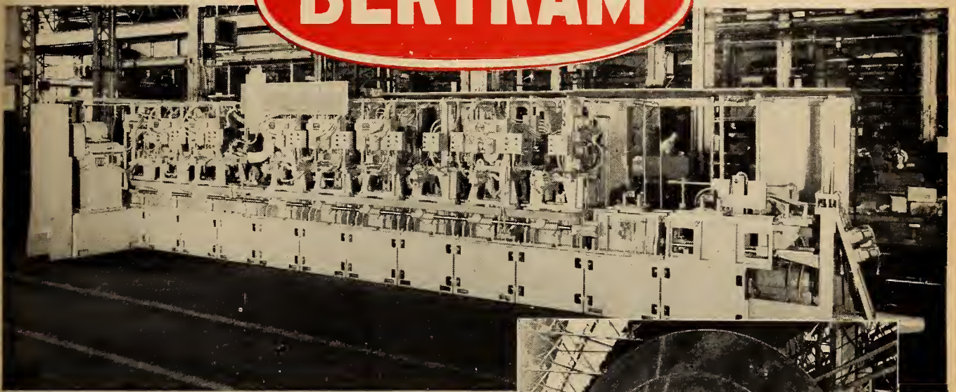
15 station automatic transfer machine
