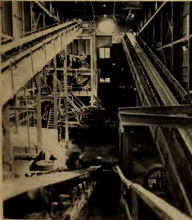
The Flin Flon mine, in Manitoba, is the second largest Canadian producer of zinc. The general view of the crushing plant (left) shows the main belt conveyors; ball mills and classifiers for secondary grinding are seen (right) in the concentrator plant. (Photo: Hudson Bay Mining and Smelting Co. Ltd.)
