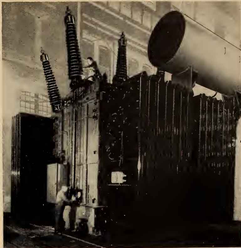
Heavy electrical equipment for the power industry is exemplified by this 300-ton autotransformer built for Hydro-Quebec's Bersimis development.
