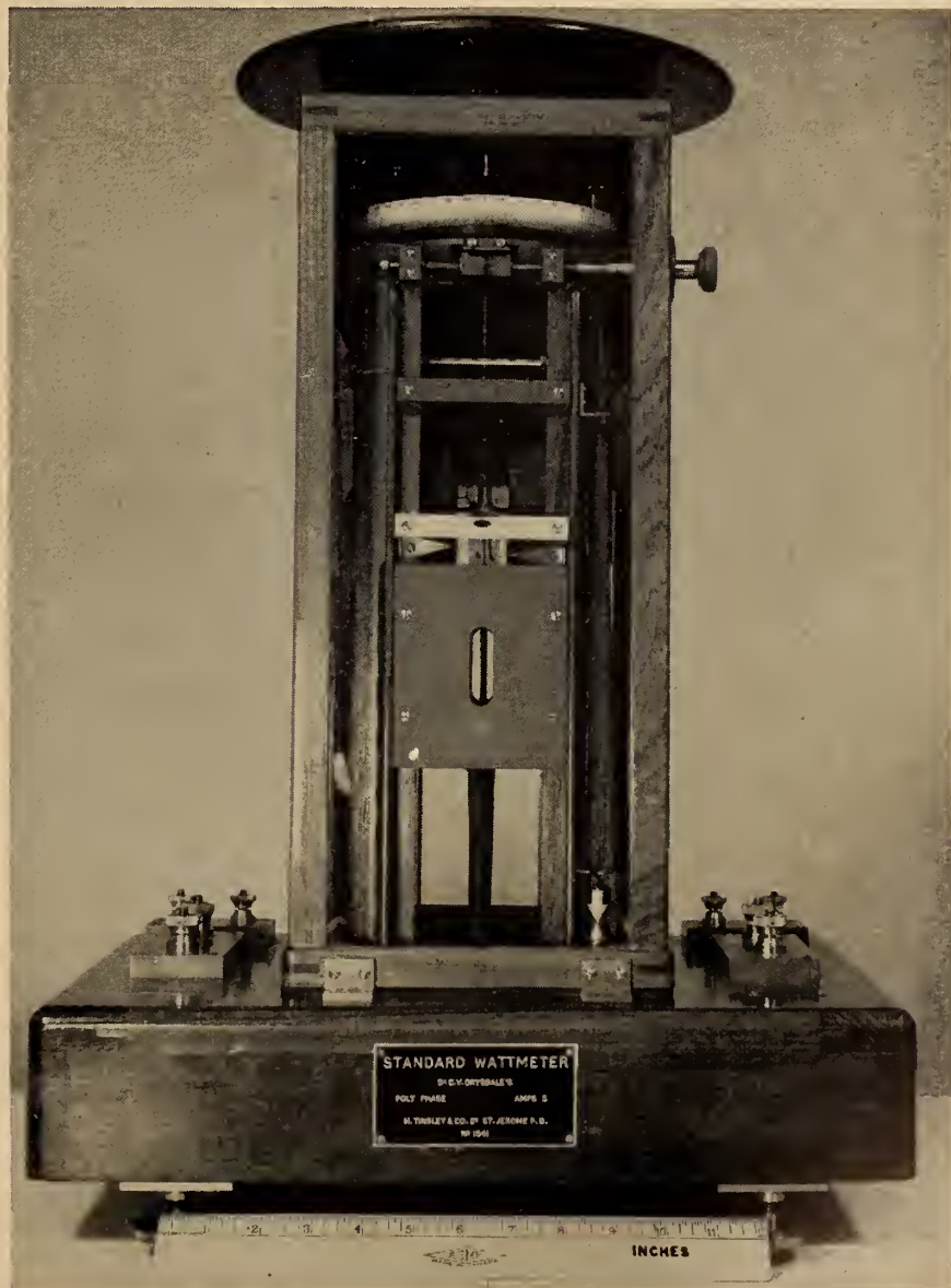
Figure 2. The Drysdale dynamometer wattmeter. Two pairs of fixed coils are perpendicular to each other and the moving coils are suspended from a torsion head by a spiral phosphor bronze spring. The moving coils are individually wound astatically, and as a result each pair of fixed coils has to be connected with the fields of the two individual coils opposing each other. The moving coil therefore moves in a far from uniform field. Construction is almost completely of wood and bakelite.
