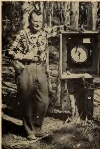
Fig. 5. Typical mercury-bulb recording thermometers, Uranium City, Sask.
