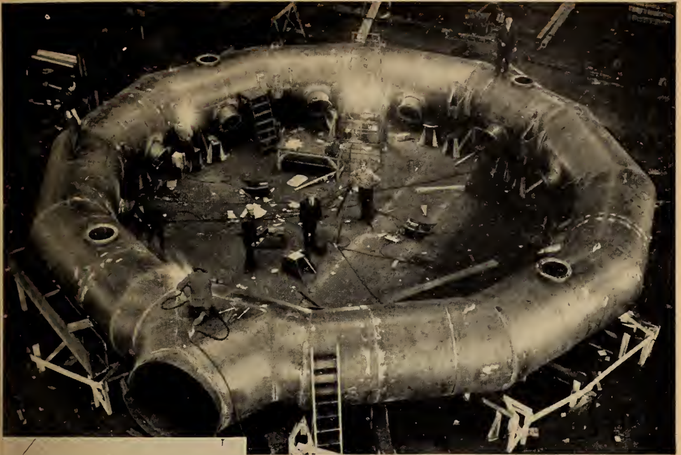
This blast furnace bustle pipe is one of a number of components built by MLW for the Dominion Foundries and Steel Company's recently completed No. 2 blast furnace at Hamilton, Ontario.
