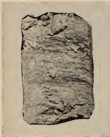
Fig. 4. Section of borehole sample of varved silty sand.
