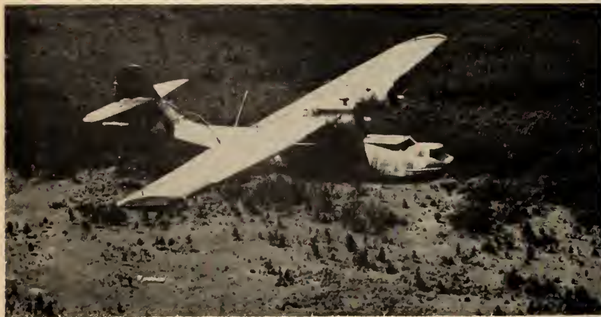
Fig. 9. A Canso amphibian provides the platform for three simultaneous geophysical methods: total field magnetic, dual-frequency electromagnetic, and radioactivity. In addition, a 35-mm. positioning camera and a radar-operated height-measuring device are in operation. All results are recorded continuously and automatically.
