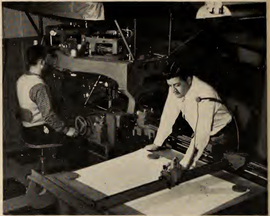
Fig. 1. A stereometric plotting machine, used for the accurate and rapid production of contoured topographic maps.
