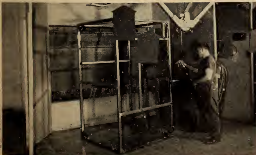
Fig. 7 (top). General view of paint mixing room. Vacuum still for thinner reclamation can be seen in background.
