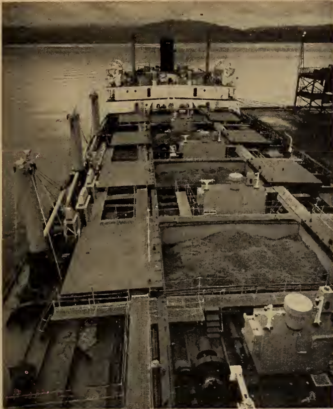
An unusual application of water transport inaugurated in 1956 was the bulk transport of kraft pulp, in "noodle" form, in the specially-constructed tanker S.S. Duncan Bay from the Campbell River mill of Crown Zellerbach Canada Limited to the converting plant in California. (Photo: Jack Cash.)
