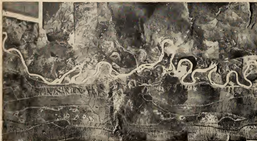
Fig. 2. A segment of a highway route location, plotted on a photographic mosaic. The photo-interpreted features include detailed drainage, waterlogged areas, soil types, sand, gravel, bedrock, and the route itself.
