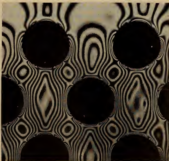
Fig. 17 (top, right). Enlargement of in-line arrangements from plate carrying vertical compression load.
