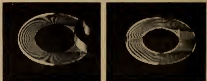
Fig. 15. (a) Left, scattered light fringe pattern for transverse plane through unperforated tube. (b) Pattern for transverse section tangent to one side of perforations in tube.
