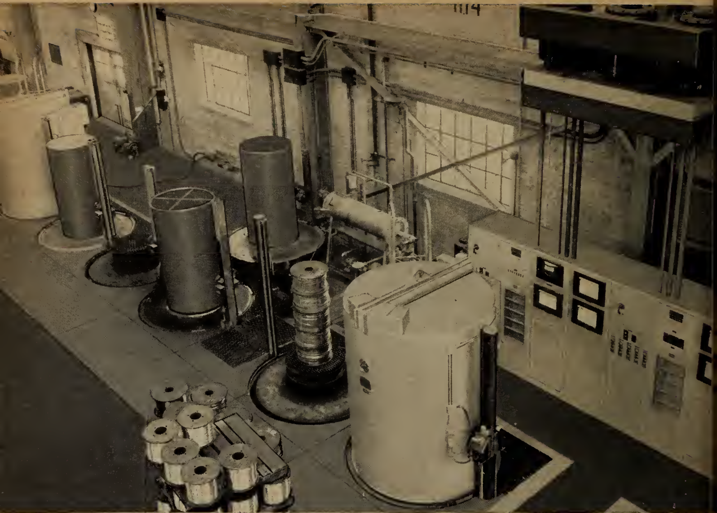
Two G-E Bell Furnaces for annealing copper wire in reel and coil form are employed in wire manufacturing, Peterborough Works, Canadian General Electric.
