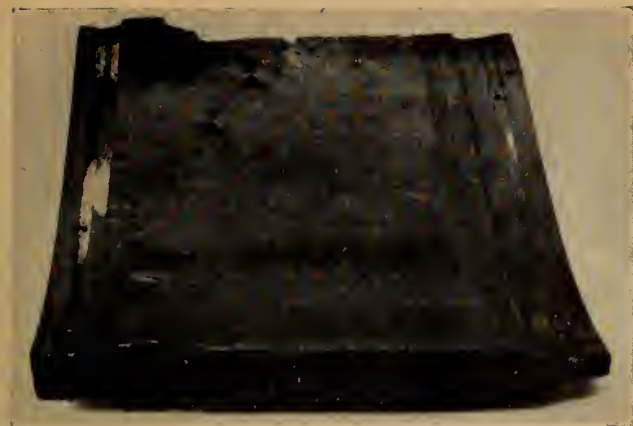
Fig. 31. Close-up, showing brittle nature of fracture.
