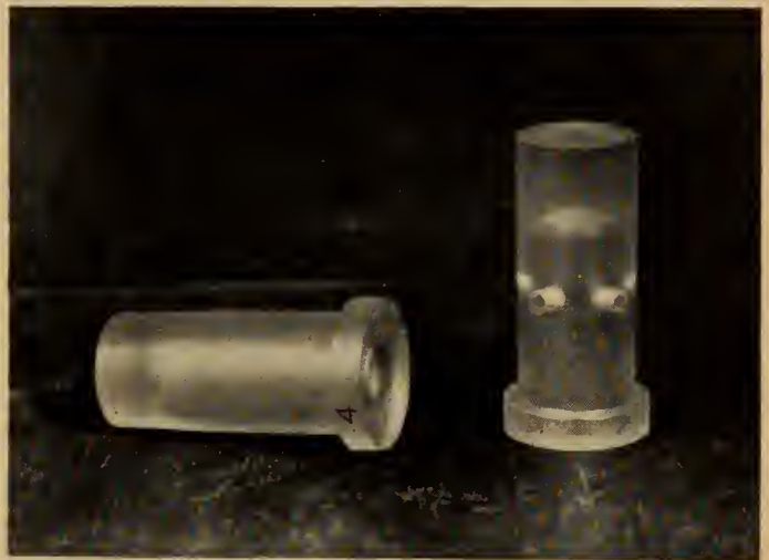
Fig. 12 (below). Two Fosterite models used in an analysis of stresses in thick-walled tubes.
