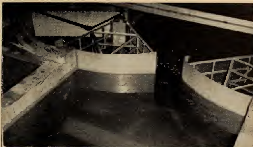
Fig. 10. Upstream view of the sector gate model in operation.
