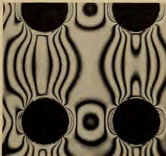
Fig. 16 (left). Plate carrying a vertical compression load.
