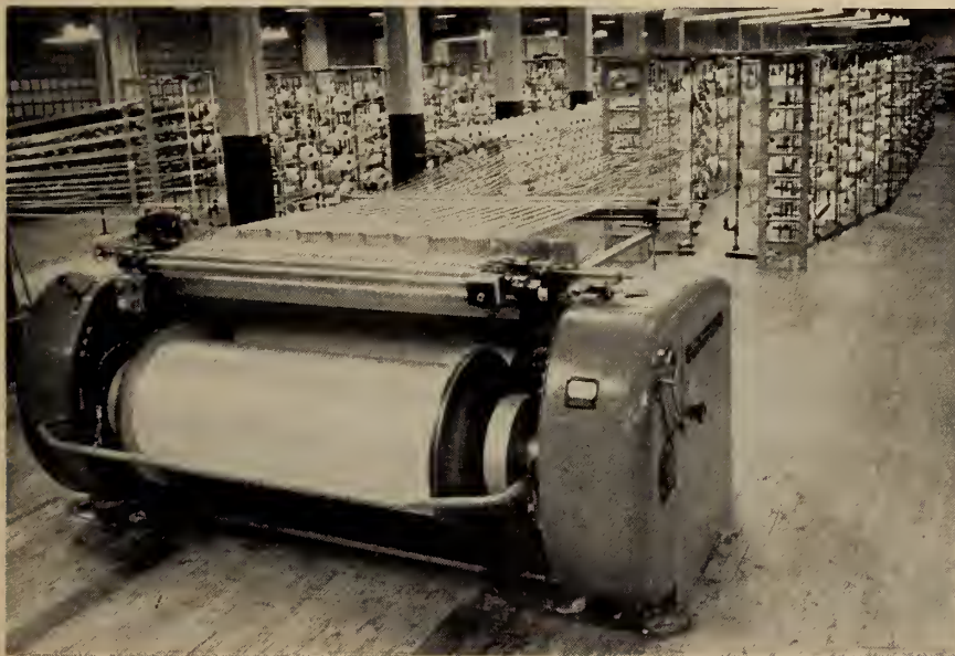
Fig. 14. High speed tire yarn beamer, with creel. Partially-filled beam, foreground, is fed from cones of yarn on the creel, right background.
