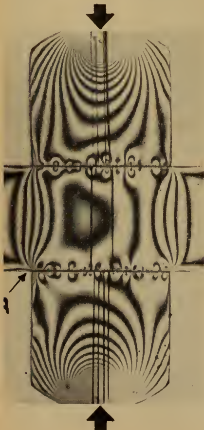
Fig. 19. Tension stress existing adjacent to large compressing contact stress.
