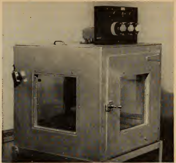
Fig. 8. Oven suitable for stress freezing. Constant temperature control is incorporated.
