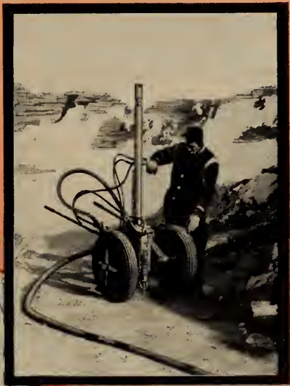
JOY FW-4-P FEATHERWEIGHT WAGON DRILL For shallow cuts and clean-up drilling
