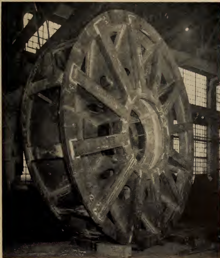
Fig. 11. Fabricated head cover for Niagara pump-turbines.
