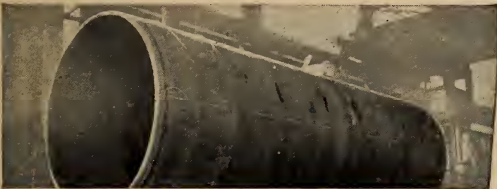
• 1 3/4" tank shell for a high pressure steam drum for an oil refinery.
