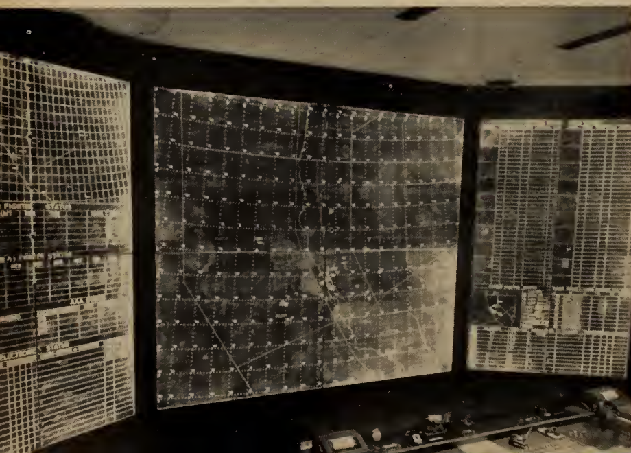
Hamilton Air Force Base, Calif. The new vertical plotting board recently installed in the 28th Air Division Air Defence Control Centre serves to plot the positions of all aircraft flying within the Division's operational area.
