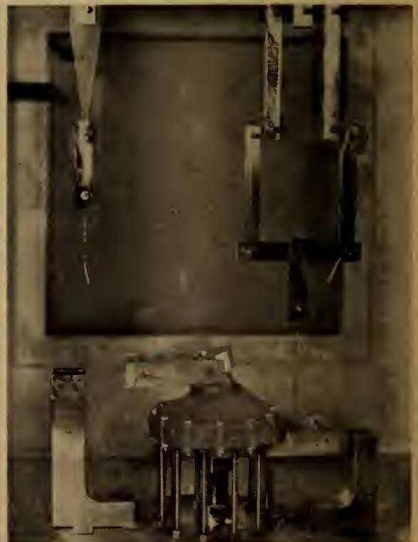
Fig. 10. Fosterite model (hub and flange joined by a conical web section) in the oven after stress freezing.
