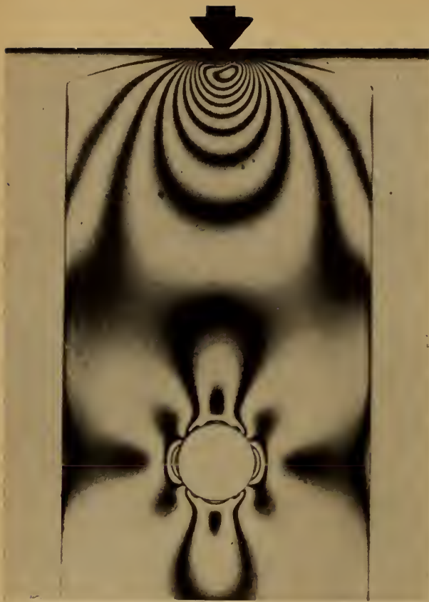
Fig. 1. Fringe pattern for short column, loaded in compression, with transverse hole
