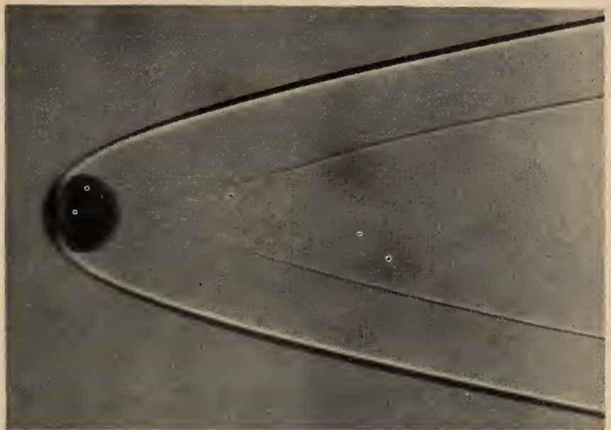
Picture of 10,000 miles per hour. The sphere was shot from a new high velocity Light-Gas Gun developed at NACA Ames Aeronautical Laboratory. Shadowgraph picture, made at one ten millionth of a second, shows the strong shock waves formed by the speeding model.
