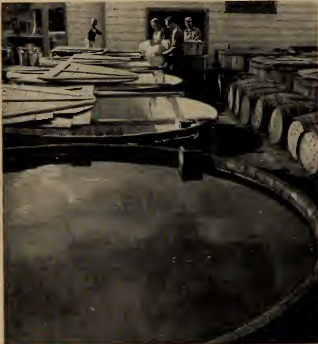
Pictured above is a bottery of Pacpipe Brine Tanks at McLarens Ltd., Vancouver, B.C., for processing and storing pickles.
