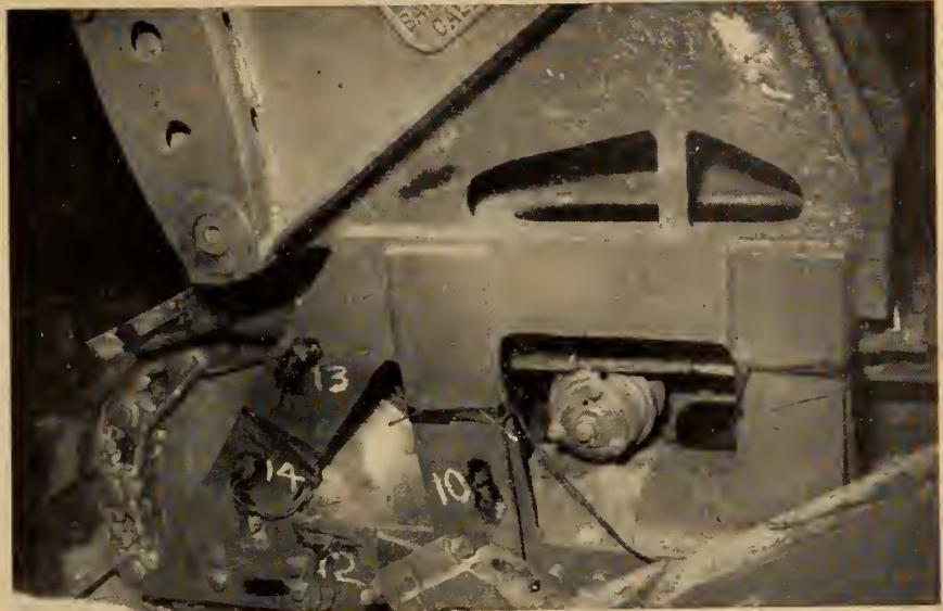
Fig. 3. Typical attachments of strain gauges to components.
