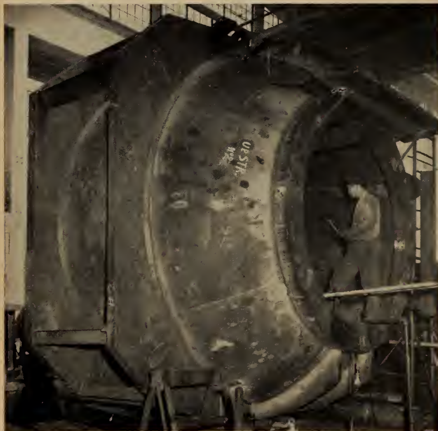
Fig. 12. Fabricated straight-flow valve body.
