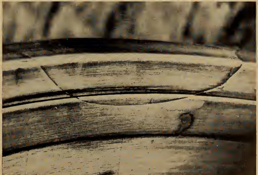
Fig. 37. Cracking over pole at change of section.
