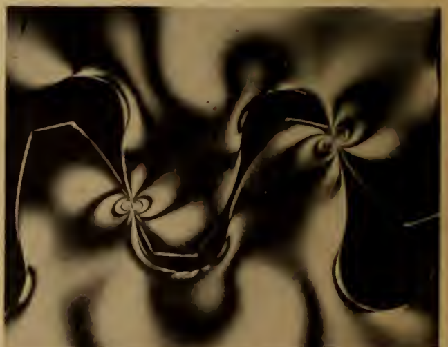
Fig. 3. Fringe pattern for spur gear teeth: two pairs of teeth in contact.
