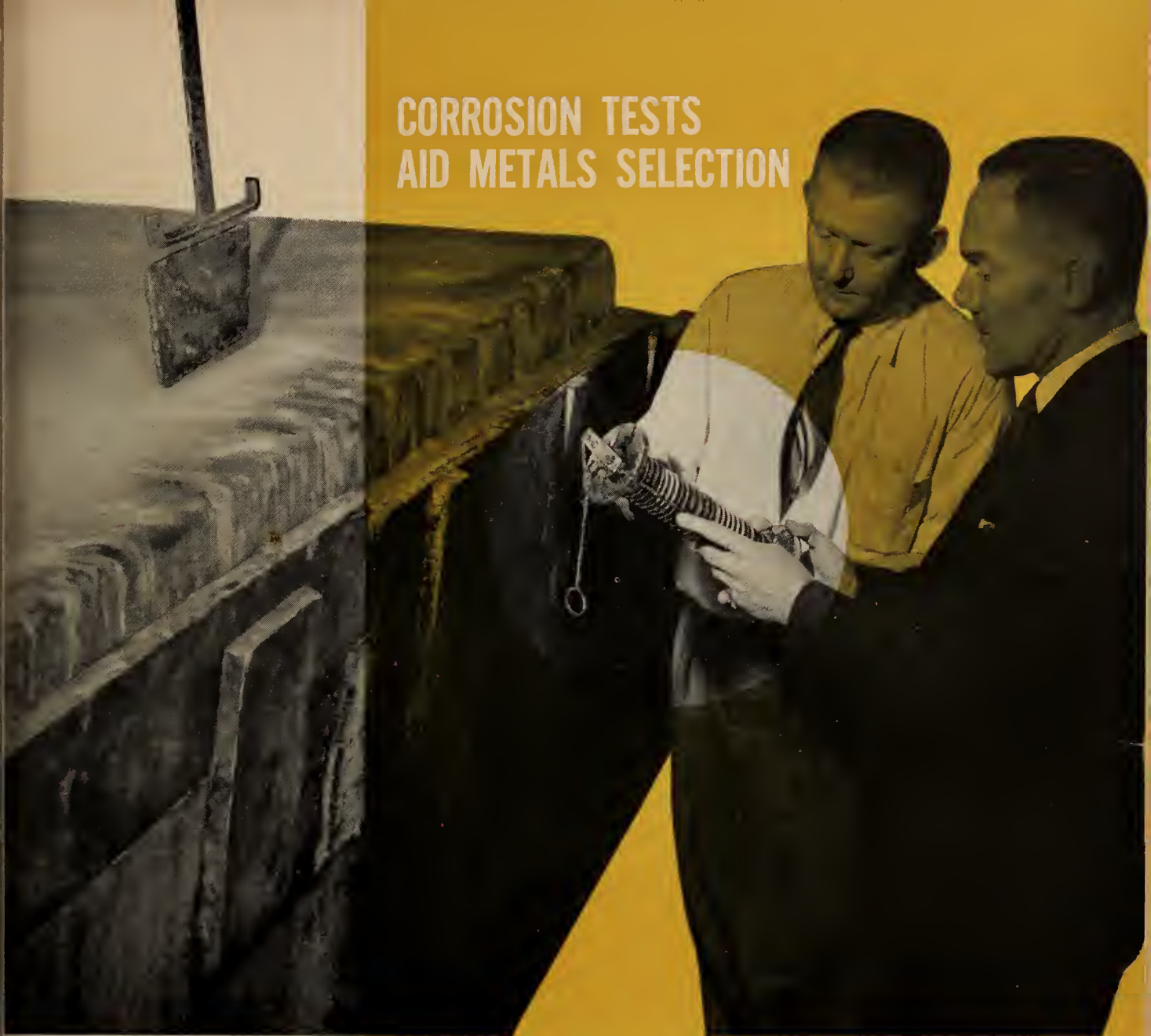
Corrosion test spool is examined by plant supervisor and INCO Research Engineer at Ontario Paper Company, Thorold, Ontario.
