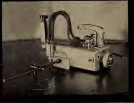
The L.A. Handicutter making a circular cut.
