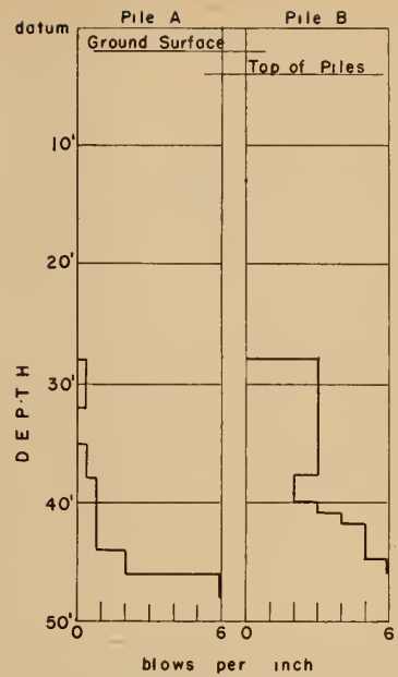
Fig. 3. Driving resistance record of piles A and B.
