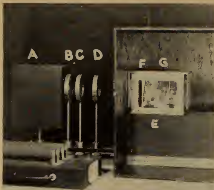
Fig. 14. Model in scattered light polariscope. A, mercury vapour lamp; B, filter; C, collimator; D, polarizer; E, plate glass tank; F, metal slit; G, model in special holder.
