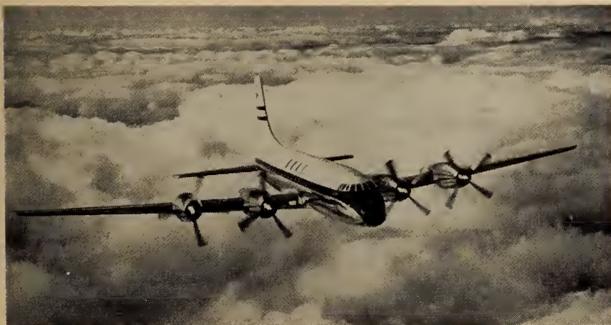
The Bristol Britannia turboprop airliner is scheduled for London—New York service in 1957. It will carry 132 passengers at 400 m.p.h. Range is some 6,000 miles.
