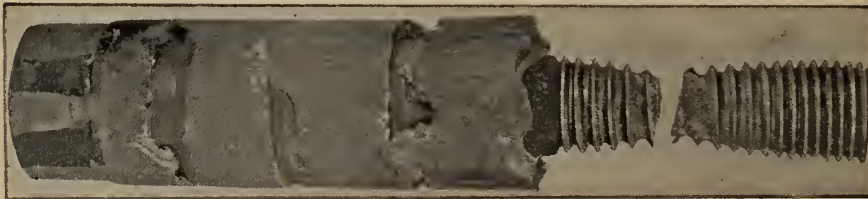
Two-inch steel bolt anchored in concrete with "CINCH" Expansion Anchors— Bolt broke at seventy tons — Anchor did not pull out.
