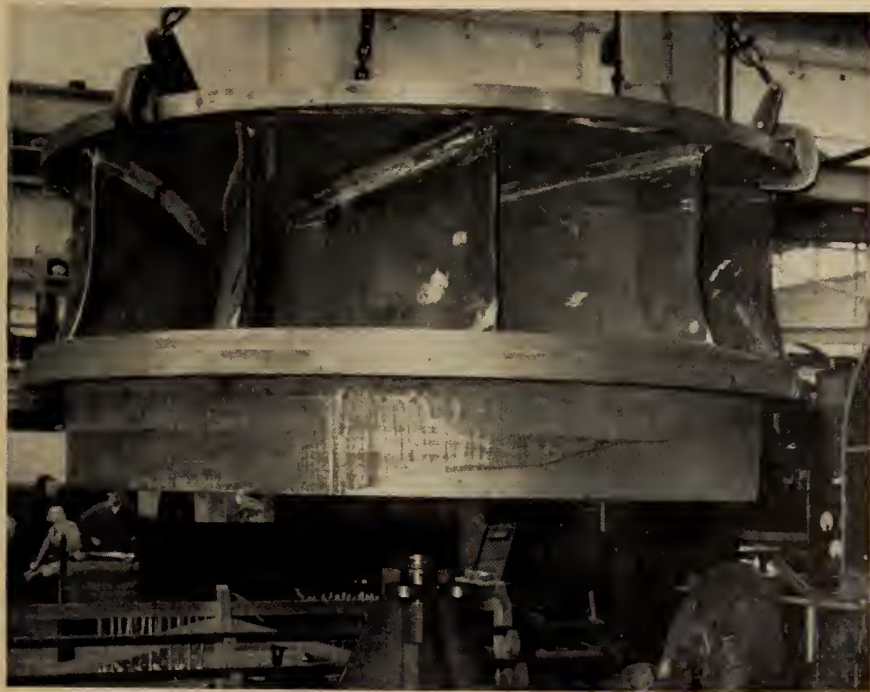
Fig. 3. Fabricated runner for 74,000 b.h.p. medium head Francis unit.
