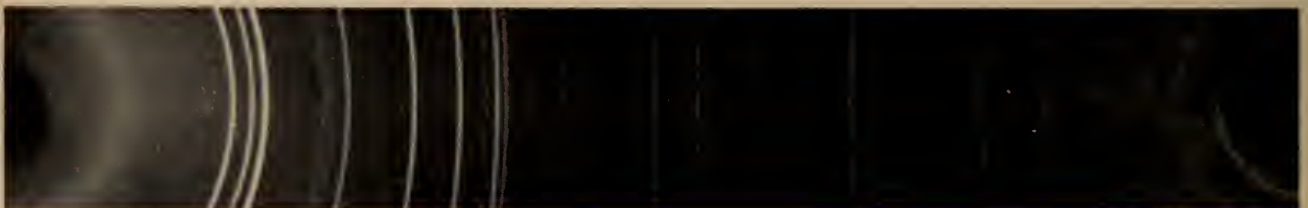
Fig. 2. X-ray diffraction pattern of ZnO.
