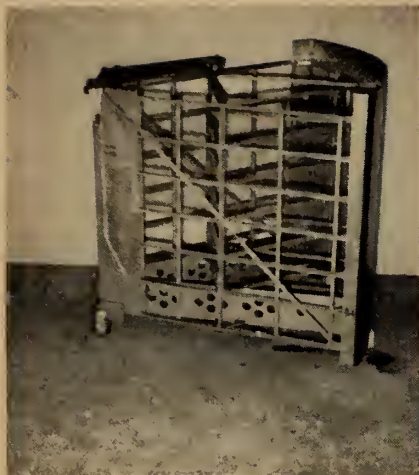
Fig. 8. Model of one leaf of a sector gate, showing framing details.
