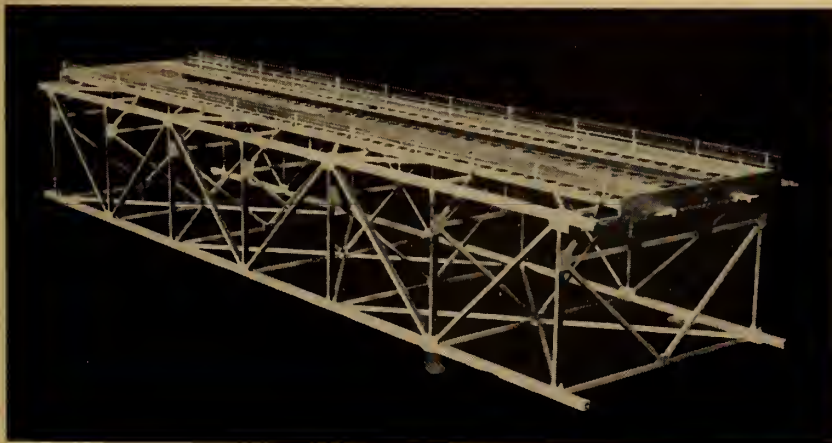
Fig. 5. Dynamic model used in the wind-tunnel tests at the University of Washington. Accurately built to 1/50 scale, the model represents a 253-foot section of the Mackinac Bridge.
