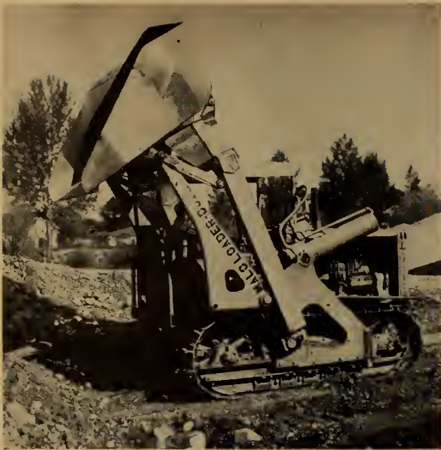
Fig. 1. First model of the overhead loader-dozer, built in 1947.
