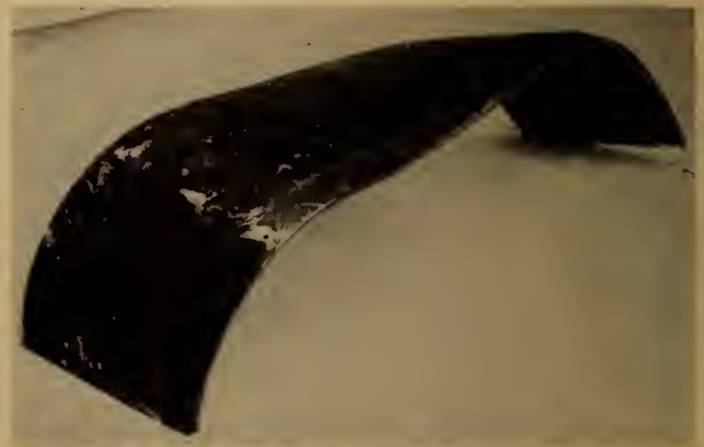
Fig. 30. Larger piece of end bell showing primary fracture.
