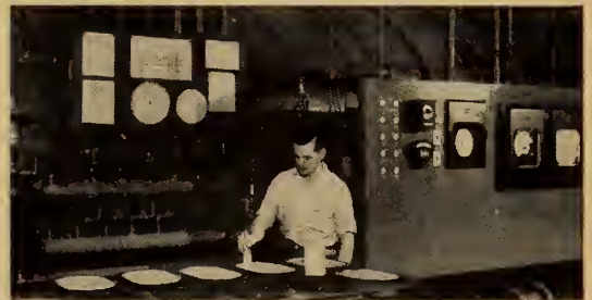
Product reliability has always been stressed at the Dominion Rubber Company. Bristol instruments do their part by precisely controlling and adjusting temperatures and pressures according to a pre-determined time schedule. To the left are Bristol diaphragm-operated control valves.
