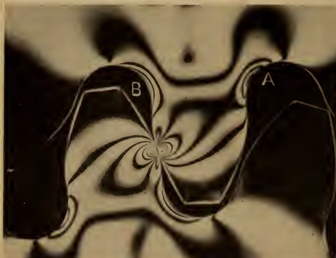
Fig. 2. Fringe pattern for spur gear teeth: one pair of teeth in contact.
